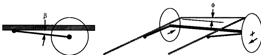
Fig. 6.16 Roll steer with a solid axle.
