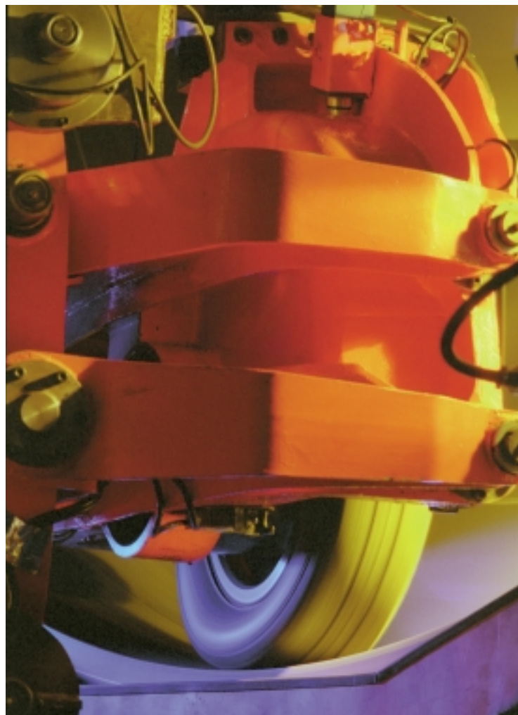
Road simulator in operation. Here, the tyre is running on the inside of the drum.
