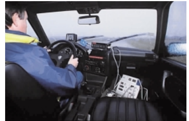
Test driver at the wheel of a vehicle equipped with instrumentation during a transversal grip test
