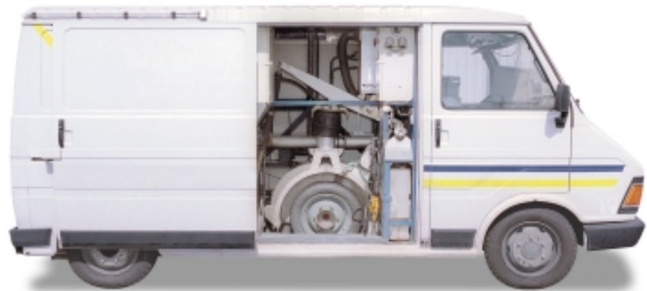
Measurement wheel connected to instrumentation
