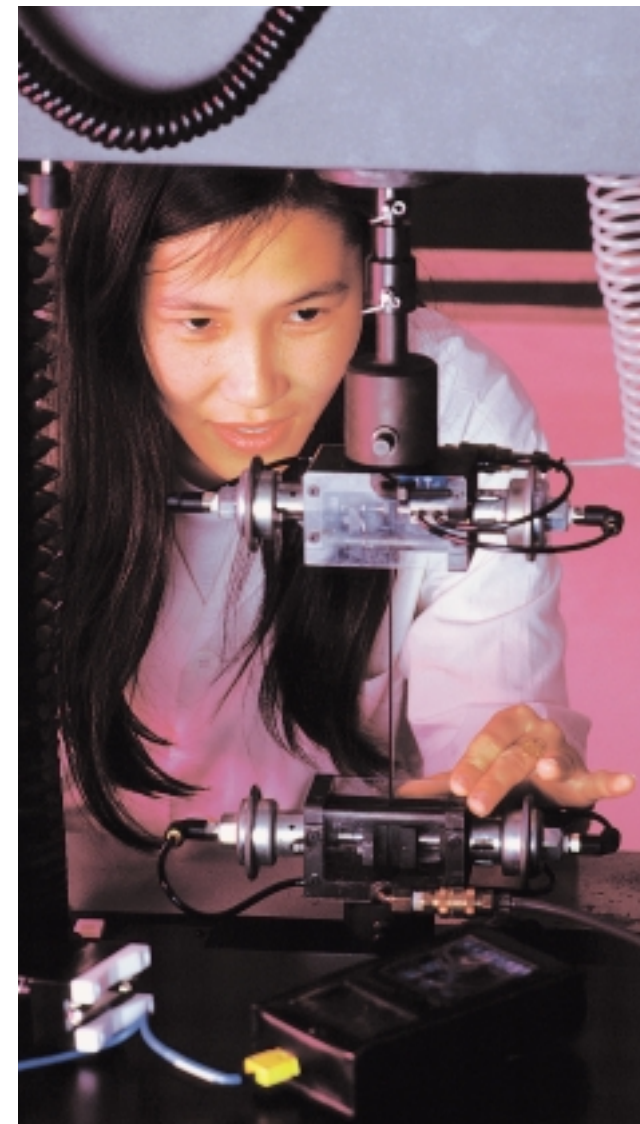
Measuring the rigidity of a material using a traction machine.
