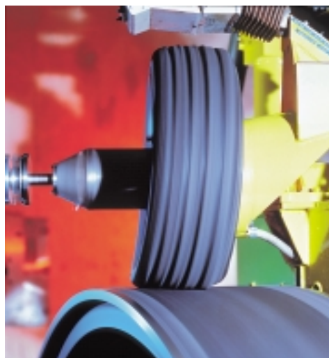
Road simulator in operation. Here, the tyre is running on the outside of the drum.
