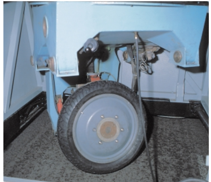
Measurement wheel connected to instrumentation
