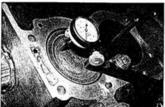
Dial gauge clamped to an alloy block.
