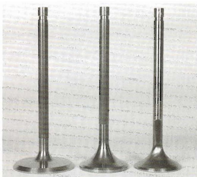
Left to right is a 2.050-inch-diameter titanium intake valve from Buick (25500039); a 1.60-inch production exhaust valve; and an inconel exhaust valve with a diameter of 1.60 inches. Buick part number is 25500025. The inconel exhaust valve is designed specifically for turbocharged applications.
