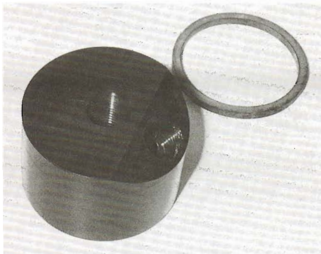
Aftermarket adapters such as this one can be used to facilitate plumbing to remote filters or coolers. The adapter threads onto the oil pump housing.
