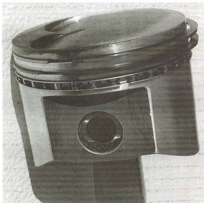
Installing double Tru-Arcs is one acceptable way of retaining full-floating wristpins. Rounded sides go together so the sharp edges dig into the aluminum of the piston to further effect the containment.
