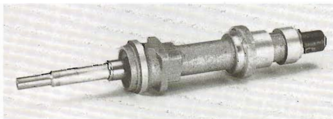
You can devise an oil pump priming tool from a worn-out Buick distributor housing and shaft. Some lathe work is necessary if the shaft is to accept a 1/8-inch drill motor.
