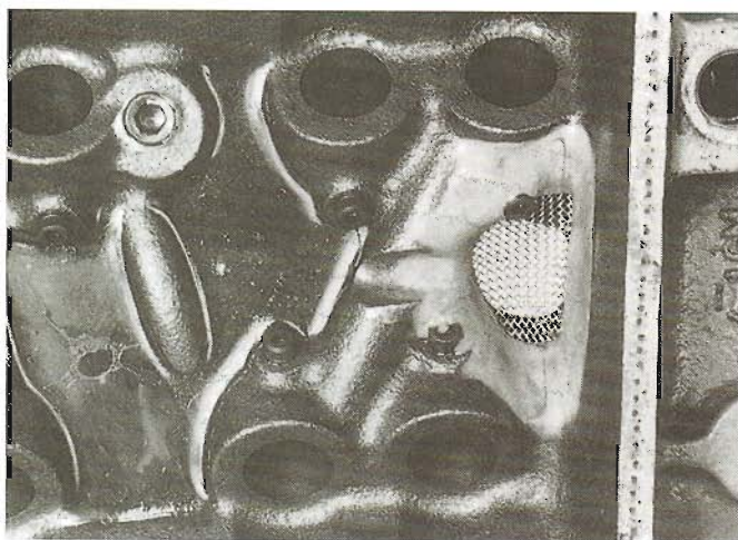
On this Stage II block, oil drainback screens have been epoxied in place at each end of the lifter valley to keep debris from reaching the oil pump. Do not use very fine screen here because it restricts oil drainback. A transparent epoxy has also been poured in the valley between the lifter bores to promote oil flow through the screen.
