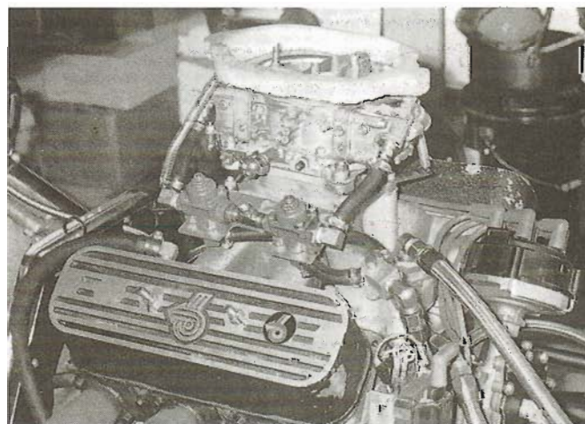
The Stage II manifold (25500029) in action on a development dyno. This piece has an aluminum 4-barrel design with a square-bore carburetor mounting flange and no heat crossover passage. Note the use of a pressure regulator for each of the float bowls. Foam at the top of the carburetor seals it to a plenum.
