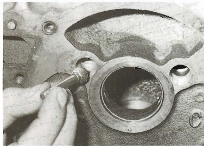
Using a round cutter, radius as best as you can the intersections in the oiling passages. This is time-consuming and tedious but worthwhile.
