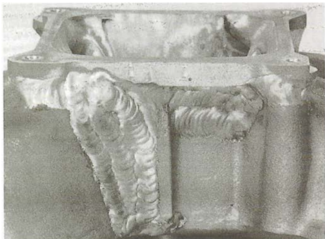
For experimental work, this manifold was welded onto the exterior of the plenum to facilitate additional interior grinding.
