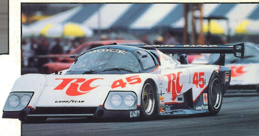
Turbocharged 3.4-liter Buick V6 in IMSA GTP configuration produces over 900 HP at 74-in.Hg boost.
