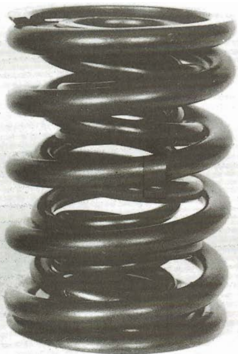
The Stage II valve spring consists of three chrome silicon wires that yield a total spring rate of 500 lbs./in. Valve closed spring height is 2.00 inches with 157 pounds on the seat. Valve open spring height of 1.35 inches yields 471 pounds on the seat. The Buick part number is 25500035.
