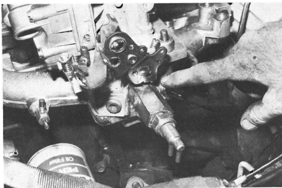
4-16. If you intend using a two barrel Holley on a Pinto with emission equipment, you will need to alter the carb linkage a little in many cases. For instance it is often necessary to cut part of the original linkage at the point indicated so that it clears everything when the throttle is opened.
