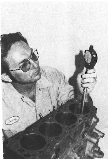
7-15. Here, Denny Wyckoff runs through the final stages of checking out a block for a hot street machine. Not only are the bores accurately sized but they have also been given the correct honing finish, as can be seen. The block has also been decked and a very important step, the tops of the bores have been chamfered to allow easy installation of the piston and ring assembly.
