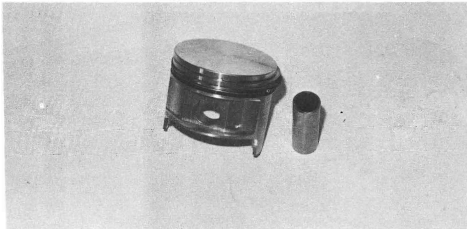
7-18. This design of Aries-made piston was used in some of the author's most powerful normally aspirated engines. Special rings made by Childs & Albert were used to combat ring flutter at 10,000 rpm. The top ring is a very thin section Dikes ring, whereas the second ring is a conventional thin-section ring. The all-up weight of this piston was 508 grams, 65 of those being due to the super-light tool steel Esslinger piston pin. Although at first sight this piston looks heavier than the Holbay item remember that it is \frac{1}{4} " longer due to the lower pin height on it. Although it's slightly heavier, it would be used in conjunction with a rod \frac{1}{4} " shorter and therefore the reciprocating weight of the small end of the rod would be correspondingly less. Couple these two facts together and the piston, plus the reciprocating weight of the rod comes out at about as low as it's possible to get. Had this piston been made with a higher pin, it would have undoubtedly been 30 or 40 grams lighter.
