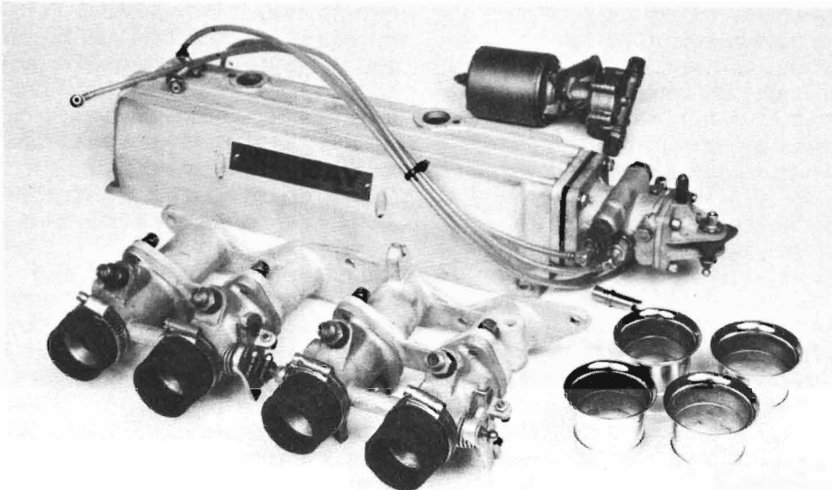
4-34. This fuel injection system is offered by Holbay Engineering. It is intended for use with petrol/gas as opposed to the alcohol systems offered by Esslinger Engineering, Racer Walsh and others.
