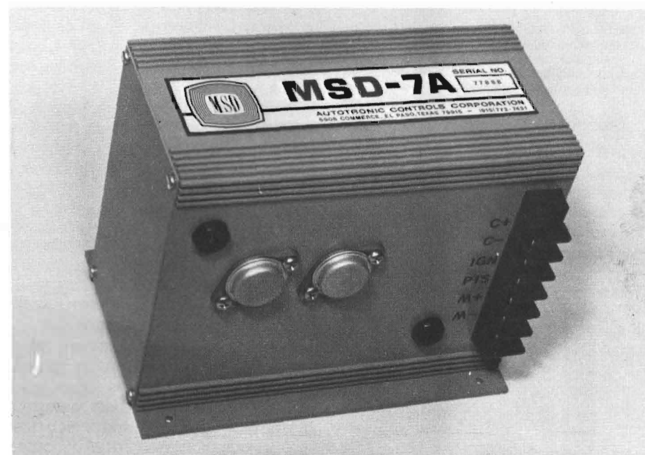
6-6. The best ignition system I could find for Ford's S.O.H.C. engine was the Autotronics M.S.D. The street version seen here performed just as well as the all-out M.S.D.7 race unit. . . .
