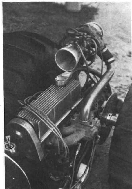
11-14. The distributor used here is a dual diaphragm unit using only the outside diaphragm. This gives 10° - 12° of retard as boost pressure builds up.
