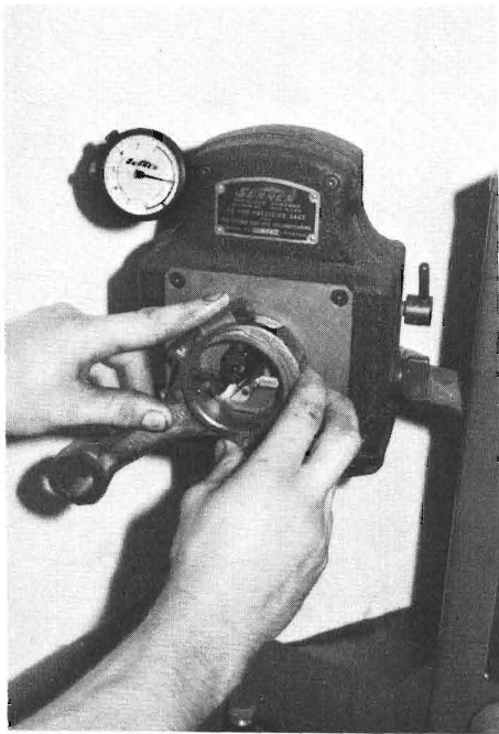
7-30. To avoid spun bearings on high rpm engines, it's necessary to make sure the bearing retention is good. One of the simplest ways of doing this is sizing the rod journal bore (that's the big end) to the minimal size permissible within the tolerance allowed. When I cut the rod as shown here, the bottom limit on the bore diameter was represented by a zero reading on the dial indicator. As you can see, this rod is smack on the bottom limit.
