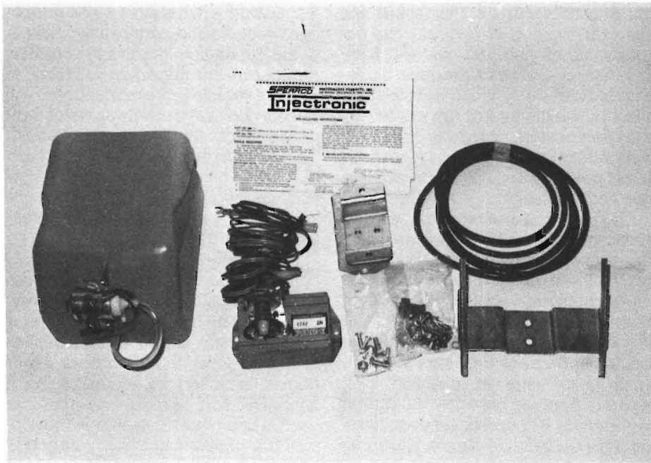
9-1. Here is a Spearco unit of the type I used on almost all my test engines. In three years' testing with numerous units, the only failure I experienced was the splitting of the reservoir tank.
