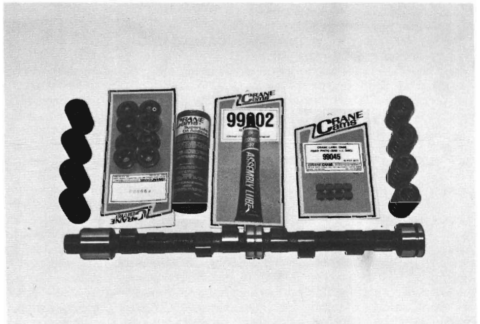
3-22. High lift and long timing are the ingredients for this Crane 333B cam. The components shown are supplied when the entire cam "kit" is ordered. The Crane Super-lube in the bottle, contains the seemingly vital ingredient Zinc Dithiophosphate which is an aid to curing rapid cam and follower wear.
