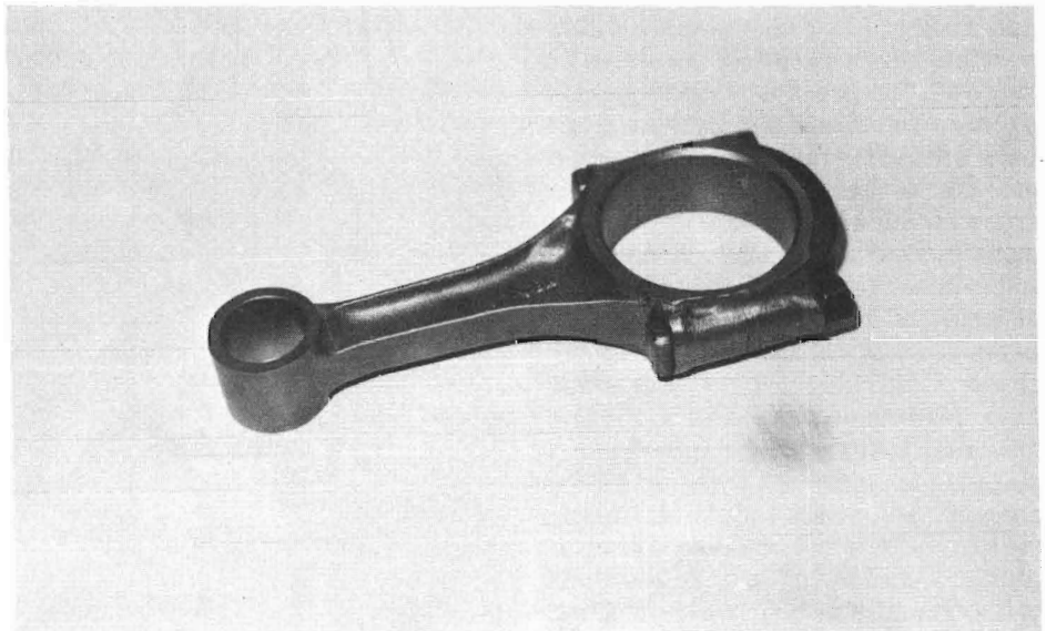
7-26. In this photo you can see just how much the pin end of the connecting rod has been lightened. Compare it with photos of standard rods seen elsewhere in this chapter.
