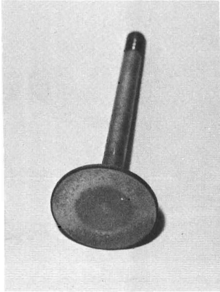
2-32. To stop the ceramic thermal barrier chipping around the edge of this exhaust valve, the valve face was machined, leaving a 0.015" (0.38mm) lip around the edge.
