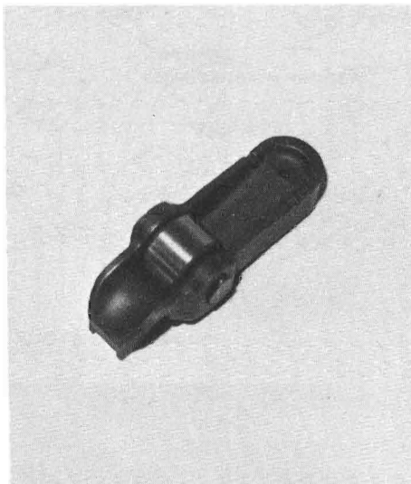
3-12 & 3-13. Manx Racing roller cam follower eliminates the cam and follower wear problem. Some changes in valve train geometry occur but these are easily accommodated as the nearby test explains. Early type shown on left, current type on right.
