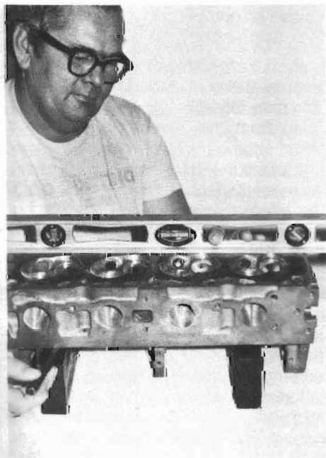
2-35. If you are cc-ing the chambers to determine the C.R., set the head CLOSE to level using a bubble level as demonstrated here by Carl Schattilly of C & G Porting.
