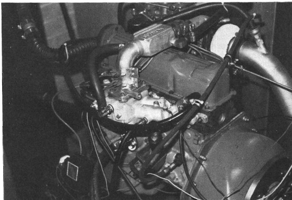
11-3. The cross-over pipe is also an Ak Miller item. When used for road-going applications, heated water from the engine is passed through the jacket of the rectangular section above the cam cover. For race applications, alcohol, super-cooled by dry ice, can be fed through to act as an intercooler.
