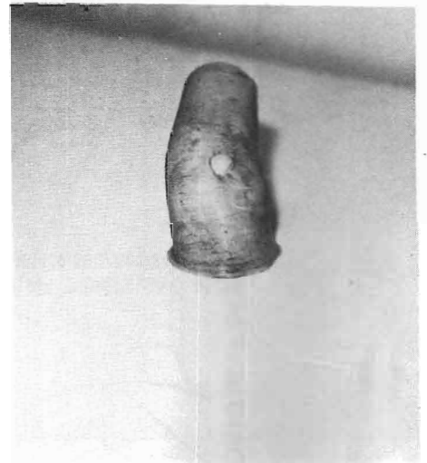
2-18. The centre of the cylinder is on the right of this exhaust port moulding. The flow direction bias shows up as a "lean" to the left.
