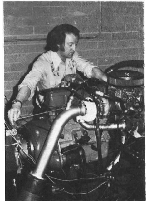
11-1. Here I am making some minor adjustments on the engine before a power run is taken. Note the white exhaust housing on the turbo. This is because it was finished with a coating of Heanium to retain the heat.
