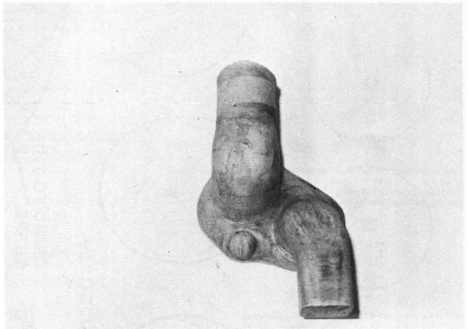
2-13. The widening of the intake port starts about \frac{3}{4} " before the valve guide. Because of the proximity of the chamber wall, the general direction of flow needs to be biased towards the centre of the cylinder. This is partially achieved by taking a little more material from the cylinder wall side of the port than from the other side.
