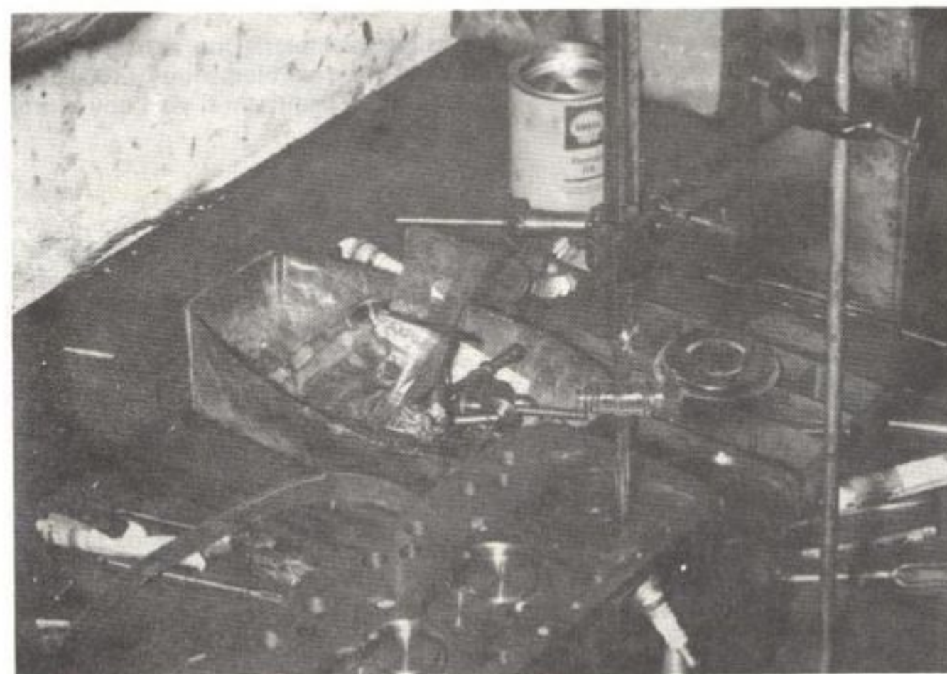
Chamber volume being measured. Note the perspex plate, with hole, covering the chamber. Use grease to seal the edges
