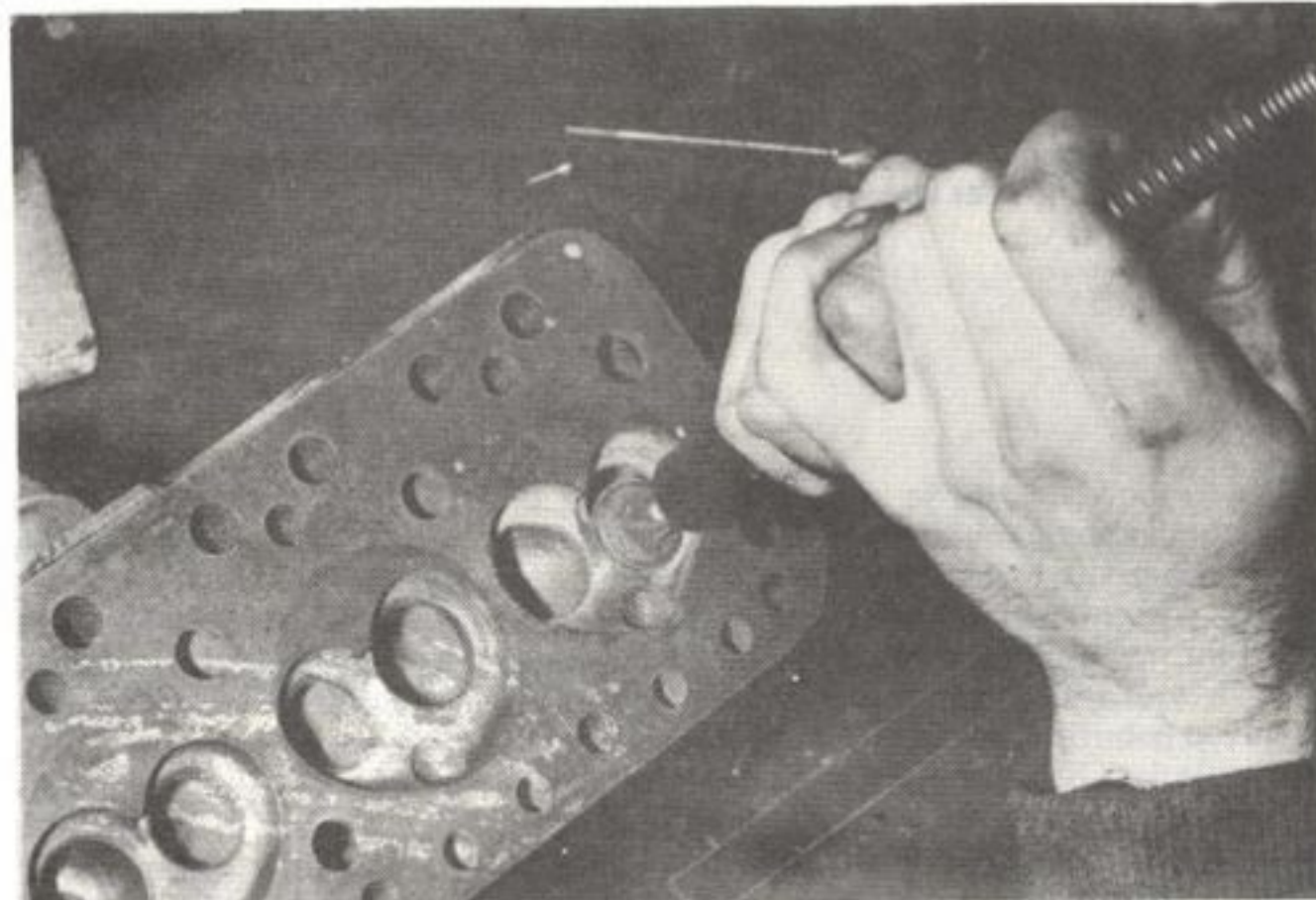
A chamber roof being polished. Care must be taken to avoid damaging the valve seat
