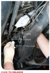
(3) Refill by squeezing lube into filler.
