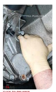
(1a) Check the level of lube in the gearbox or axle by inserting your finger.
