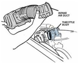
Remove the air duct and inspect it carefully for leaks or tears that might permit uncleaned air into the engine.
