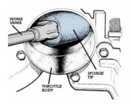
The Intake Snake is one way to safely clean throttle blades and throttle body castings of deposits.
