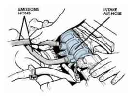
Remove any hoses or wires on the air duct connecting the throttle body to the air cleaner housing. Mark which hose or wire goes where to avoid confusion later
