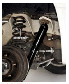
Here's an example of a cone-shaped bump stop (in the spring).
