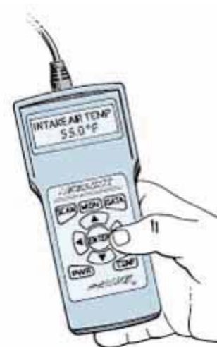
Units with more features will let you snapshot and store data while the car is being driven.
