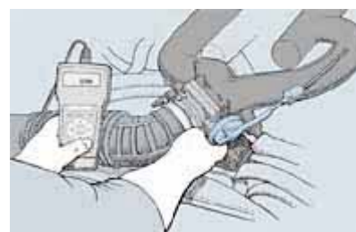
Data-stream scan tools will let you investigate the functioning of most sensors, like the throttle position sensor being checked here.
