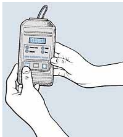
Simple code readers/resetters like this one do not give you sensor data.
