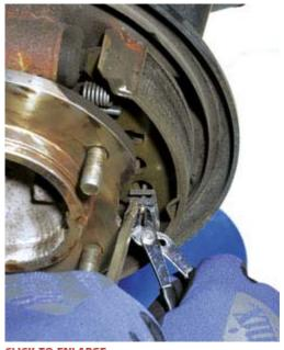
**CLICK TO FNI ARGE Depress the springs** and twist the retaining clips to release the shoes from the backing plate.
