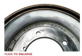
**Brake drums are marked** with their maximum allowable inside diameter and should never be machined beyond the limit.
