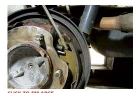
Use an old screwdriver to pop the springs off the shoes to allow the two shoes to separate and come away from the hub.
