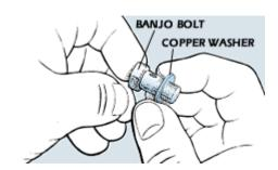
Always replace any copper sealing washers on brake line connections with new ones.
