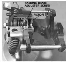
Rear calipers with parking brakes require special techniques to retract the pistons at pad replacement time.
