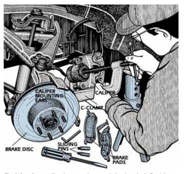
Check for a frozen caliper by attempting to push the piston back. Don't hang the caliper by the hoseuse a piece of wire.
