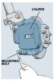
Some makers say that the mounting bolts cannot be reused. Check before removing.
