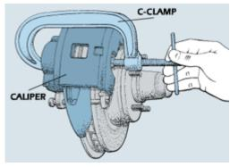
Some types of sliding calipers can be pushed back without removing them from the caliper mounts. Be sure its not seized sliding surfaces that are binding, though.
