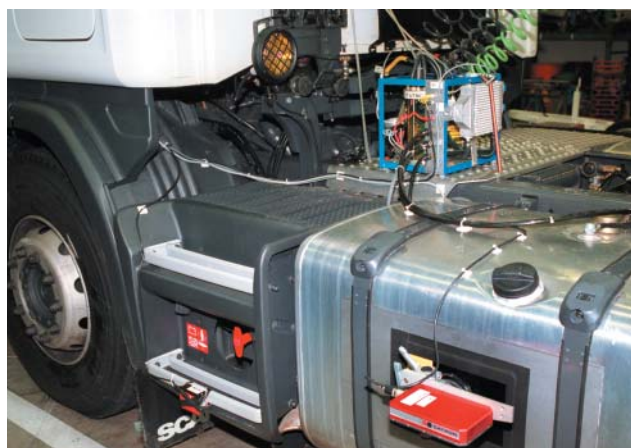
Truck fitted with a flowmeter
