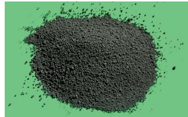
Carbon black is a fine powder obtained by the incomplete combustion of petroleum oils.
