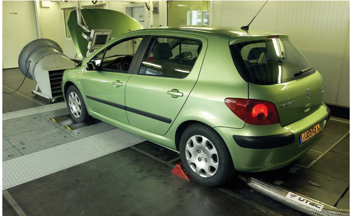
UTAC (Union Technique de l'Automobile, du motocycle et du Cycle) pollution and fuel consumption chassis dynamometer in Montlhéry, France
