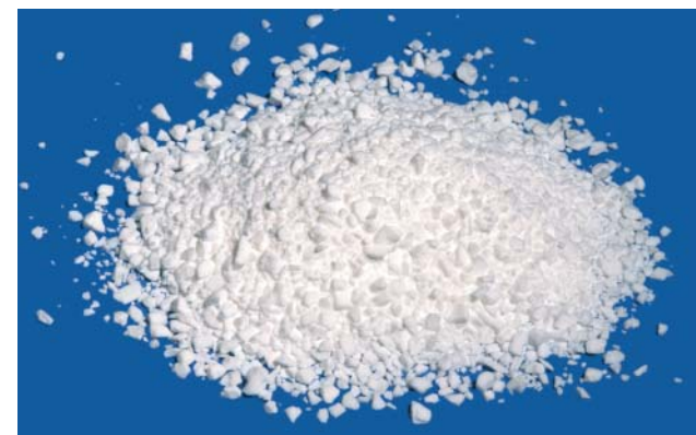
The amorphous silica ( \text{SiO}_2 ) used in tyres is obtained by the fusion of sand and sodium carbonate ( \text{Na}_2\text{CO}_3 ) at a very high temperature. The sodium silicate thus obtained is placed in water, forming an aqueous solution which is then subjected to precipitation using sulphuric acid.
