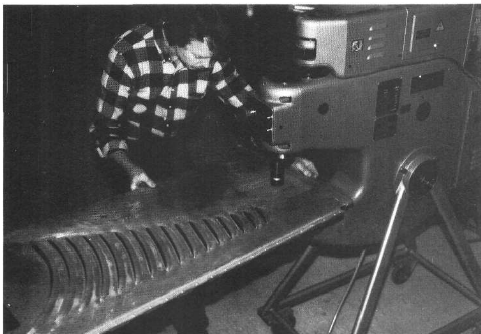
Bill Bizer is using an Eckold Piccolo Kraftformer to repair a Duesenberg hood. The hood had a stretched area several inches in from the edge.
