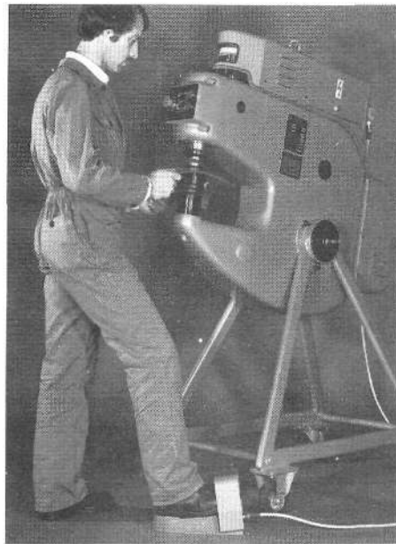
The Eckold piccolo model Kraftformer is one of my favorite tools. There is a variety of special tooling available to suit most any shaping need. Photo Courtesy W. Eckhold A.G.
