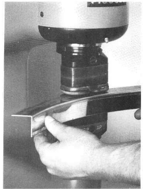
Eckold makes "no mar" dies for their piccolo Kraftformer. One set lets you stretch metal without marring it, another set lets you shrink without marring. Photo courtesy W. Eckhold A.G.
