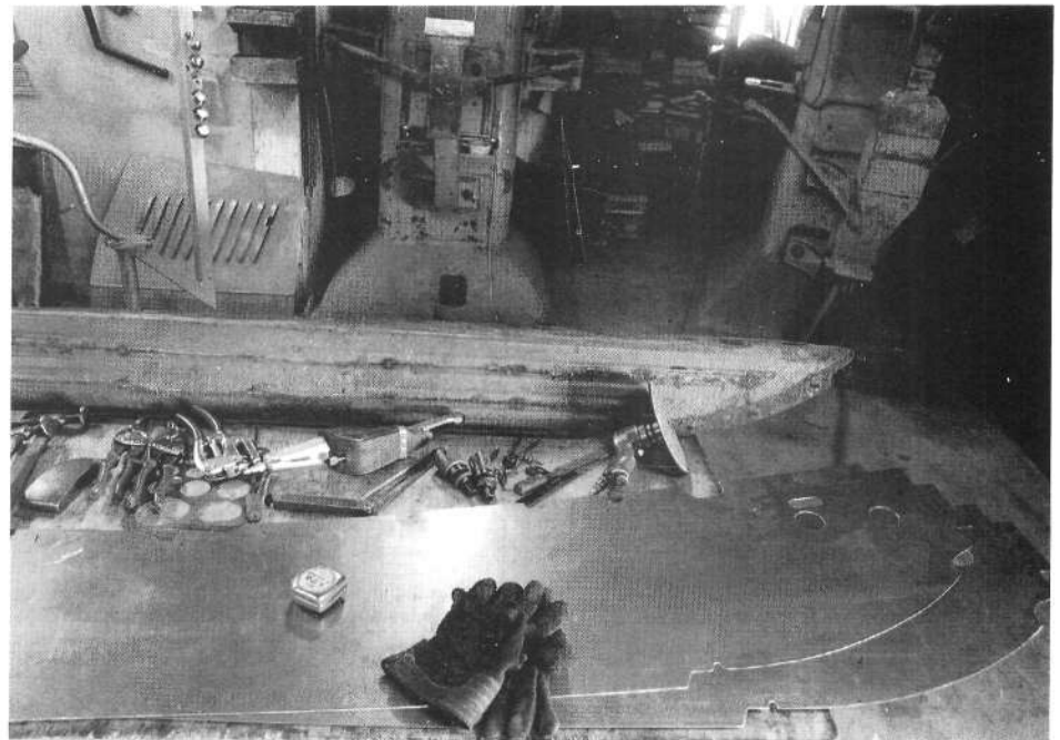
Scott floated the grooved area of the disk over the stretched metal. He used moderate pressure until the area began to grow outward. He kept applying pressure until the area was hot enough to make a wet rag sizzle when it was applied to the area to cool it.
