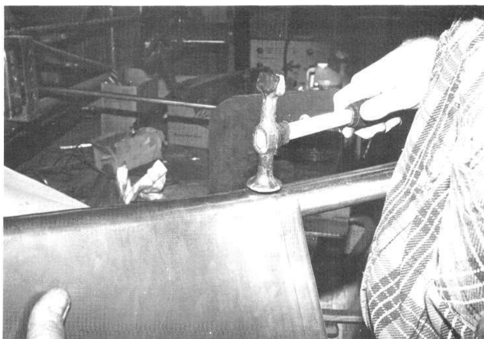
My favorite hammer is the Proto 1427 body hammer, which seems to be in my hand all the time. It's versatile, and has a replaceable fiberglass handle.
