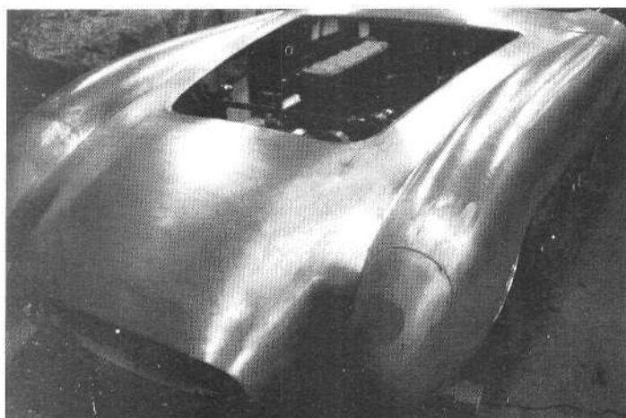
Care, craftsmanship and mastery of power hammer techniques are responsible for these fenders. They are made from individual pieces which have been accurately assembled.
