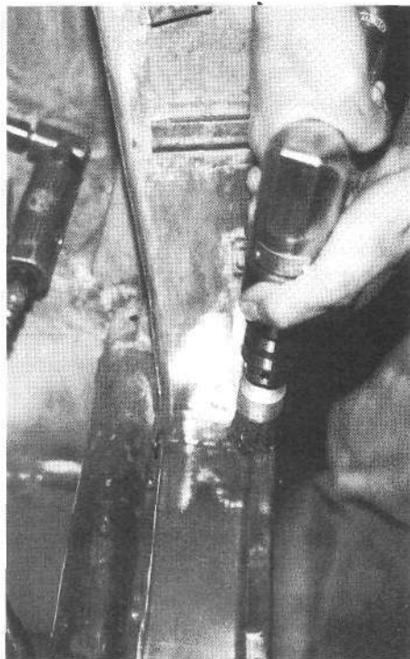
A rotary wire brush mounted in an air drill is just the tool to thoroughly clean steel before lead work.
