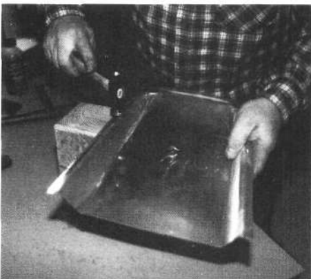
After bending the flange on the beader, I corrected any surface irregularities by tapping with a small hammer over a flat wooden surface.
