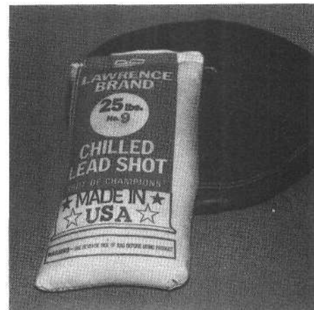
A leather shot bag 12-inch in diameter, 2-inch thick is filled with two 25-lb. bags of #9 birdshot. This shot bag is available through U. S. Industrial Tool and Supply Co.
