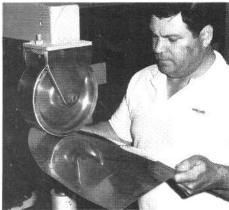
It takes several different wheelings to get a high-crowned curve. Start with light pressure and increase it as you move the metal evenly through the wheel. Photo by Michael Lutfy
