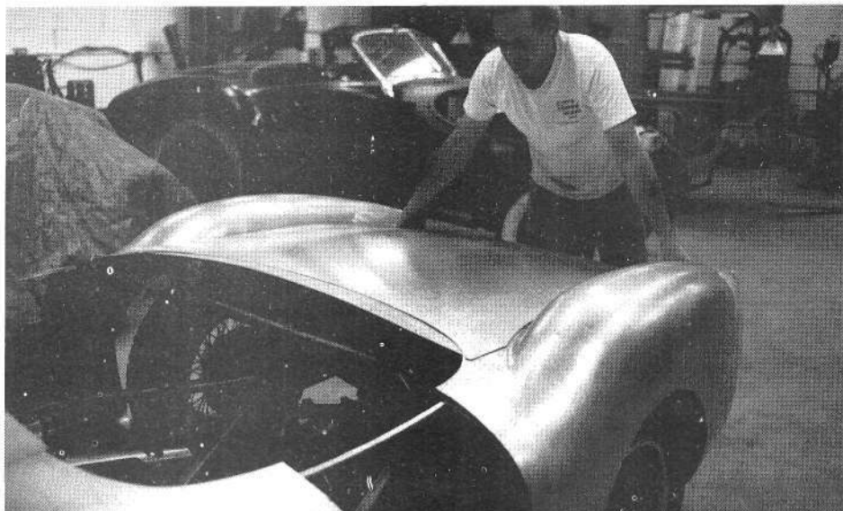
It's best to have the project nearby, because shaping with the power hammer is a gradual process that requires constant checking for a perfect fit.
