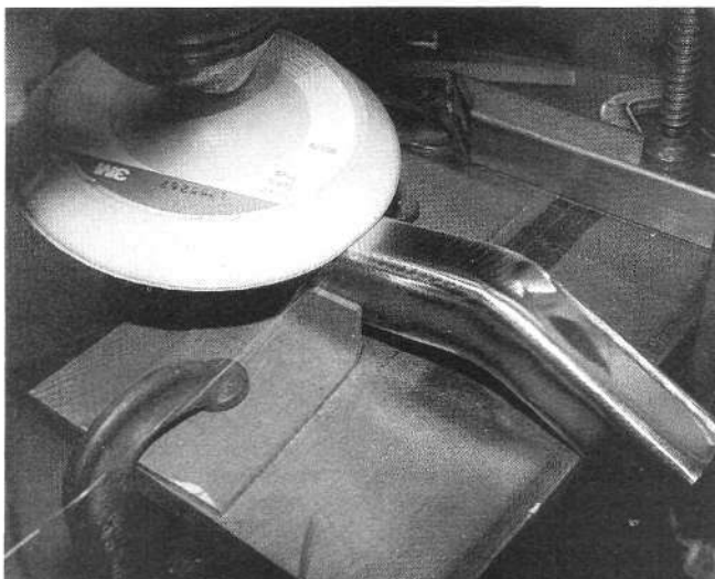
Metal-finish after final welding. Any high spots of the weld are filed off. I used a soft pad sanding disk for the final sanding. This does a nice job and it works fast.
