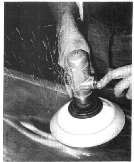
40-grit sandpaper was mounted on a soft pad sander to finish smoothing the metal.
