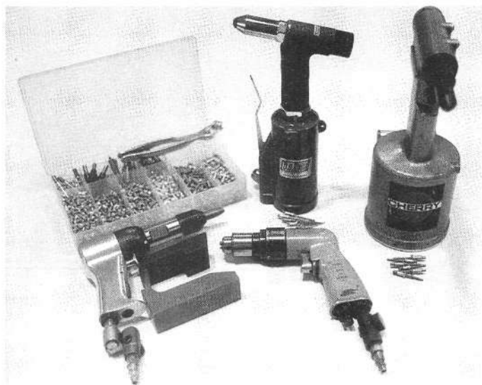
These are some of the tools used in riveting. Each has its own special application. Pneumatic rivet guns need a pressure regulator to maintain the right operating pressure.
