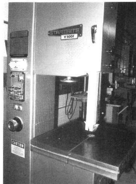
A contour cutting, multi-speed bandsaw is a must. Good ones include a blade welder. A push block saves fingers and helps control the work. Photo by Michael Lutfy
