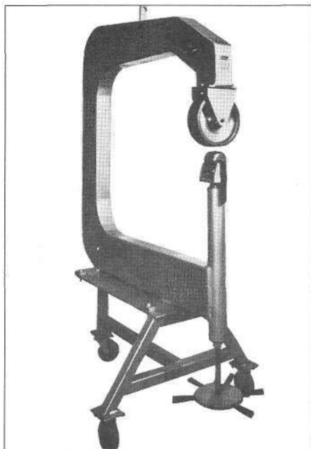
Recently U. S. Industrial Tool and Supply Co. began producing a fabricated steel English wheel in the United States. It's available with a variety of anvils. It's very strong and reasonably priced.
