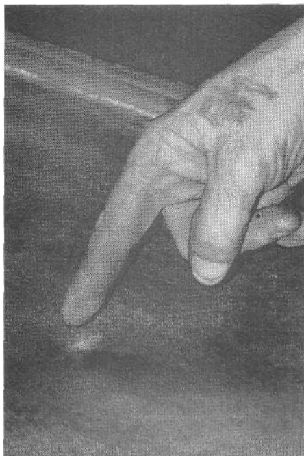
The dent in the rear panel of a '34 Packard was about 1/2-in. in dia. and 1/4-in. deep.
