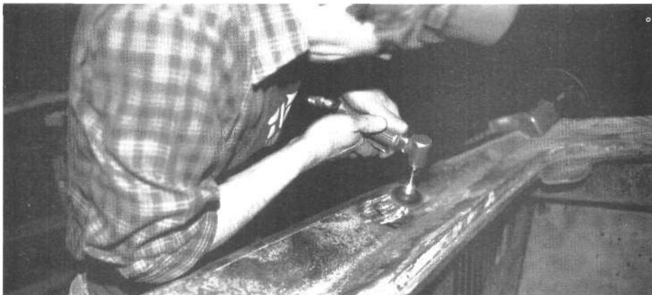
Be careful removing excess weld from a patch. Do not remove any of the metal surface. After initial grinding you may need to use more dollying to raise low areas.
