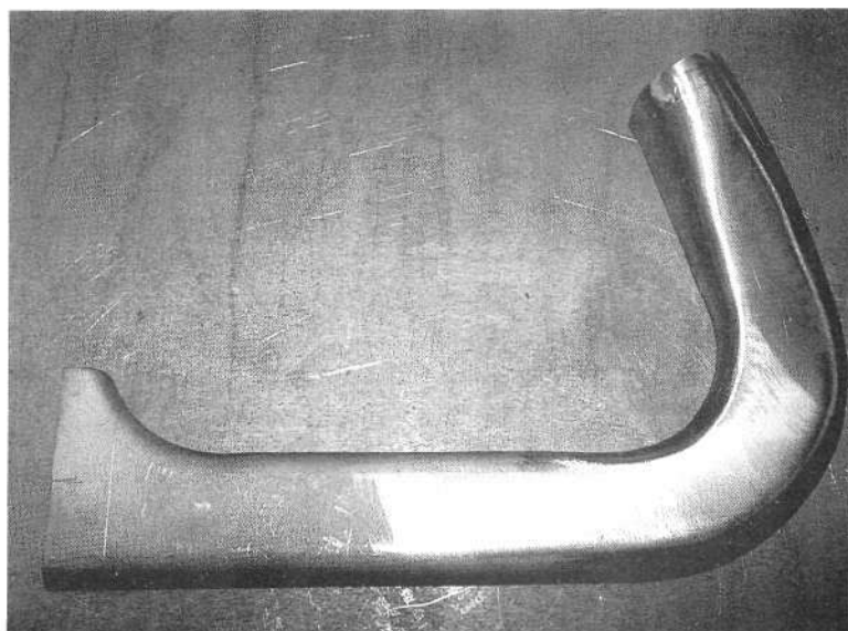
This pattern for the top hold down strip goes the full length of the part, but only up to the tangent. It's made this way so I can form the metal from where the bend begins.
