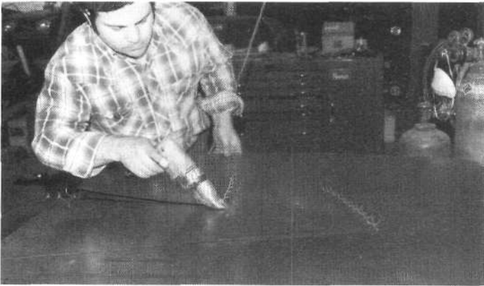
Electric shears make quick work of cutting floor blank. Material is 0.040-in. mild steel. Foot area has already been beaded.
