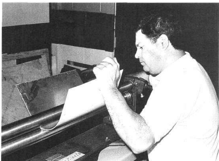
Tennsmith also makes a good 36-in. x 2-in. roller. I used it to roll the center part of an aluminum seat. Photo by Michael Lutfy.
