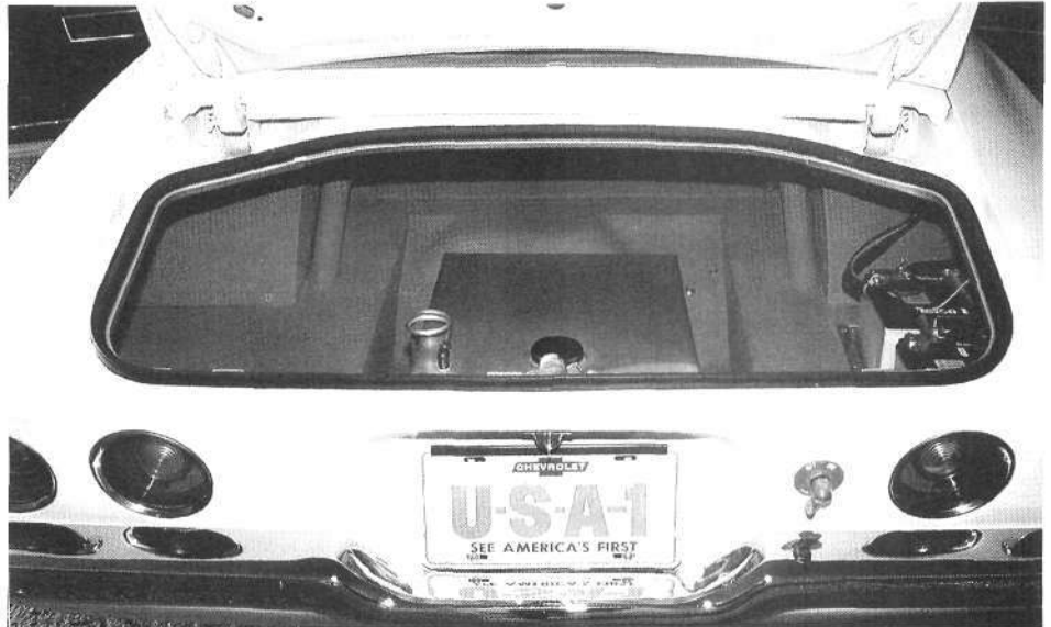
Most sheet metal on today's street machines is custom-made. The trunk of this Camaro features wheelhouses, rear firewall and fuel cell—all fabricated by hand. Photo by Jim Kelso.
