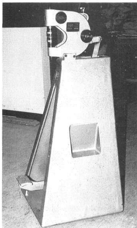
Recently U. S. Industrial Tool and Supply Co. and Eckold combined talents to produce a really great foot powered shrinker/stretcher.
