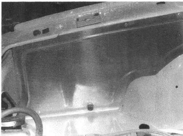
Bead simply follows the periphery of the panel. This type of bead is mainly for appearance.
