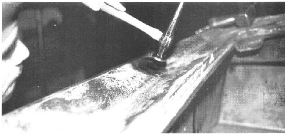
Don't stretch the metal in a patch by hammering too hard. Use the hammer, and the dolly held underneath, to level the patch's surface so it matches the fender.
