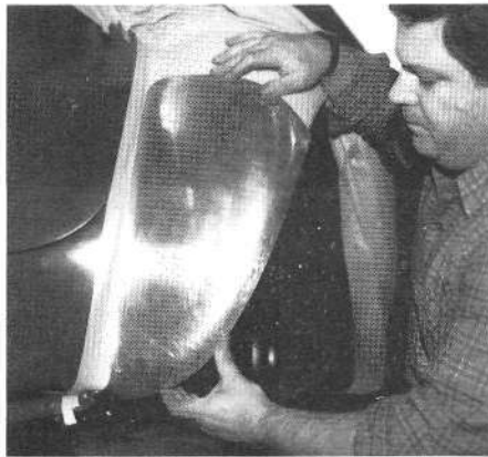
This Cobra fender guard shows what is possible once you master the English wheel.
