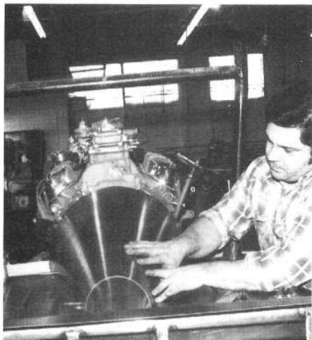
Checking transmission cover fit after Cleco-ing it in place. It fits well along the floor and is tight against the driveshaft tunnel.
