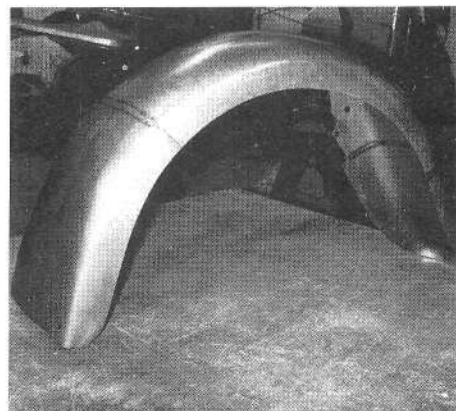
The entire fender was actually shaped from four individual pieces. Once all of the metal shaping is done, a wire is rolled into the fender edge for a finishing touch.
