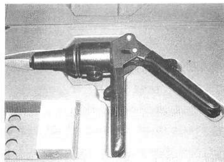
A hydraulic rivet gun will pull steel rivets up to 3/16" in dia. It will save a tremendous amount of energy pulling large rivets.
