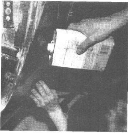
Neutralizing a surface after leading is extremely important. Any residue of tinning fluid or beeswax could make the final paint lift off the metal.
