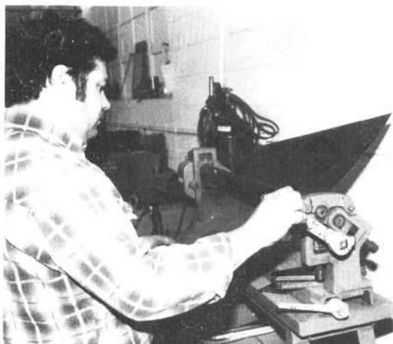
Rolling transmission cover requires that the roller be adjusted for more pressure at the small end to curve the blank into a cone.
