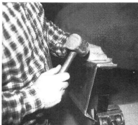
I started rolling the edge with a T-dolly held in a vise. I worked evenly all across the top and sides hammering gently, until the metal was halfway rolled under.
