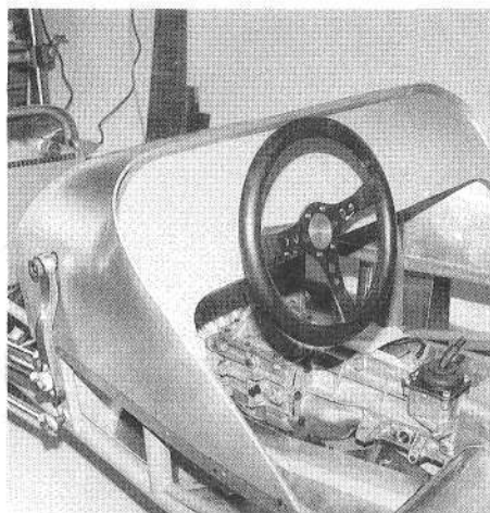
I made the body and all other aluminum parts for my own roadster from 3003-H14, 0.063-in. thick. It shapes and welds easily and holds up to road use.
