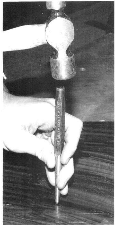
Hold a center punch vertical. Mark exactly where the center should be. Hit it firmly for a good mark.
