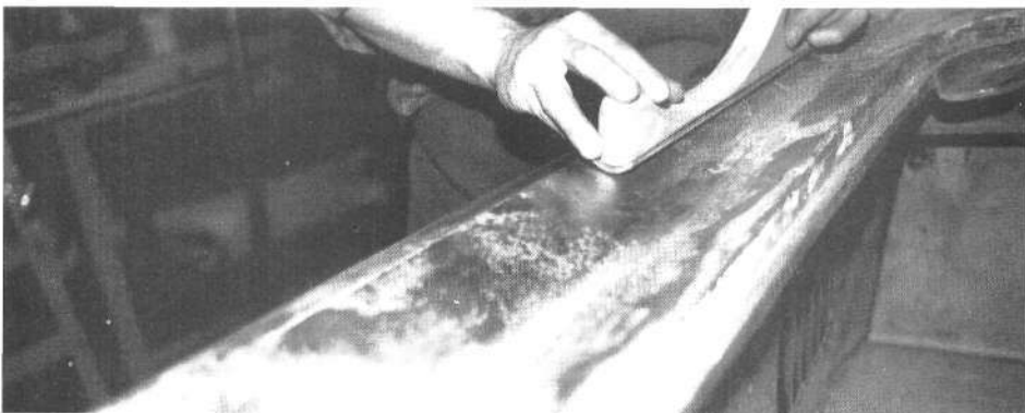
The last step in metal finishing a patch is using a vixen file to smooth the surface.
