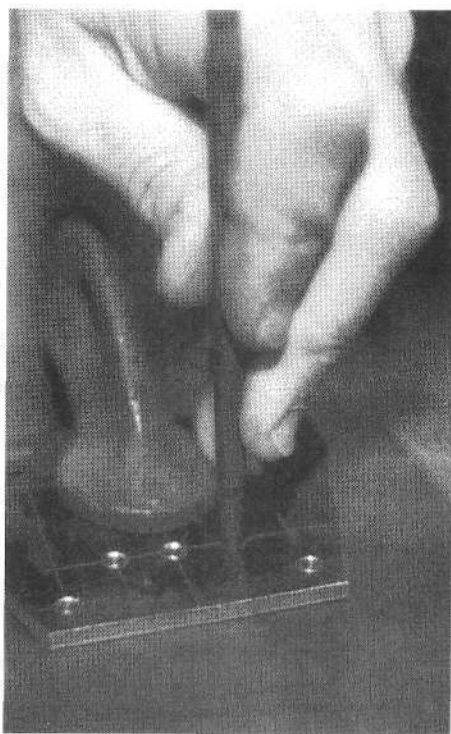
Transfer punches are a quick accurate way to transfer location information from a pattern to the metal.
