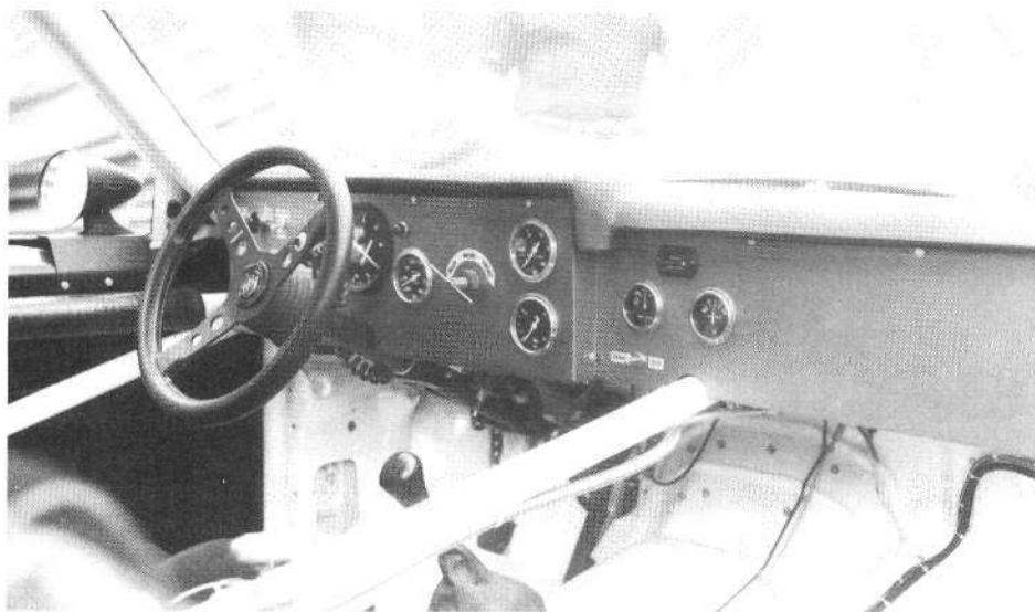
This GT racer retains stock floorpan as required by rules. Custom-fabricated aluminum instrument panel is anodized blue.
