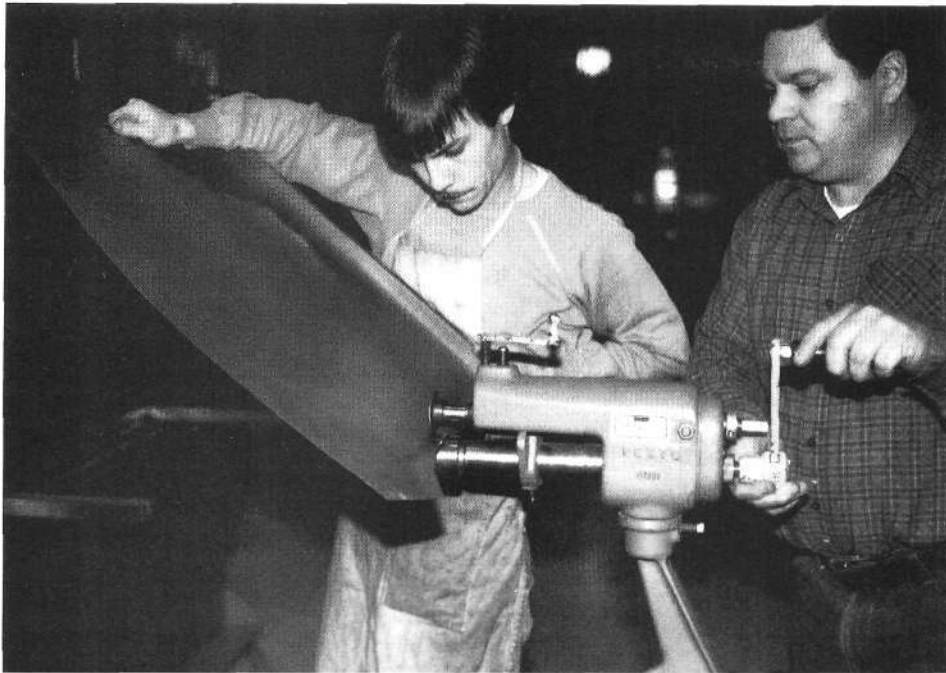
Steve Miller is actually indenting the metal so he can bend a curved flange. I'm just cranking to provide power while he tells me how slow or fast to crank. This teamwork can produce great results.
