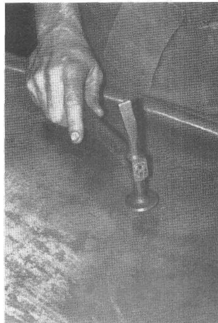
Scott Knight bumped up the dent with a dolly. Then he hammered and dollyed the metal until it formed a low, smooth swell.
