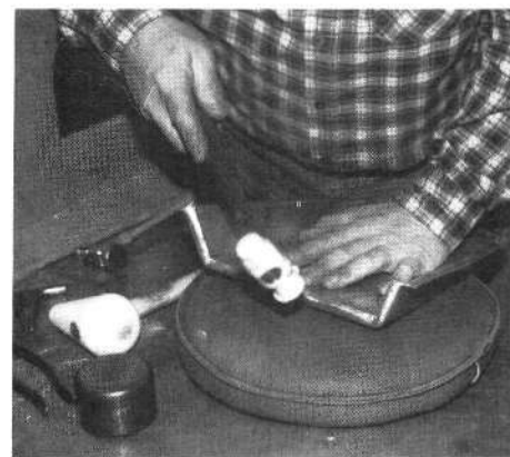
The scoop is resting on a leather shot bag so I won't scratch it. I used a teflon hammer to roll the metal the rest of the way under.
