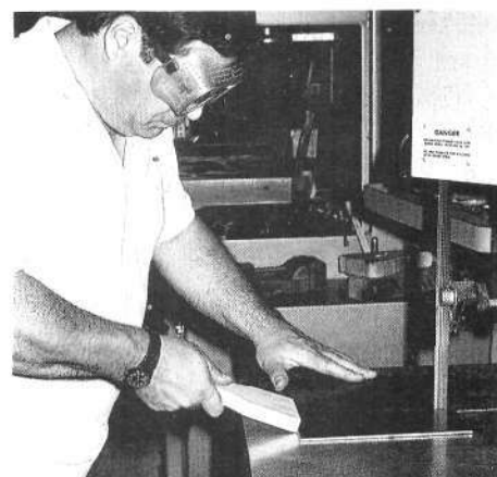
A cut-off type bandsaw is excellent for long, straight cuts. I'm using a push block and wearing safety goggles. Photo by Michael Lutfy.
