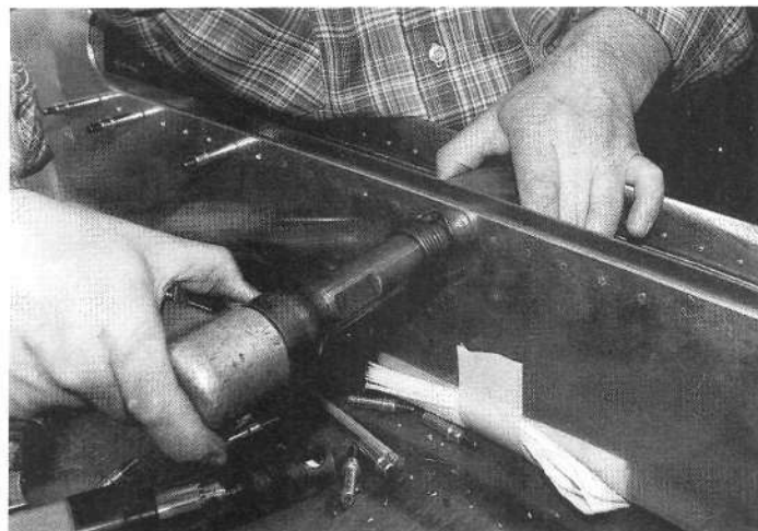
I'm tightly holding a bucking bar directly behind the rivet gun, exactly on center. This ensures an even shop head on the rivet.
