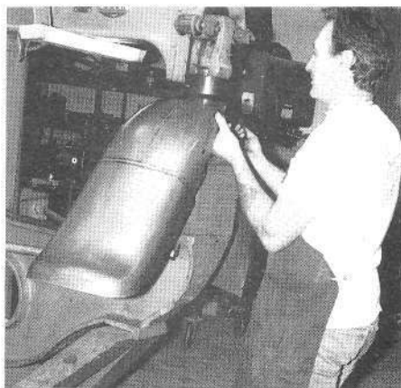
The Yoder power hammer can shape steel easily. A high crown die set was used to form this '32 Ford fender.
