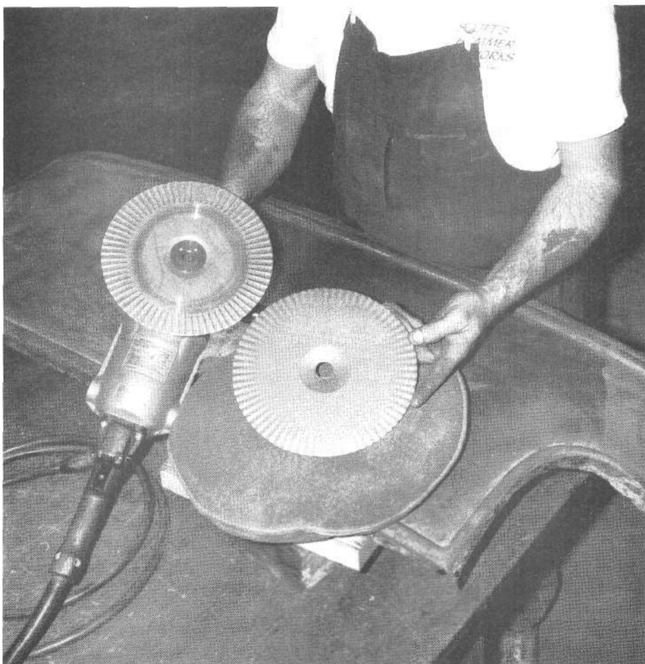
Scott Knight's special shrinking and leveling disk is not a magic wand, but he thinks it's as important to a body man's bag of tricks as his hammer and dolly. Notice how a shot bag is holding the panel down while Scott works.
