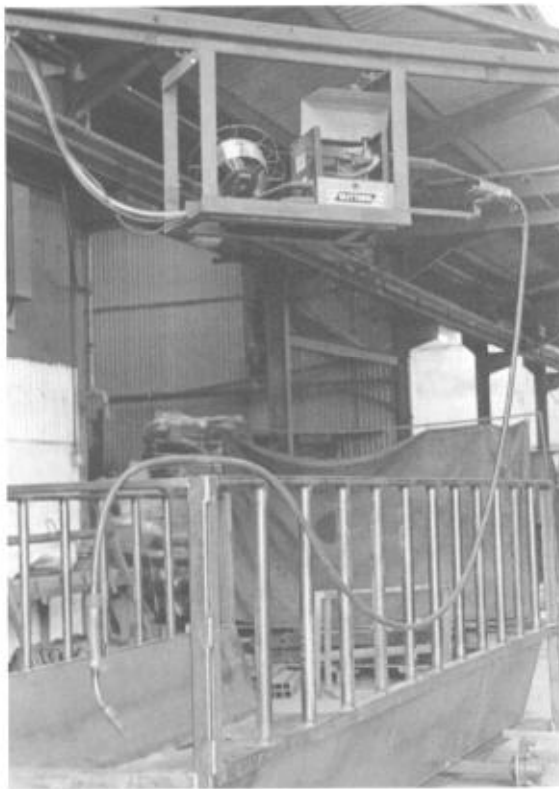
An industrial MIG welding situation with wire feed unit mounted on an overhead boom.
