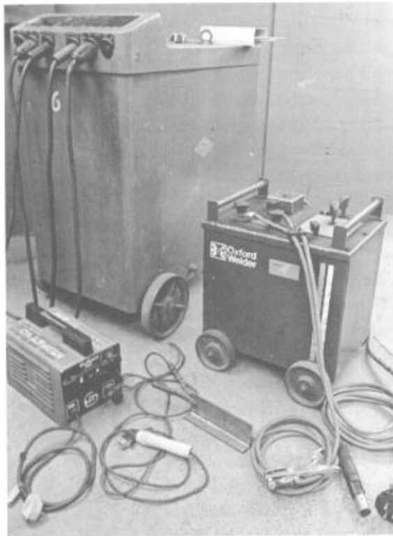
MMA welding sets from a DIY to a large 'double operator' set.
