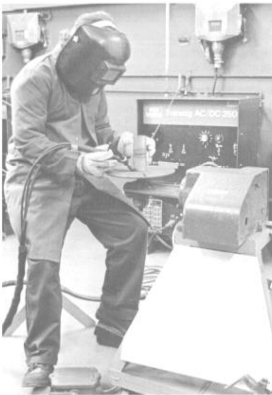
TIG welding can require all four limbs!
