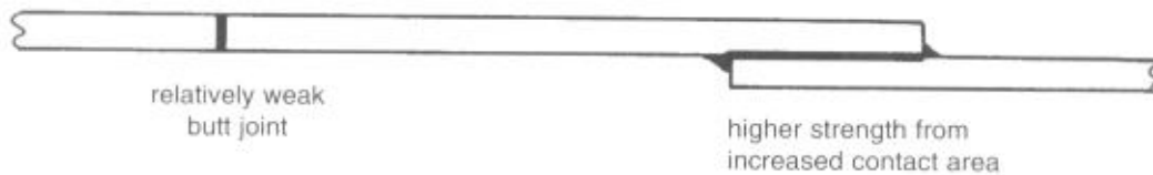
Joint design for soldering.
