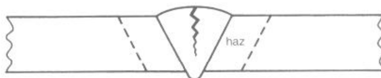
solidification (hot) cracking in a single V butt weld caused by sulphur or high restraint
