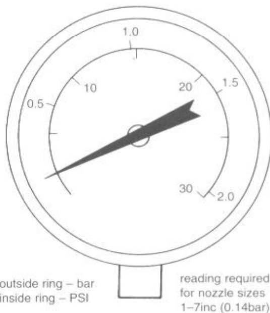
The delivery pressure gauge set typically on 0.14bar.
