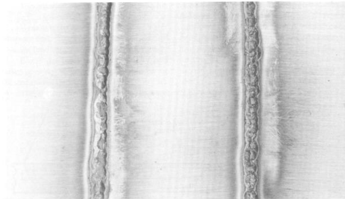
Underbeads of TIG welded butts in stainless steel with argon protection (left) and without protection (right).
