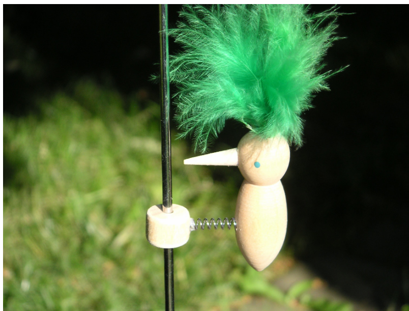
Fig. 12.10 At rest, this system is “self-braking.” If one swings the bird, the self-braking is intermittently removed and the fastener slides down the rod. This alternating change between sticking and sliding is an example of a sprag-slip movement.
