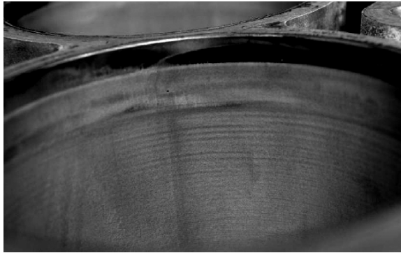
Fig. 13.2 Photograph of a cylinder in a combustion engine with “washboarding.”
