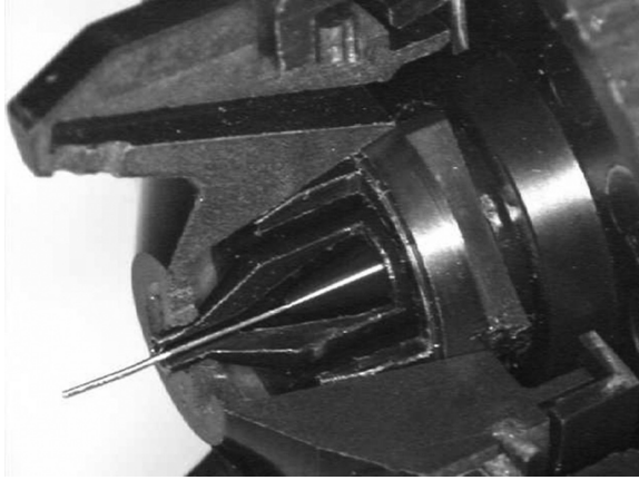
Figure 4.24 Internal charging of the paint
