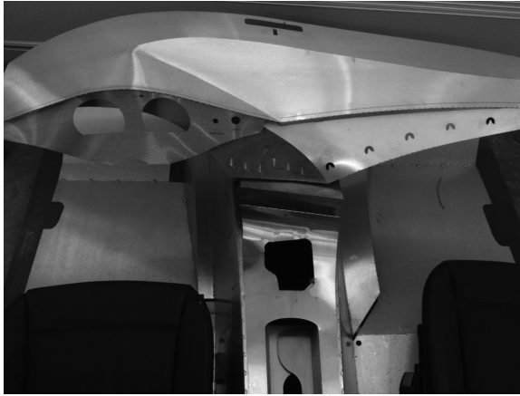
Figure 2.53 An example of the Industrial Origami dash panel
