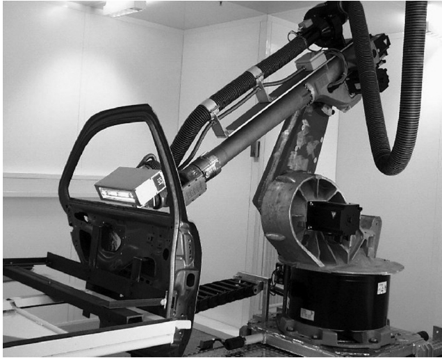
Figure 4.14 The UV curing robotic implementation
