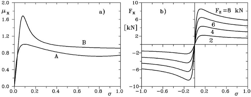
FIGURE 2.38. (a) Curves  $\mu_x(\sigma)$  for a 145 R 13 tire obtained with Eq. (2.24) (curve A) and for a 245/65 R 22.5 tire obtained from Fig. (2.25) (curve B). (b) Curves  $F_x(\sigma)$  for some values of vertical load Fig. (2.25) for a 205/60 R 15 V tire.
