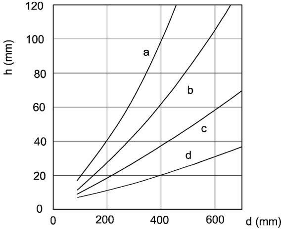
FIGURE 2.9. Effect of the average piston dimension  $d$  on sinking  $h$ , for different values of pressure  $p$ , on snow (curve a:  $p = 0.1$  MPa; curve b:  $p = 0.08$  MPa; curve c:  $p = 0.06$  MPa; curve d:  $p = 0.04$  MPa).
