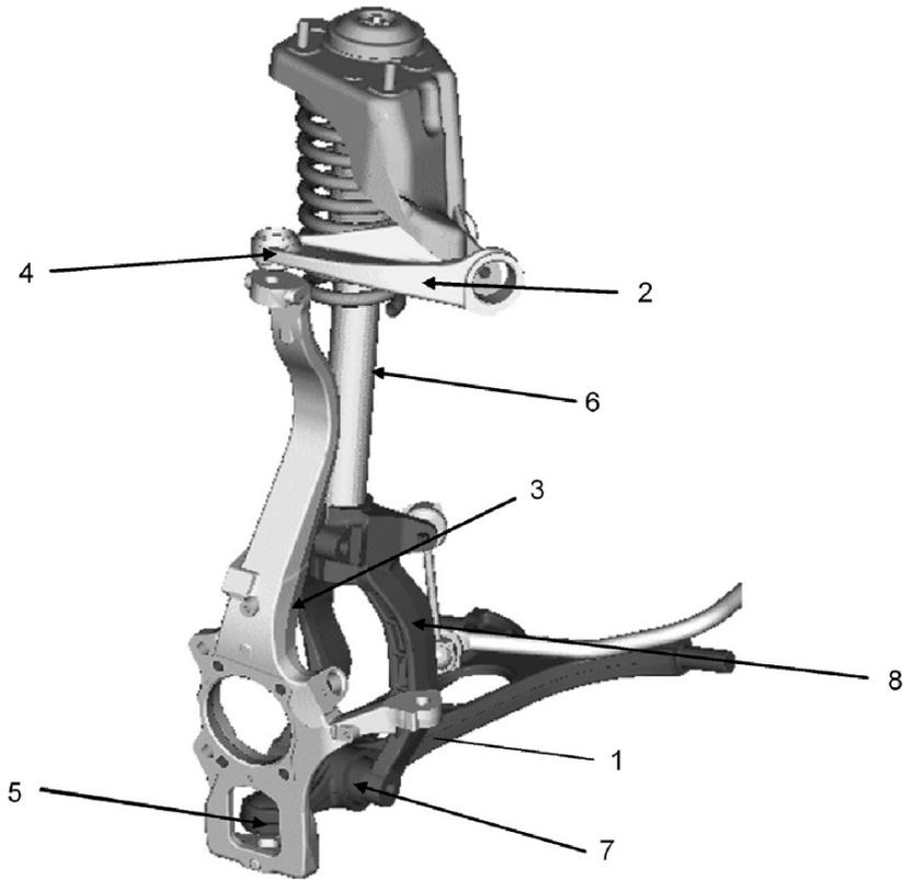
FIGURE 3.36. The lower arm 1 and the upper 2 are linked to the car body with rubber bushings. These arms are also linked, at the other end, to the strut 3, through spherical joints 4 and 5. The fork arm 8 connects the lower arm with the shock absorber (Alfa Romeo).
