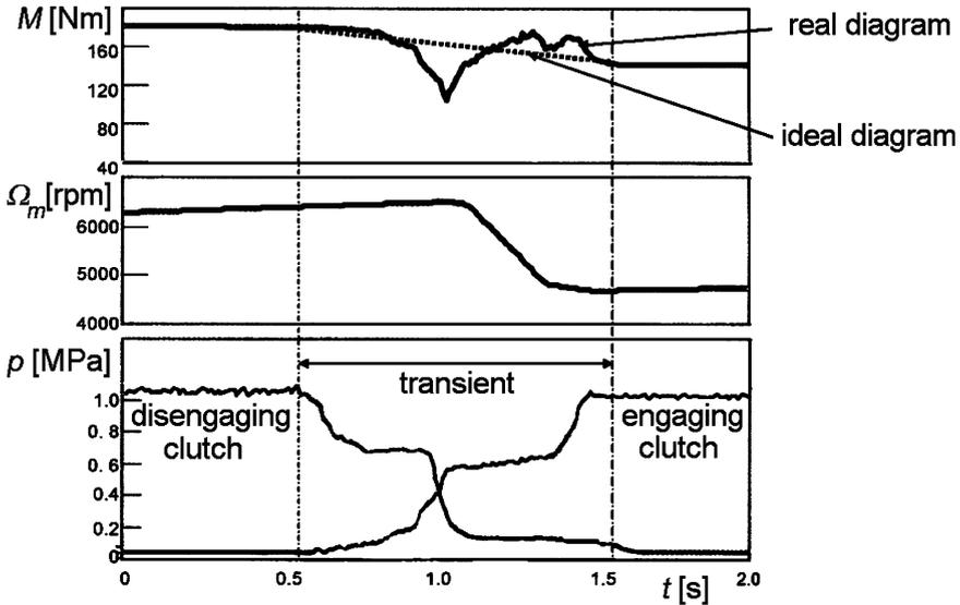
FIGURE 15.34. Diagram of the most important magnitudes involved in an upshift versus time  $t$ ; from the top, gearbox output torque  $M$  (real and ideal values), engine speed  $\Omega_m$  and oil pressure  $p$  on brakes are represented.
