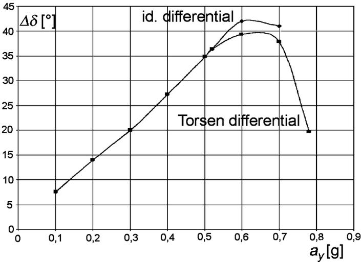
FIGURE 13.19. Understeer index diagram (the understeer index is assumed to be the difference  $\Delta\delta$  between the actual steering wheel angle and the zero speed steering angle) of a rear wheel driven car on a 200 m radius steering-pad in the case of ideal differential and Torsen differential. The zero speed steering angle is 13.6 deg for the ideal differential and 14.9 deg for the Torsen differential.
