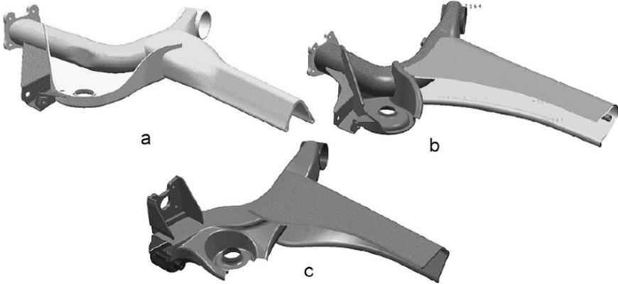
FIGURE 3.53. Design alternatives for a twist beam axle: (a) tubular type; (b) hybrid type; (c) Type made by stamped parts only.
