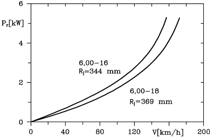
FIGURE 2.24. Influence of rolling radius on rolling resistance power  $P_r$ .  $F_z = 4.75$  kN,  $p = 250$  kPa.
