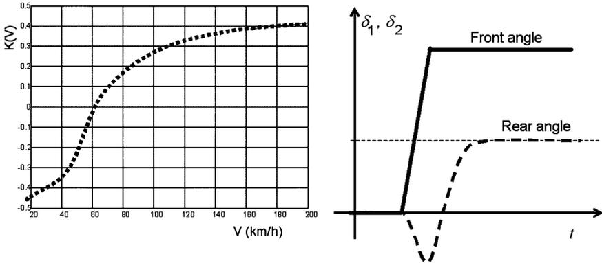
FIGURE 6.4. Diagram of the front and rear steering angles versus time in a steering transient with a dynamic speed dependent system.
