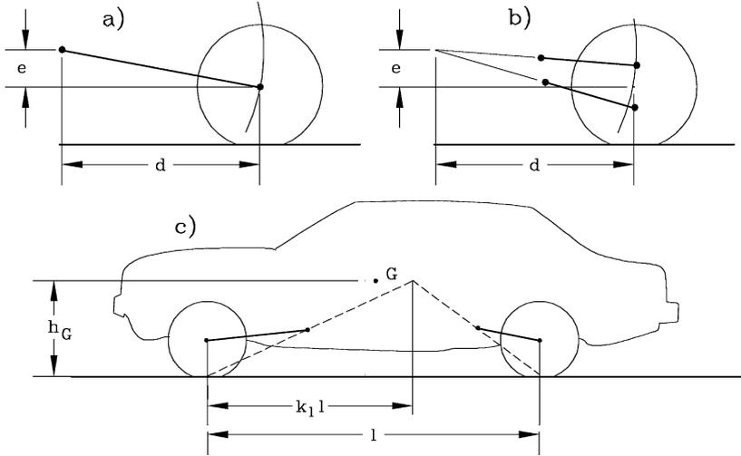
FIGURE 3.82. Relationship between  $\partial x/\partial z$  and suspension geometry, for trailing arms (a) and double wishbone (b) suspensions. If arms are parallel,  $d \rightarrow \infty$ . How to establish the anti-dive effect (c).
