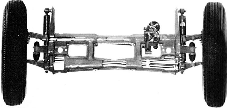
FIGURE 1.16. The Porsche suspension is made with two double trailing arms elements; it was developed in 1931 and produced by Volkswagen till the 1970s.
