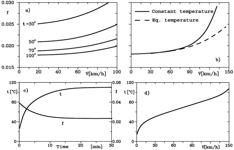
FIGURE 2.22. (a) Rolling resistance coefficient at constant temperature. (b) Comparison between  $f(V)$  at constant temperature and at equilibrium temperature for each speed. (c) Reduction of rolling resistance coefficient and temperature increase for increasing time at a speed of 185 km/h. (d) Equilibrium temperature as a function of speed.
