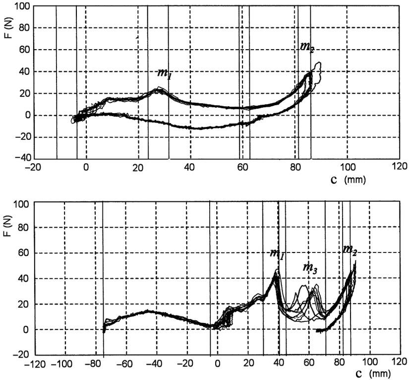
FIGURE 12.6. Diagrams representing shift stick knob force  $F$  (vertical axis) versus lever stroke  $c$  (horizontal axis) on a single stage gearbox with acceptable and unacceptable behavior (acceptable at the top, unacceptable at the bottom): In the second diagram the double shock phenomenon is announced by the third peak  $m_3$ .
