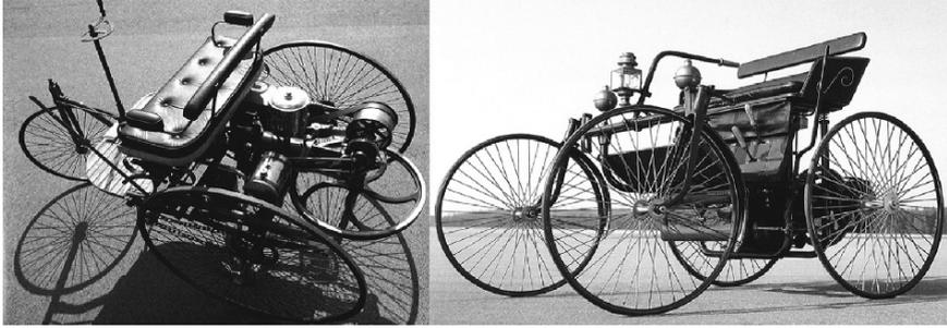
FIGURE 1.4. The first cars with an internal combustion engine, the tricycle of Benz and the *Stahlradwagen* of Daimler give no evidence of great attention to the suspension system. Both lack a front suspension and the second features no suspensions at all, with a suspended seat only.
