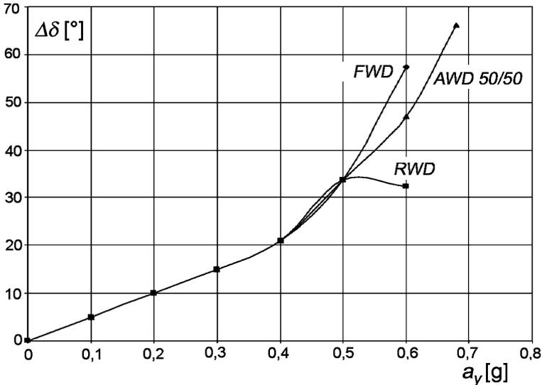
FIGURE 13.21. Diagram of the understeer index  $\Delta\delta$  as a function of the lateral acceleration  $a_y$  for the car in the previous examples, with a front wheel FWD, rear wheel RWD and all wheel drive AWD (50% of torque on each axle) with no friction transfer differential.
