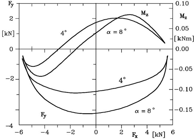
FIGURE 2.61. Polar diagrams of lateral force on the wheel at constant sideslip angle and self aligning torque as function of longitudinal force.
