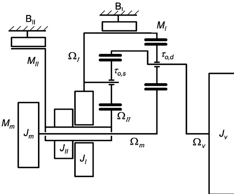
FIGURE 15.33. Epicyclic gear train scheme suitable for four speeds; the rotating masses involved in the shift from first to second speed are shown.
