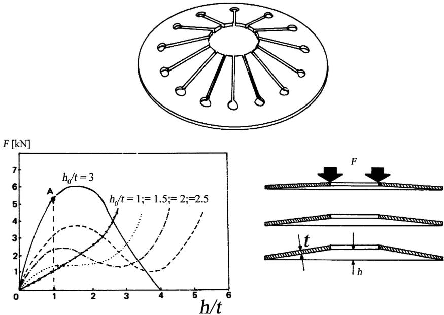
FIGURE 11.4. Diaphragm spring. On the graph at lower left is shown the elastic characteristic of springs as function of the actual height  $h$ , divided by the spring thickness  $t$ . Curves are parameterized in function of the aspect ratio  $h_0/t$ , where  $h_0$  is the unloaded spring height.
