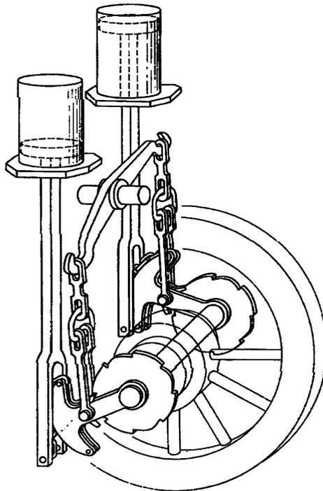
FIGURE 8.1. Drawing of the transmission mechanism from the piston to the wheel in the steam engine cart designed by Cugnot in 1769.
