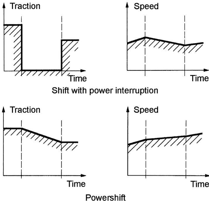
FIGURE 15.1. Qualitative diagrams of traction force and speed as a function of time for gear shift with interruption of power and powershifts.
