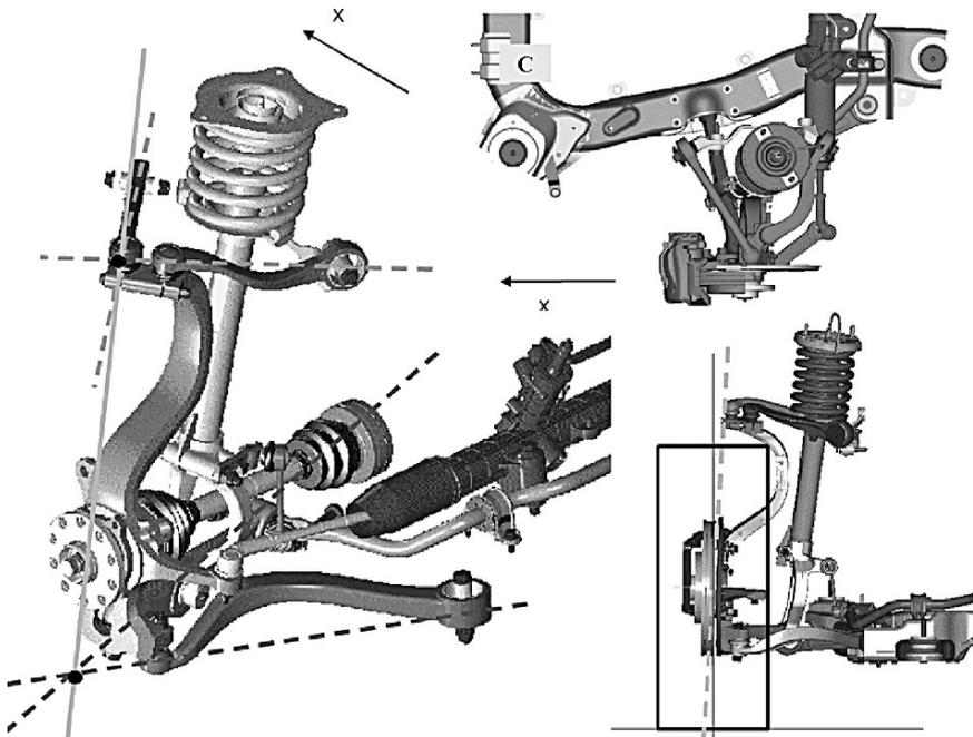
FIGURE 3.39. High double wishbone suspension with both virtual center suspension arms; the figure shows the geometrical construction needed to obtain king pin axis position (Lancia).
