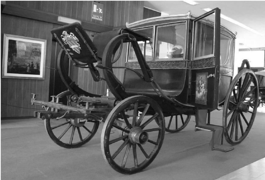
FIGURE 1.1. This coach built around 1650 shows the existence of a suspension; the sprung mass includes the passenger compartment only and is connected to the unsprung mass with four leaf springs with leader belts (Automobile Museum of Turin).
