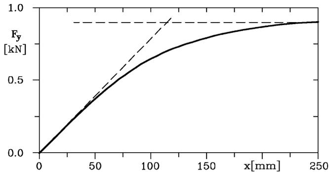
FIGURE 2.69. Lateral forces applied to a standing tire then put in rotation for various times or distances. Tire 140 12,  $F_z = 3.5$  kN,  $p = 138$  kPa.
