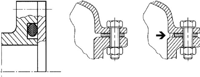
FIGURE 16.10. Examples of seals on covers; from the left, an O-ring seal for round covers, a pre-formed gasket and a gasket polymerized in situ.
