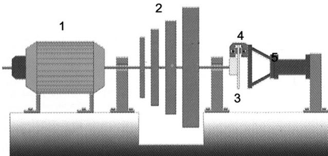
FIGURE 5.27. Scheme for testing a brake separated from its vehicle. The test bench includes a dynamometer and a set of flywheels simulating vehicle inertia.
