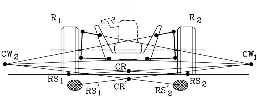
FIGURE 3.78. Position of roll center  $CR$  for a low double wishbone suspension with  $1'2'$  and  $3'4'$  arms parallel to the  $x$  axis.  $CR$ : position with rigid tires;  $CR'$ : position with deformable tires.
