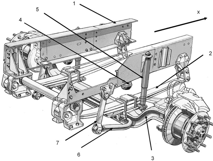
FIGURE 3.62. Design details of a front rigid axle suspension for an industrial vehicle (Iveco).
