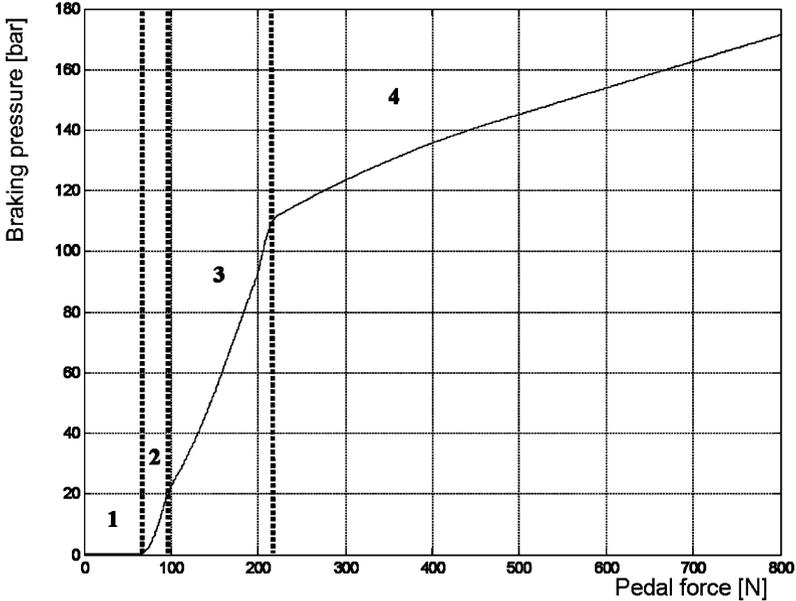
FIGURE 5.13. Example of the characteristic curve of a power brake; the braking pressure is shown as a function of the load applied on the pedal.
