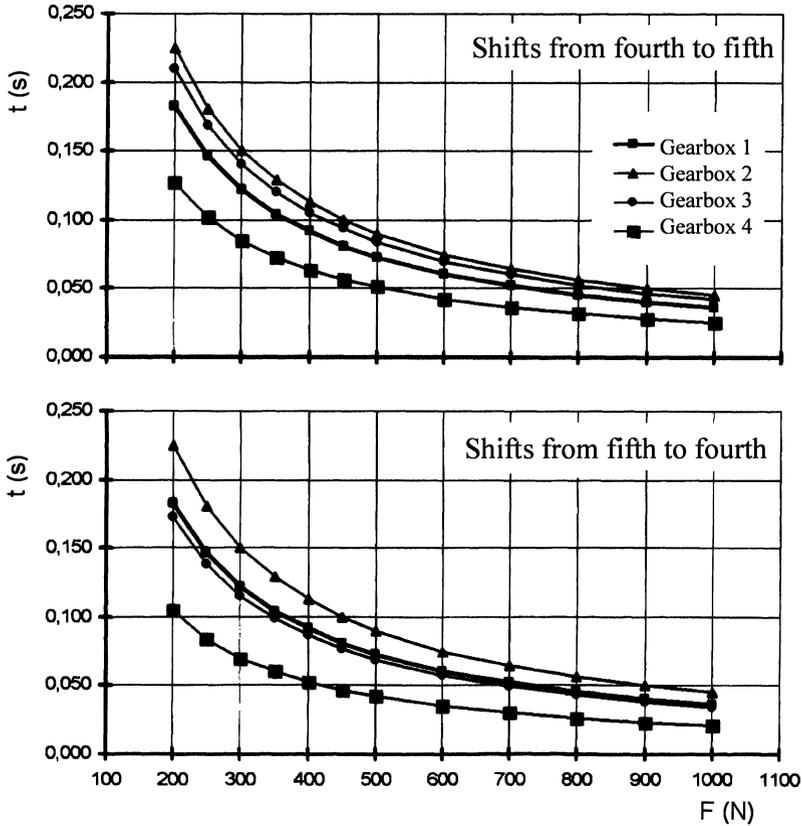
FIGURE 12.5. Diagrams representing synchronization time  $t$  (on the vertical axis) versus knob shifting force  $F$  (on the horizontal axis), for different single stage gearboxes and for shifts from fourth to fifth and vice versa.
