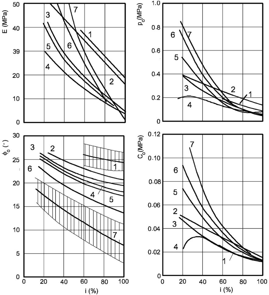
FIGURE 2.11. Primary identification parameters of the behavior of a natural ground, as a function of the relative content of water  $i$ ; curves with number 1 refer to a sandy loose soil, with 7 to a clayey soil, while numbers 2 to 6 refer to sandy soils with increasing sand content.
