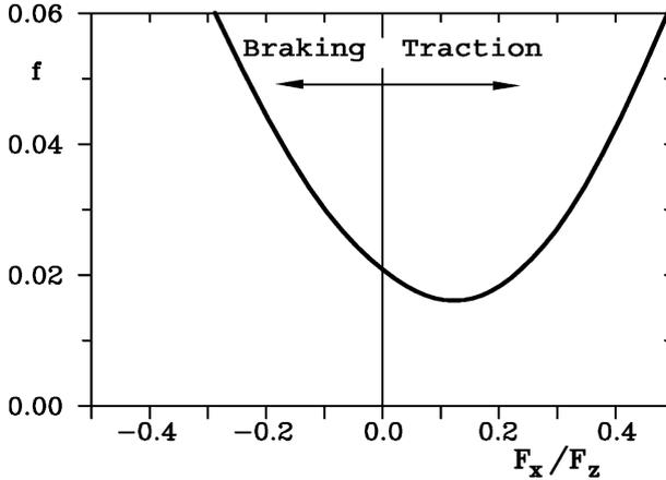
FIGURE 2.26. Rolling resistance coefficient as function of braking and traction force.
