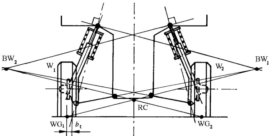
FIGURE 3.5. McPherson suspension. the figure shows the geometric construction to determine the roll center RC, not taking tire deformation into account.
