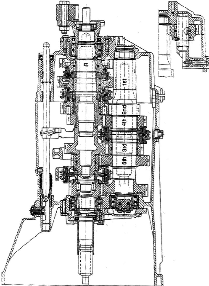
FIGURE 9.8. Double stage six speed gearbox (GETRAG).
