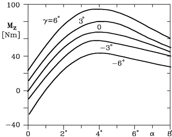
FIGURE 2.51. Self-aligning torque as a function of sideslip angle, for different camber angles. Radial tire 185 R 14,  $p = 230 \text{ kPa}$ ,  $F_z = 3.5 \text{ kN}$ .
