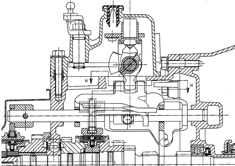
FIGURE 10.4. Cross section of a transversal gearbox; the forks of first and second speeds and of third and fourth speeds can slide on the bar of the fork of the fifth speed (FIAT).
