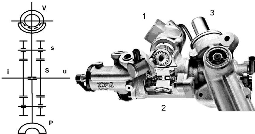
FIGURE 6.6. Actuator for front wheel steering control, made with an epicyclic gear adding to the steering wheel angle the contribution of an electric motor. At right the steering box; at left the kinematic scheme (BMW).
