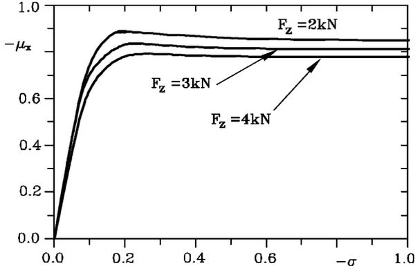
FIGURE 2.37. Influence of the vertical load  $F_z$  on function  $\mu_x(\sigma)$ . Tire 150 15,  $p = 170$  kPa,  $V = 100$  km/h.
