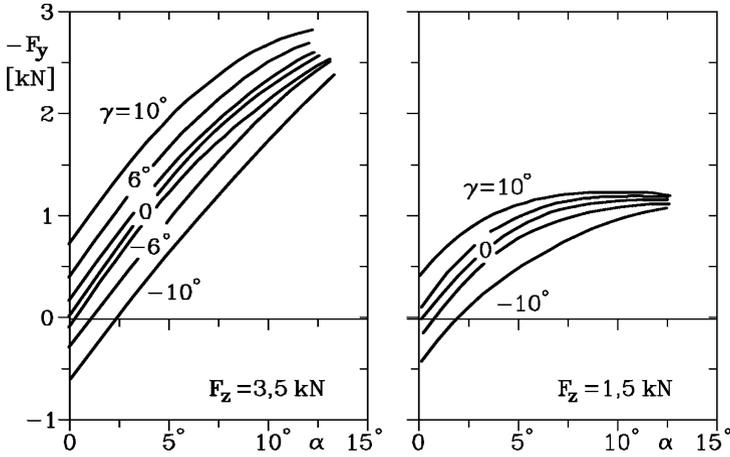
FIGURE 2.50. Cornering force as a function of the sideslip angle for different values of camber angle and for two values of the vertical force. Tire 135 13,  $p = 160 \text{ kPa}$ ,  $V = 40 \text{ km/h}$ .
