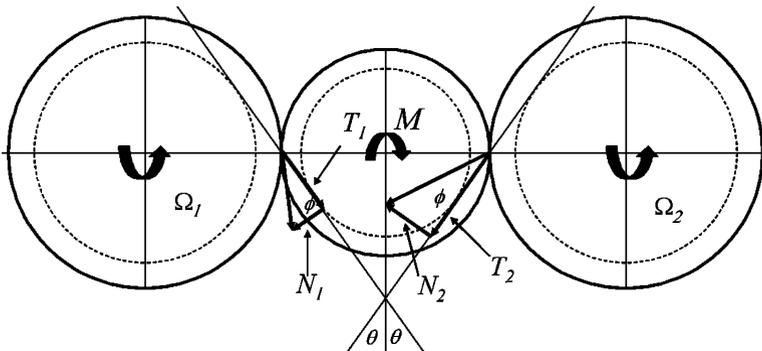
FIGURE 13.11. Scheme of forces acting on a bevel gear differential; reference planes of planet wheels are represented coincident with the reference planes of satellites.
