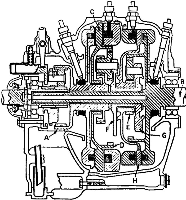
FIGURE 8.18. Semi-automatic gearbox produced by Cotal from 1934. The different elements of epicycloidal gears are braked by electromagnets; the reverse is engaged manually.
