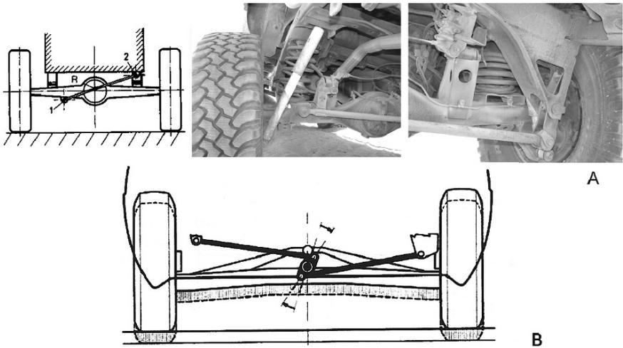
FIGURE 3.58. Systems for axle guidance; at top a Panhard bar; at bottom, a De Dion mechanism.
