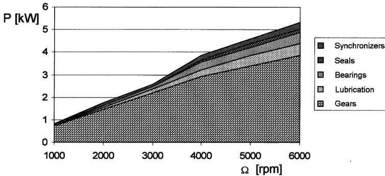
FIGURE 9.3. Contributions to total friction loss of a single stage gearbox designed for 300 Nm as function of input speed.
