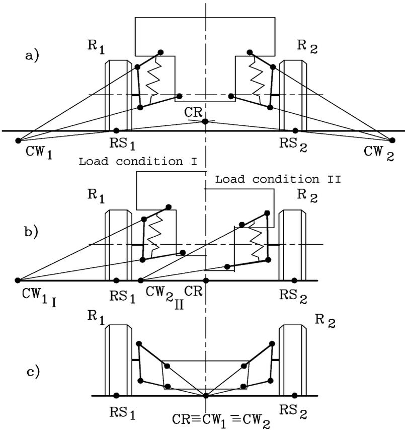
FIGURE 3.79. Low double wishbone suspensions.
