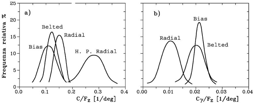
FIGURE 2.55. Frequency distribution of the cornering stiffness (a) and camber stiffness (b) for different car tire types.
