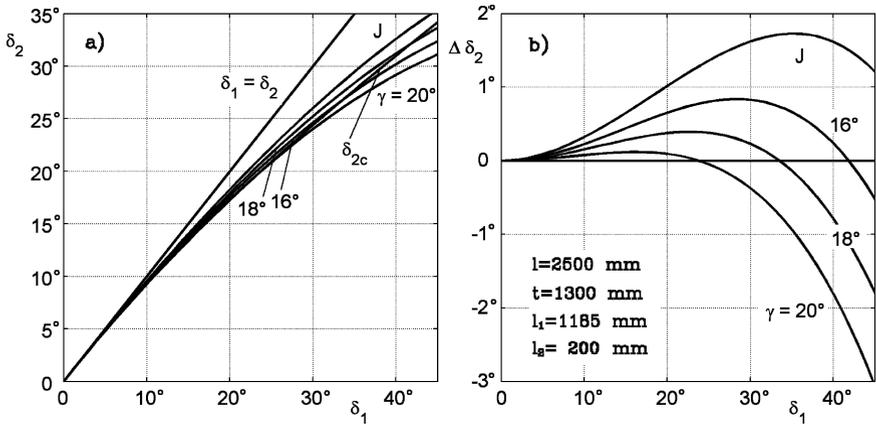
FIGURE 4.3. (a) Relationship  $\delta_2(\delta_1)$  obtained with the Jeantaud quadrilateral (curve J) compared with that obtained using the correct kinematic relationship and three different values of  $\gamma$ . (b) Steering error,  $\Delta\delta_2 = \delta_2 - \delta_{2c}$  as a function of  $\delta_1$  for the same steering systems.
