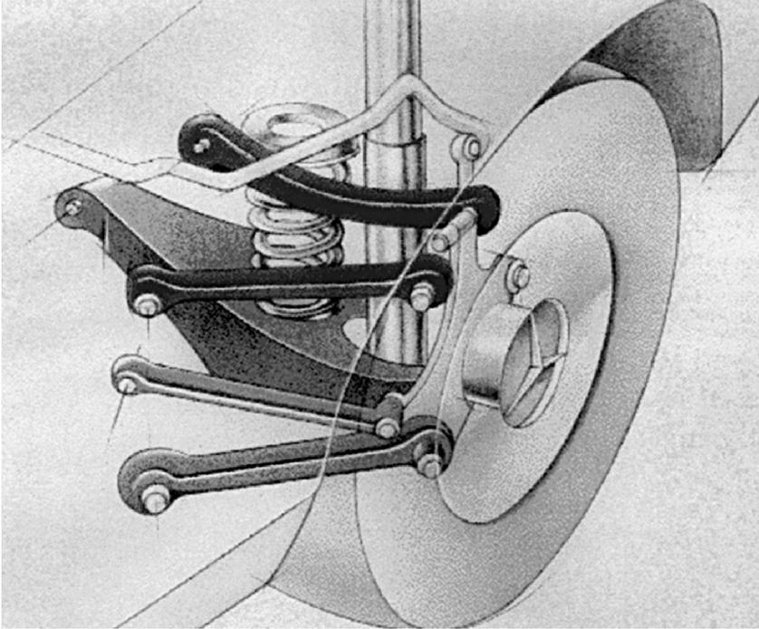
FIGURE 1.25. Multilink rear suspensions were first mass produced by Mercedes in 1982.
