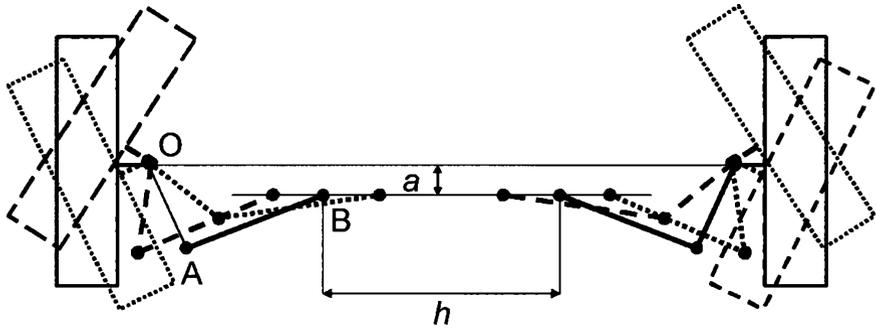
FIGURE 4.4. Kinematic scheme to calculate steering error by a rack and pinion steering box.
