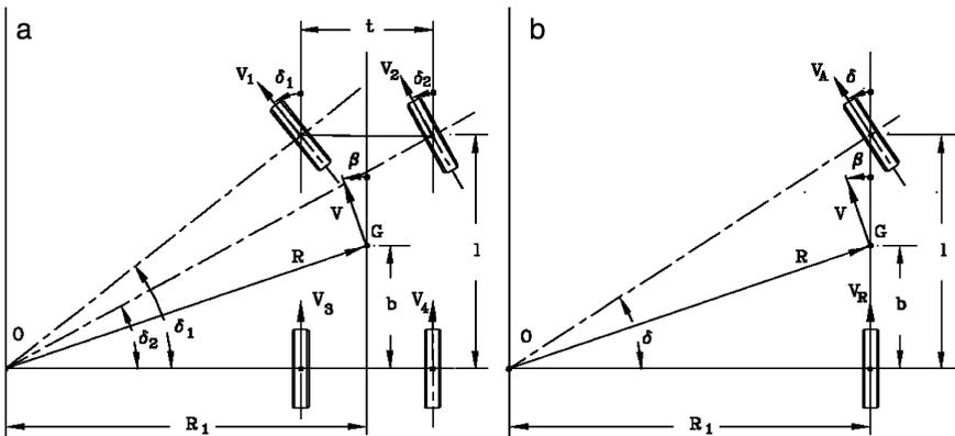
FIGURE 4.1. Kinematic steering of a four-wheeled and a two-wheeled vehicle.
