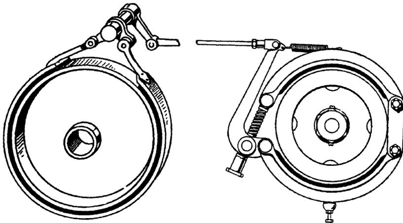
FIGURE 1.35. Band brakes and external shoe brakes, to be applied on the transmission line before the differential and final drive.
