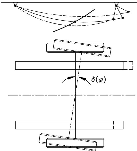
FIGURE 3.64. Roll steering of a rigid axle.
