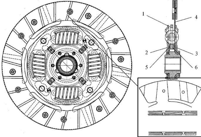
FIGURE 11.7. Driven plate (Valeo). The cross section shows the main and the auxiliary torsion dampers. The detail on the right shows how friction liners are mounted on the disc, in order to make the engagement progressive.
