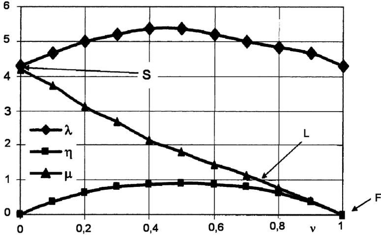
FIGURE 11.18. Characteristic curves of a torque converter representing  $\lambda$ ,  $\eta$  and  $\nu$  as a function of  $\nu$ .  $\lambda$  is multiplied by 10,000.
