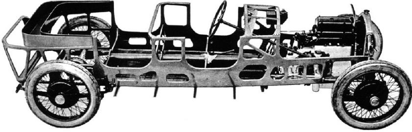
FIGURE 1.42. Complete chassis with parts of the unitized body of the Lancia Lambda of 1922. This picture is only for illustration; in fact, mechanical components were assembled to the structure only after the completion and painting of the body.
