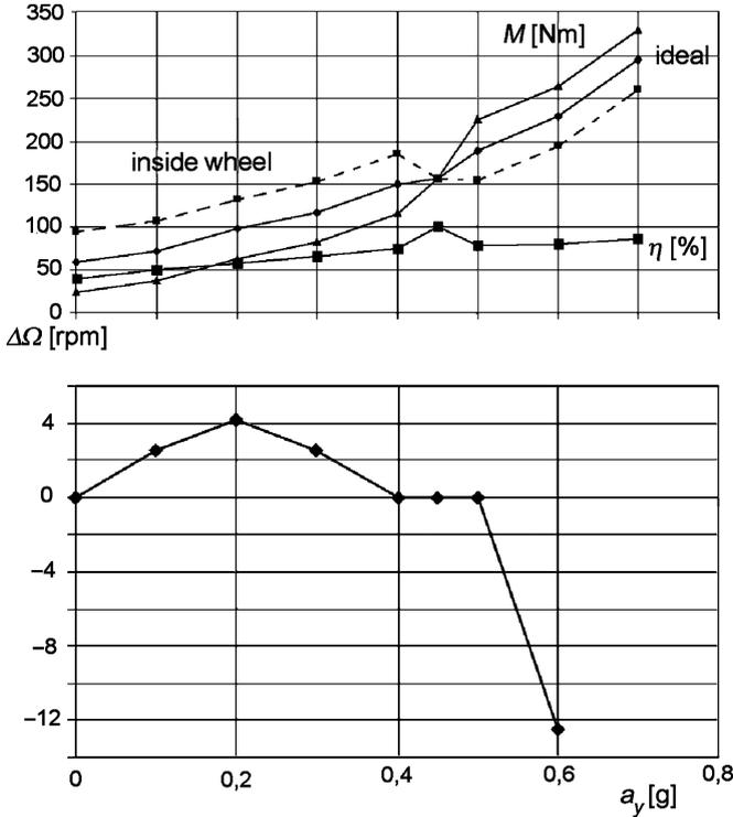
FIGURE 13.17. Upper figure: driving wheel torque  $M$  diagram and efficiency  $\eta$  diagram in the case of a pre-loaded differential; torque on inside (dotted line) and outside wheel can be compared with the ideal differential value without mechanical losses. Lower figure: speed difference  $\Delta\Omega$  between wheels.
