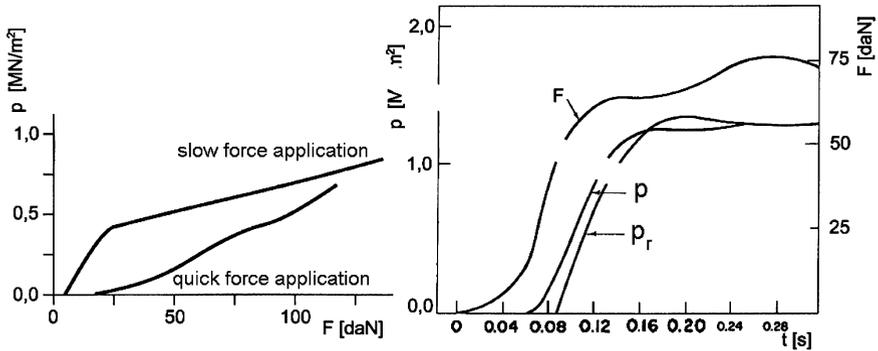
FIGURE 5.20. Left side: Quasi-steady and transient response of a vacuum power brake. Right side: Diagram of pedal force  $F$ , master cylinder pressure  $p$  and rear brake piston pressure  $p_r$  versus time.
