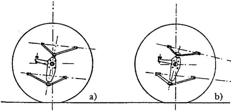
FIGURE 3.80. Low double wishbone suspension with non-horizontal articulation axis (a) and non-parallel axis (b). The inclination of these axis determines the position of the pitch center.
