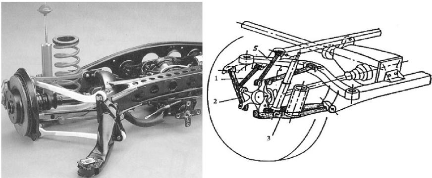
FIGURE 3.49. Classic multilink suspension for the rear axle of a rear wheel driven car, with five linkages, one for each degree of freedom subtracted from the wheel to allow the suspension stroke only (Mercedes).
