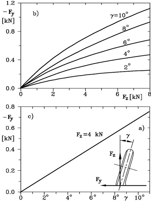
FIGURE 2.49. Camber force. (a) Scheme; note that  $F_y$  is negative and directed to the opposite as shown. Camber force as function of vertical load (b) and camber angle (c). Tire 165 13,  $p = 200$  kPa.
