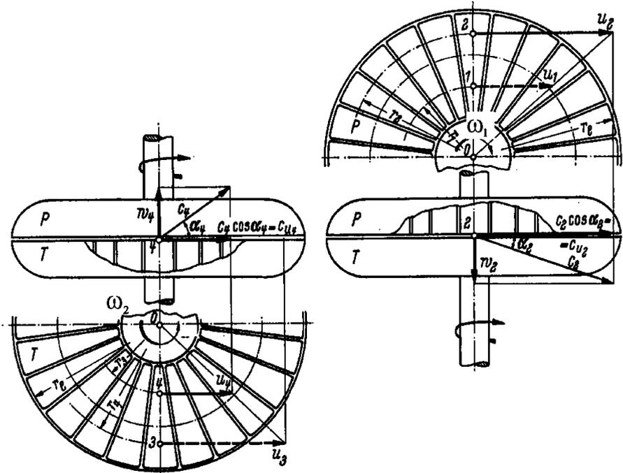
FIGURE 11.15. Speed triangles in a hydraulic clutch.
