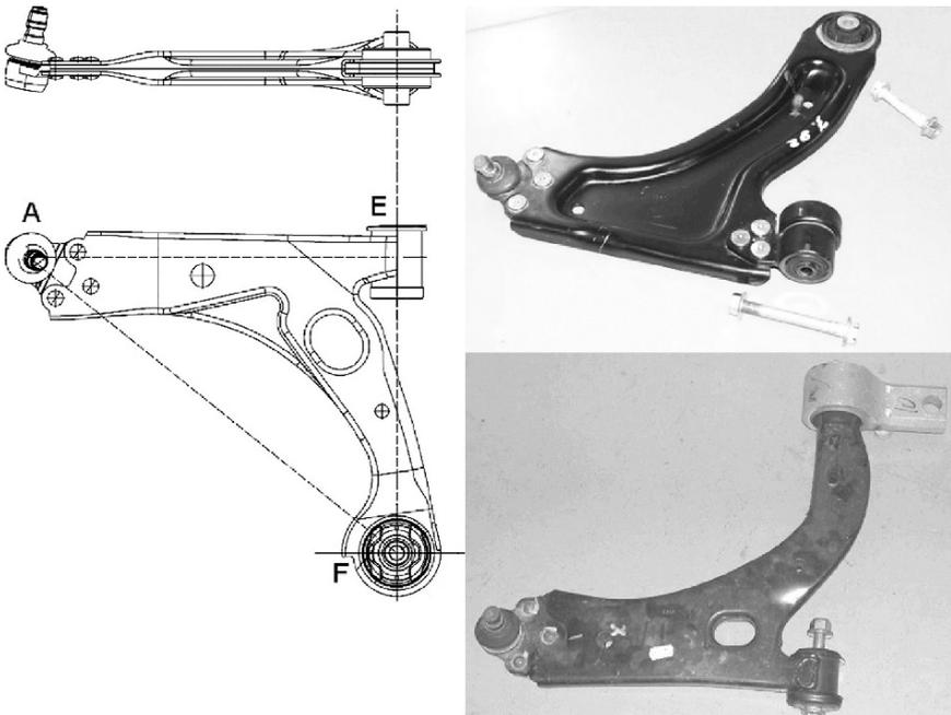
FIGURE 3.16. The banana like shape of the lower arm of the McPherson suspension is the result of a compromise between handling and comfort.
