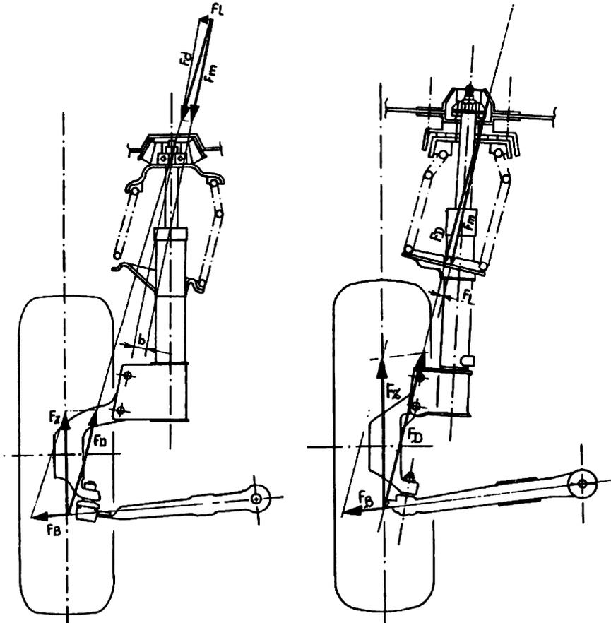
FIGURE 3.12. Scheme of McPherson suspension with integral (left) and double (right) thrust bearing.
