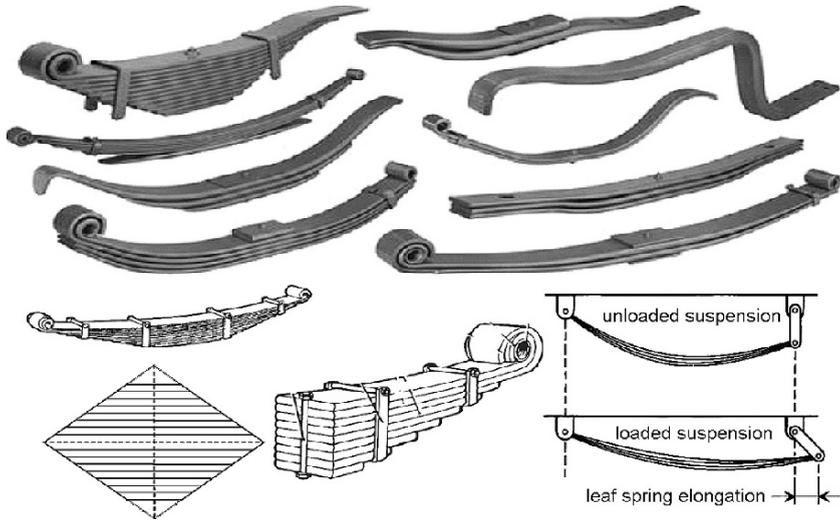
FIGURE 3.57. Different kinds of leaf springs for rigid axles (upper part); the scheme shown on the left at bottom shows how a semi-elliptic leaf spring can be seen as a uniform flexural strength body; the scheme on the left shows the motion of the leaf spring end because of suspension stroke.
