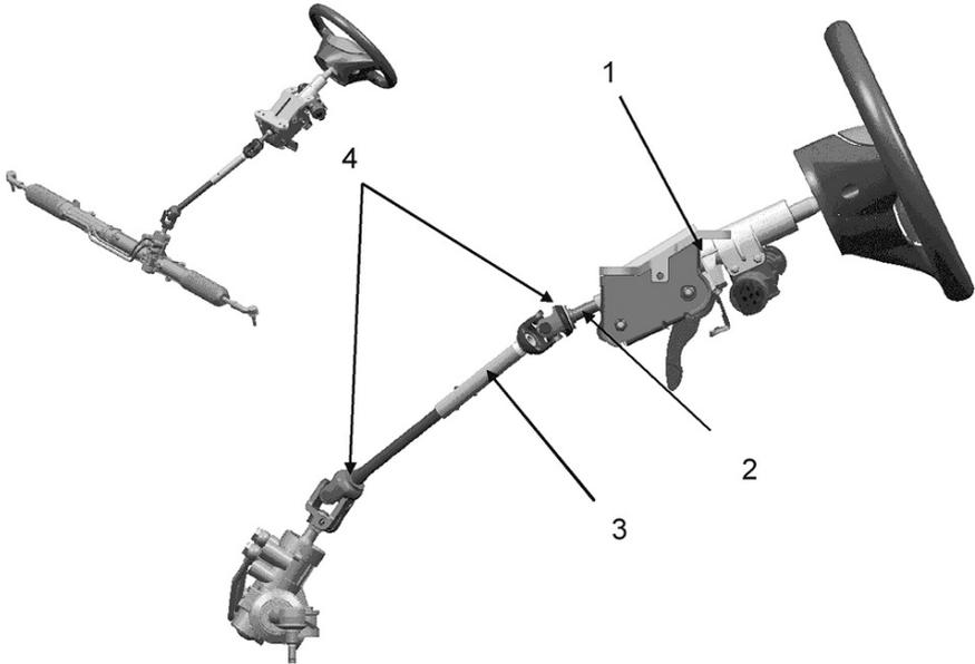
FIGURE 4.13. Steering column assembly, capable of adapting steering wheel position on the  $zx$  vertical plane. The miniature clarifies the inclined position of the middle section of the column, suitable to allow structural collapse with no intrusion of the steering wheel into the passenger compartment.
