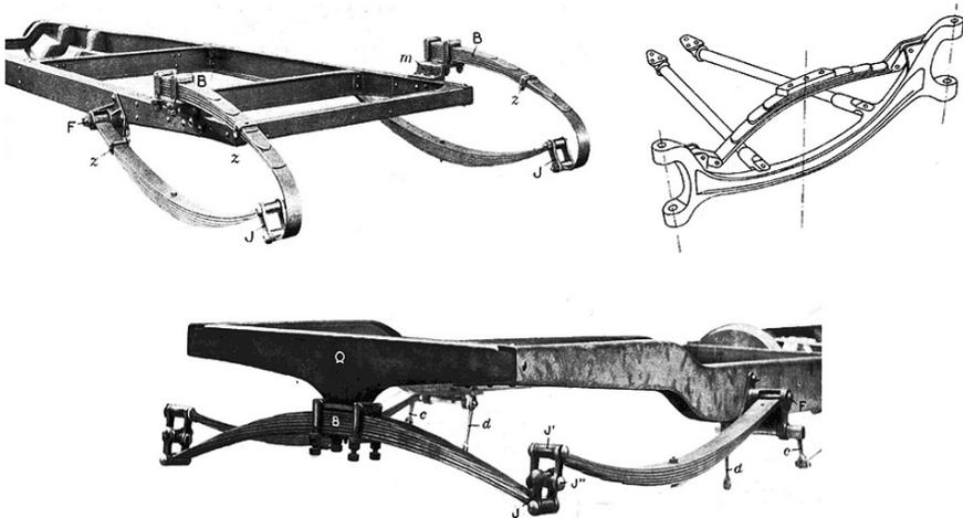
FIGURE 1.7. Some application schemes for leaf springs. On the top left is shown a  $\frac{3}{4}$  ellipse solution; on the right the Ford scheme with a single spring for each axle; at the bottom a three leaf spring solution equivalent to that of the  $\frac{3}{4}$  ellipse.
