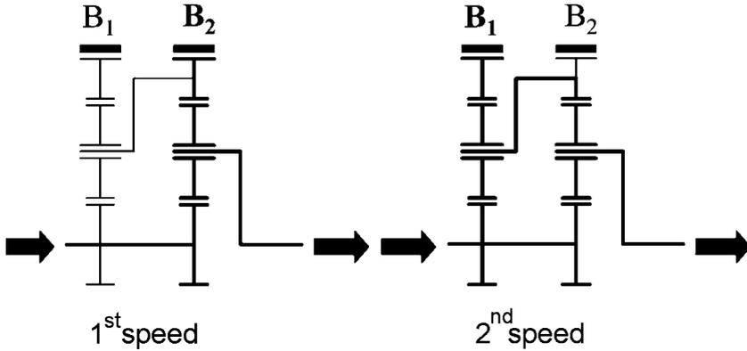
FIGURE 15.11. Scheme of a Wilson compound epicycloidal gear train; two speeds can be obtained by stopping one of the two annulus wheels with  $B_1$  and  $B_2$  band brakes.
