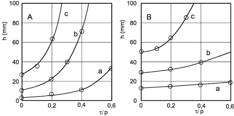
FIGURE 2.10. Piston sinking  $h$  due to the simultaneous presence of normal pressure  $p$  and shear pressure  $\tau$ , for a sandy soil (A) and a clayey soil (B). Curves a, b and c correspond to pressure  $p$  of 0.02, 0.03 and 0.04 MPa.
