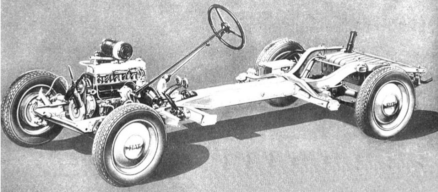
FIGURE 1.40. Central beam frame structure of Fiat 1500 of 1935; the structure is made of steel sheet pieces stamped and riveted to each other.
