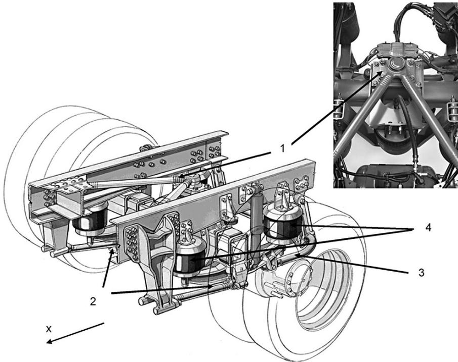
FIGURE 3.67. Rear suspension for a heavy duty industrial vehicle, featuring pneumatic springs; the axle is guided by an upper triangular arm and two lower longitudinal arms (Iveco).
