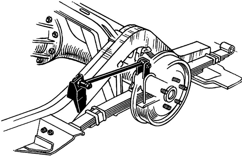
FIGURE 1.10. Example of a rigid axle with leaf springs, showing additional linkages for reducing axle steering and S deformation.
