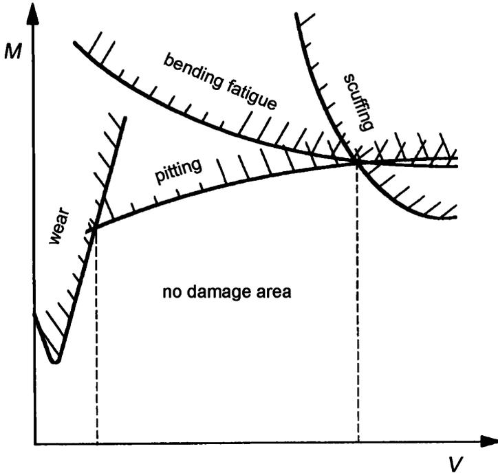
FIGURE 16.2. Qualitative diagram of the transmitted torque  $M$  as a function of circumferential speed  $V$  showing the typical shape of operation boundary curves for bending fatigue, pitting, scuffing and wear; the area below the curves envelope corresponds to operation without danger of damage. In consideration of the most likely speed values, pitting is the most important limiting condition.
