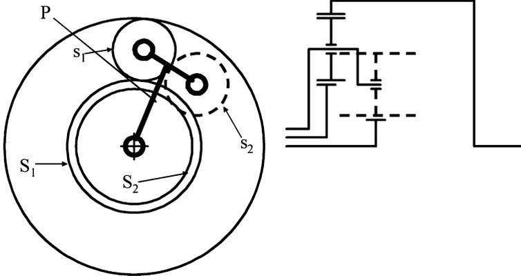
FIGURE 15.13. Scheme of a compound Ravigneaux epicyclical gear train; the satellite  $s_1$  is represented conventionally with dotted lines, because its drawing plane is not on the sketch plane.
