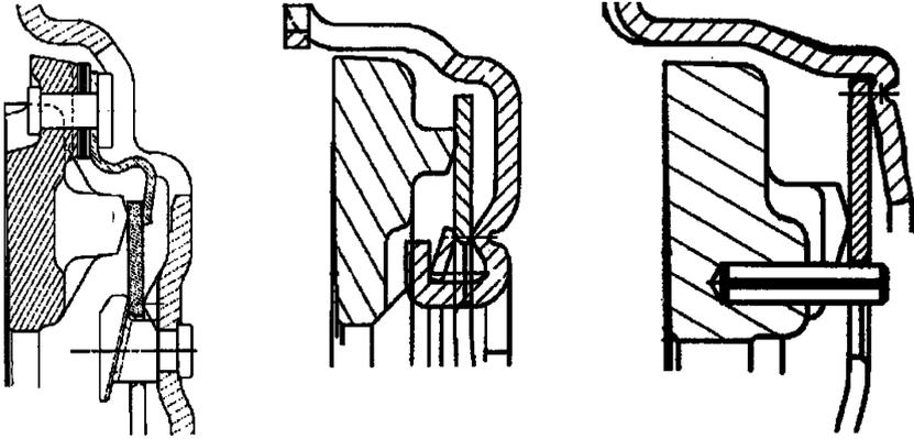
FIGURE 11.6. Internal disengagement mechanisms with pulled disc (the two drawings at left) and pushed disc. Different fulcrum types for the diaphragm spring are also shown.
