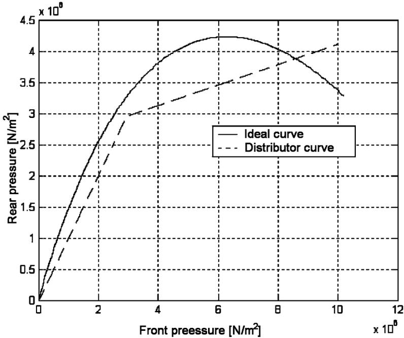
FIGURE 5.12. Comparison between the ideal distribution curve of braking pressure and the actual distributor curve.
