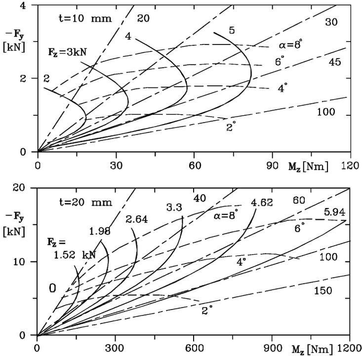
FIGURE 2.44. Gough diagrams. (a) Radial ply tire for a car 145 R 16;  $p = 180$  kPa,  $V = 50$  km/h; (b) cross ply tire for an industrial vehicle 300 20,  $p = 675$  kPa.
