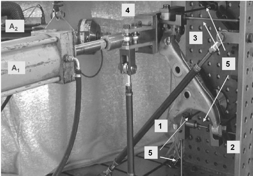
FIGURE 3.86. Fatigue test of a single suspension arm.
