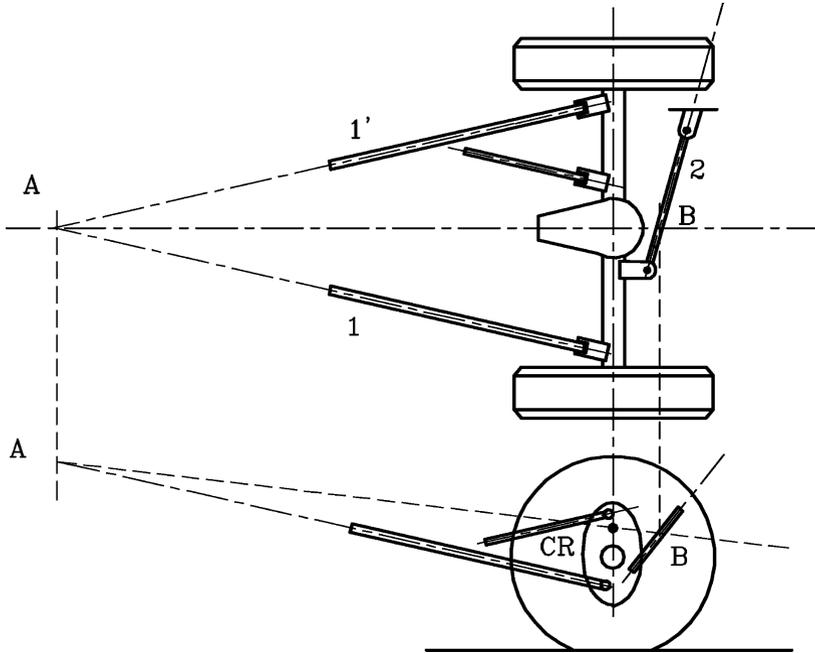
FIGURE 3.77. Three-link suspension. Position of point CR.
