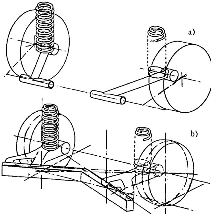
FIGURE 3.44. Trailing arm suspension (a) and semi-trailing arm suspension (b).
