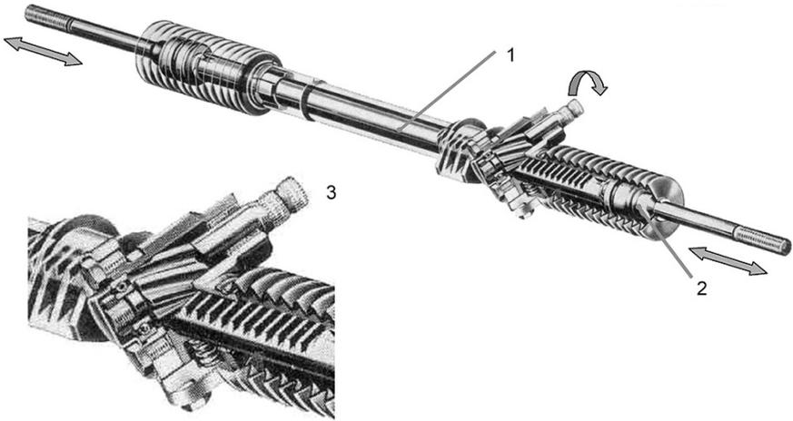
FIGURE 4.8. Rack and pinion steering box; the gearing point between rack and pinion is enlarged in the lower view.
