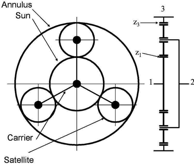
FIGURE 15.10. Scheme of a simple epicycloidal gear train.
