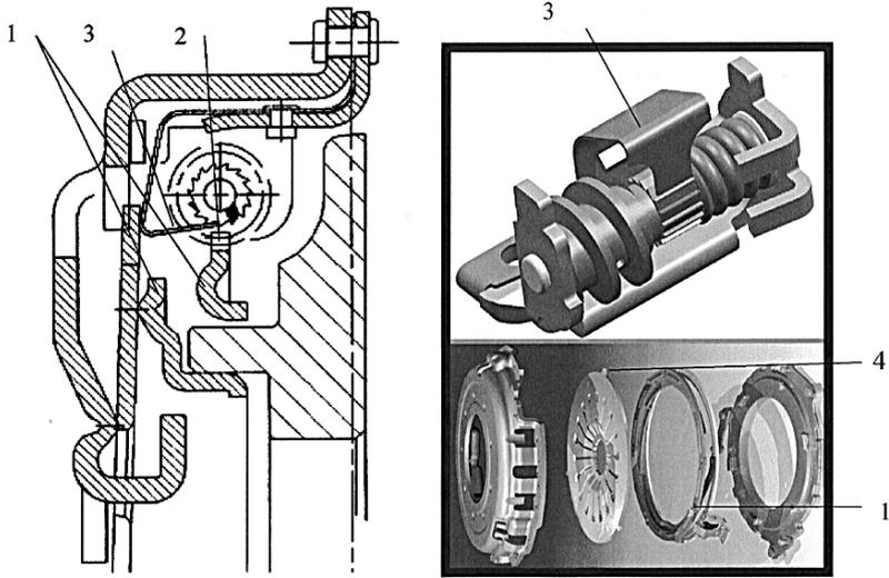
FIGURE 11.11. Self-adjusting mechanisms compensating for the effects of wear on the driven plate thickness (Valeo).
