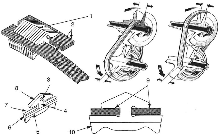
FIGURE 15.22. Detail of the pulley motion in a Van Doorne steel belt CVT (upper part); detail of the belt (lower side). The torque is transmitted by belt compression.
