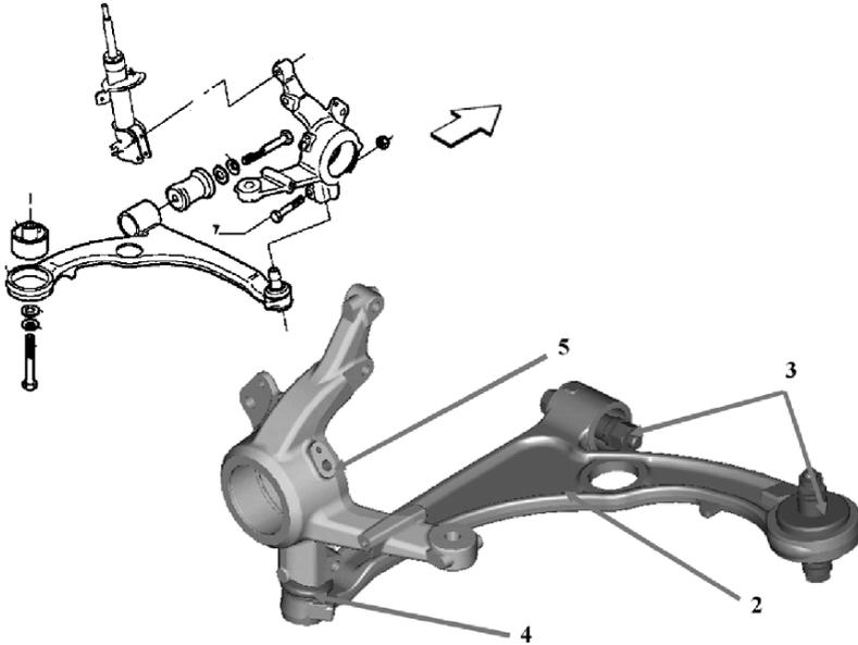
FIGURE 3.7. The lower arm 2 is connected to the subframe 1 in two different points, through elastic bushings 3; a spherical joint 4 links the arm to the strut 5.
