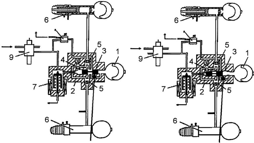
FIGURE 6.15. Scheme of hydraulic pneumatic suspensions, able to control vehicle trim and roll stiffness; in the A position (at left) the axle has a low roll stiffness, while in the B position (at right), the stiffness is higher (Citroën).
