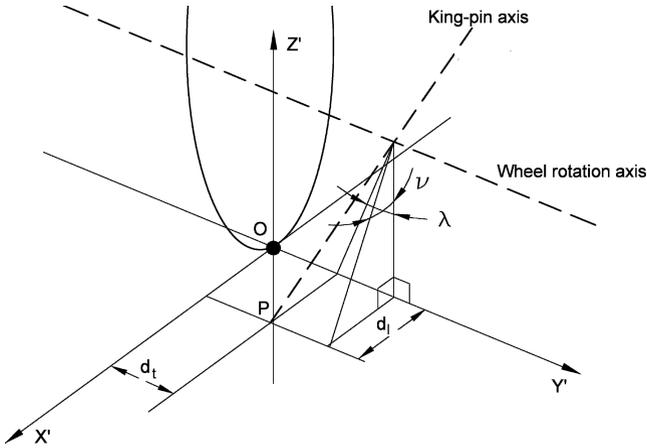
FIGURE 3.1. Steering geometry.
