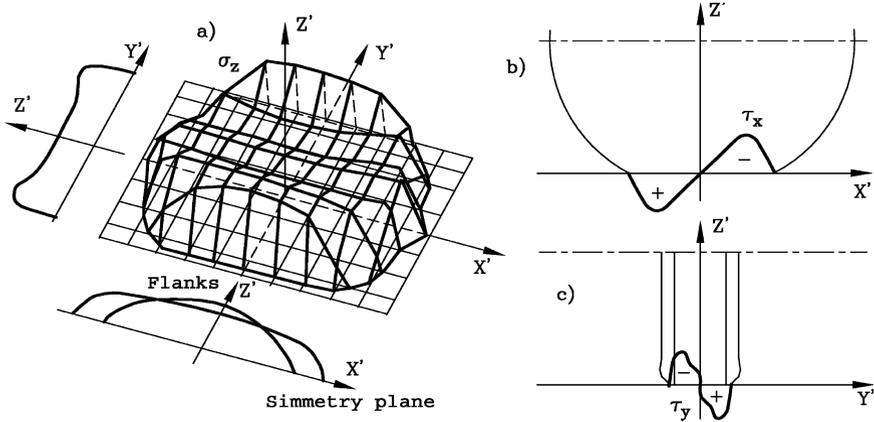
FIGURE 2.27. Force distribution in contact patch. (a) Normal pressure  $\sigma_z$ . (b) Tangential pressure  $\tau_x$  in the symmetry plane. (c)  $\tau_y$  and in the  $Y'Z'$  plane.
