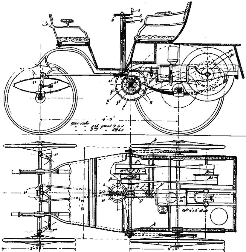
FIGURE 8.3. Two speed transmission of the Benz car in 1886, leather belt type. Two tensioners can shift belts from a position engaged with a driving pulley to that engaged with an idling pulley.
