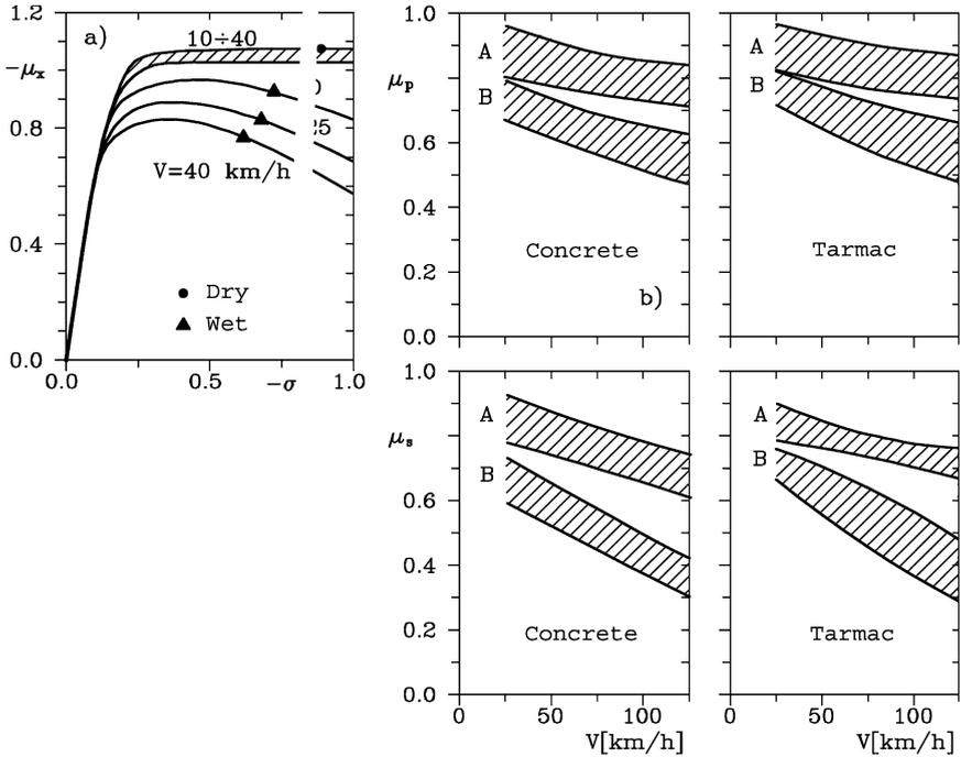
FIGURE 2.34. Influence of car speed on  $\mu_p$  and  $\mu_s$  on wet and dry road. Cross and bias ply tires 165 l5 e 150 R l5 with  $F_z = 3,75$  kN.
