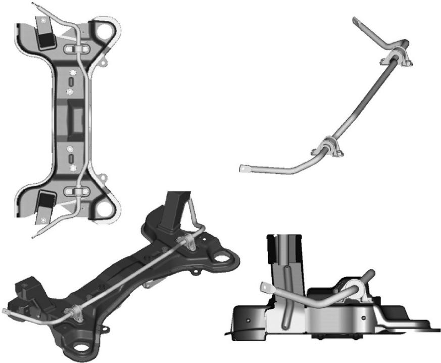
FIGURE 3.26. Anti-roll bar mounted on the suspension subframe.
