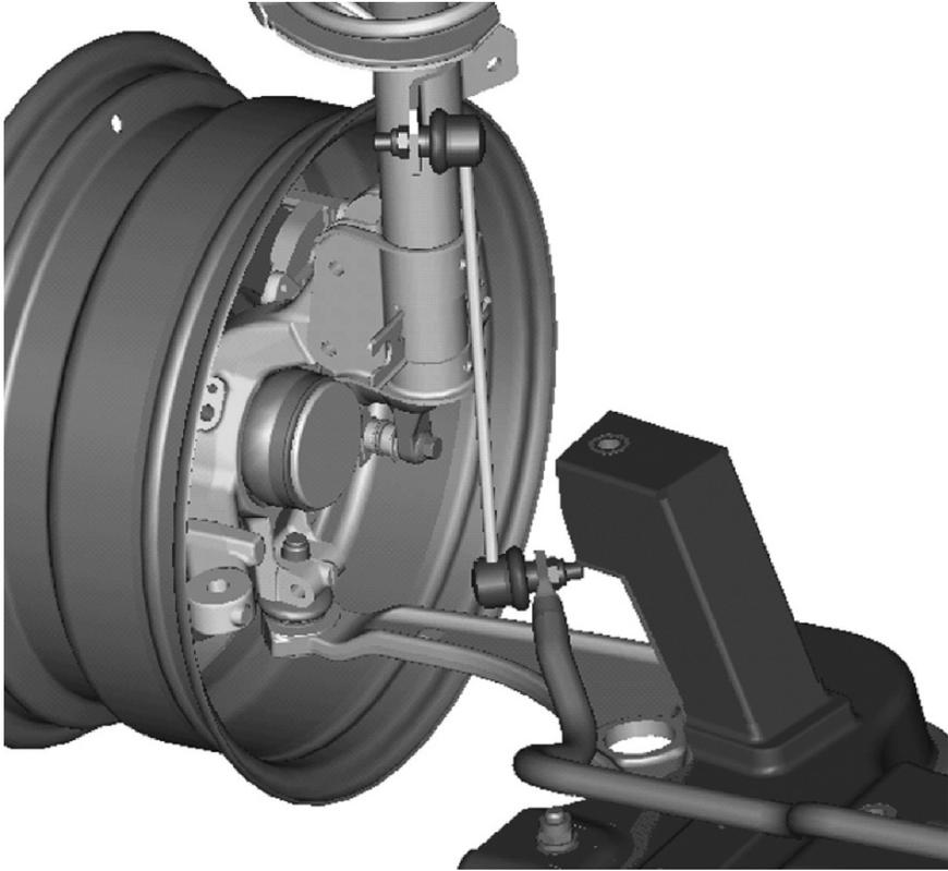
FIGURE 3.27. Anti-roll bar connected to the shock absorber through a pendulum bar.
