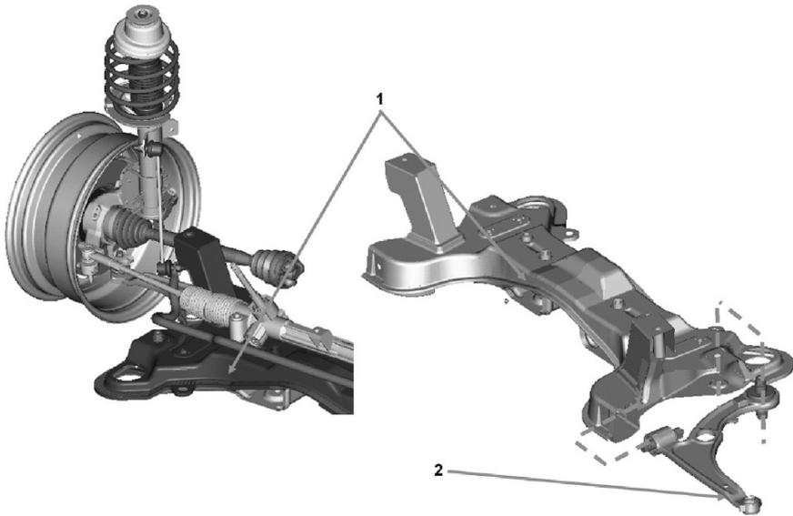
FIGURE 3.6. McPherson suspension for the front axle of a medium size front driven car; the lower arm (2) is articulated to the body through an auxiliary frame also called the subframe (FIAT).
