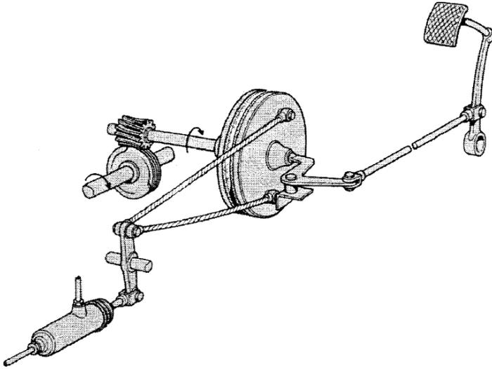
FIGURE 1.38. A mechanical power brake adopted by Rolls-Royce; the necessary energy derives from the propeller shaft and is transferred to the braking system by a clutch, operated by the brake pedal.
