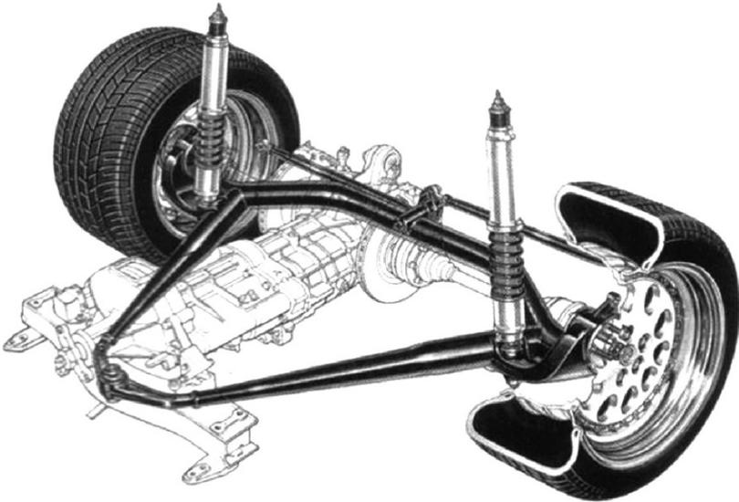
FIGURE 1.21. A particularly elegant example of a rigid rear axle is provided by Alfa Romeo. This scheme was adopted on different cars starting from the 1970s. It can be considered an improvement of the De Dion-Bouton suspension.
