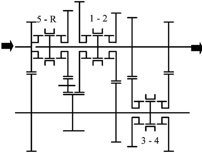
FIGURE 9.6. Scheme of an on-line double stage gearbox for a conventional lay-out.
