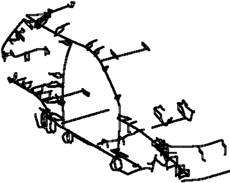
FIGURE 7.16. Final scheme of a beam model; the shape of the beams is determined by placing them below the styled exterior shape and assigning to them compatible cross sections, scaled from existing data bases.
