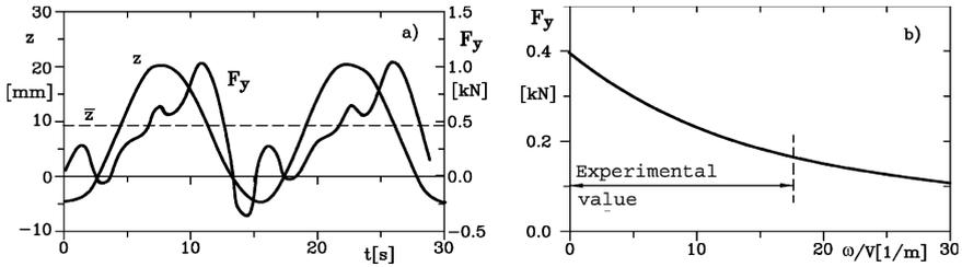
FIGURE 2.71. (a) Lateral force on a tire working with constant side slip angle, but with a rim moving vertically according to harmonic law  $z(t)$ . (b) Mean value of the force  $F_y$  as a function of the ratio between  $\omega$  (referred to  $z(t)$ ) and  $V$ .
