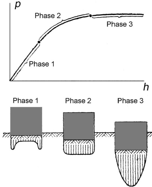
FIGURE 2.7. Main phases of deformation of an ideal homogeneous soil, expressed by sinking  $h$  as a function of applied pressure  $p$ . The lower diagrams show qualitatively the distribution of stress in the soil.
