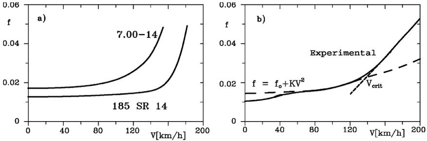
FIGURE 2.15. Diagram of rolling resistance  $f$  as a function of speed  $V$ . (a) Measured on a cross ply tire 175 14 and on a radial tire 185 R 14; (b) experimental curve (radial tire 135 R14, inflated at 190 kPa, with vertical load of 340 kN) compared with Eq. (2.13).
