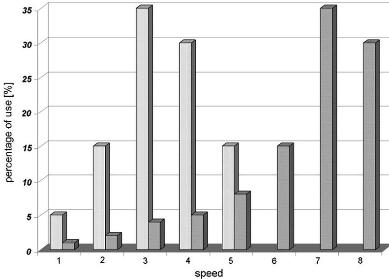
FIGURE 16.1. Qualitative diagram of different speeds, in the average life of a car (5 bars histogram) and of a medium duty industrial vehicle (8 bars histogram).
