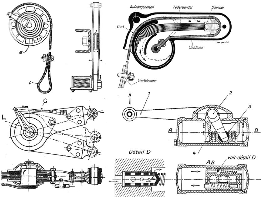
FIGURE 1.8. Some types of shock absorber, suitable for after market applications. The first three in the first row and the first in the second row work on mechanical friction; the last can also be adjusted. The fifth example refers to a hydraulic shock absorber.
