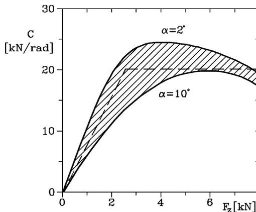
FIGURE 2.57. Cornering stiffness in function of load  $F_z$  (curve shown as  $\alpha = 10$  deg is a sort of “secant” stiffness).
