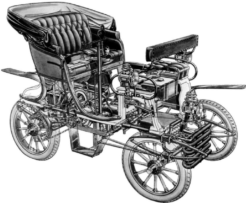
FIGURE 1.5. The Fiat  $3\frac{1}{2}$  HP of 1899 features a chain and sprocket transmission, where the sprocket is set in the center of curvature of the path of motion of the rear axle. Notice the Jeantaud steering system.
