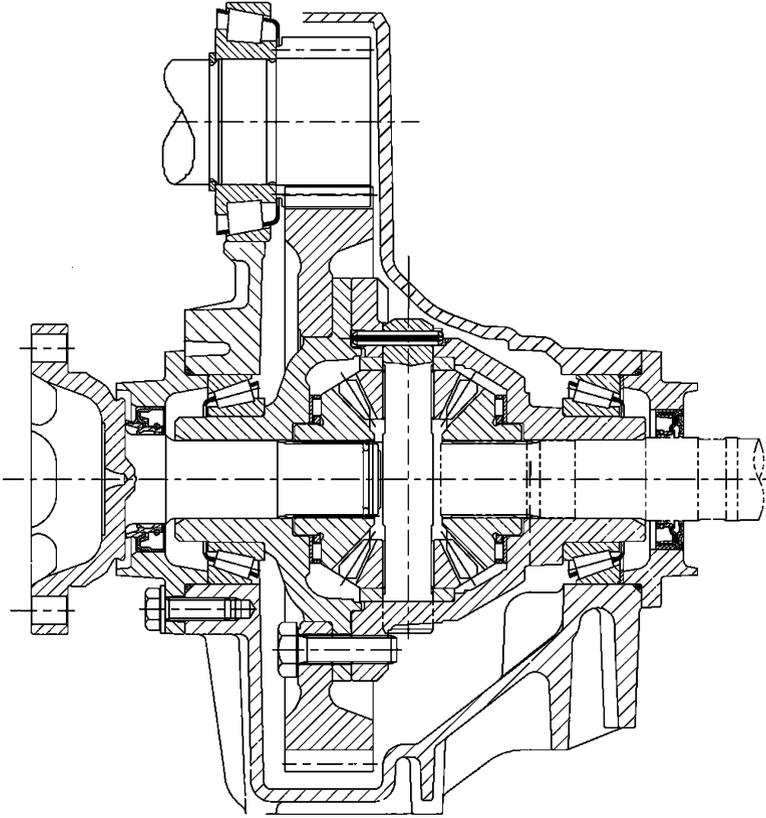
FIGURE 13.2. Differential and final drive for a front wheel driven car with transversal engine (FIAT).
