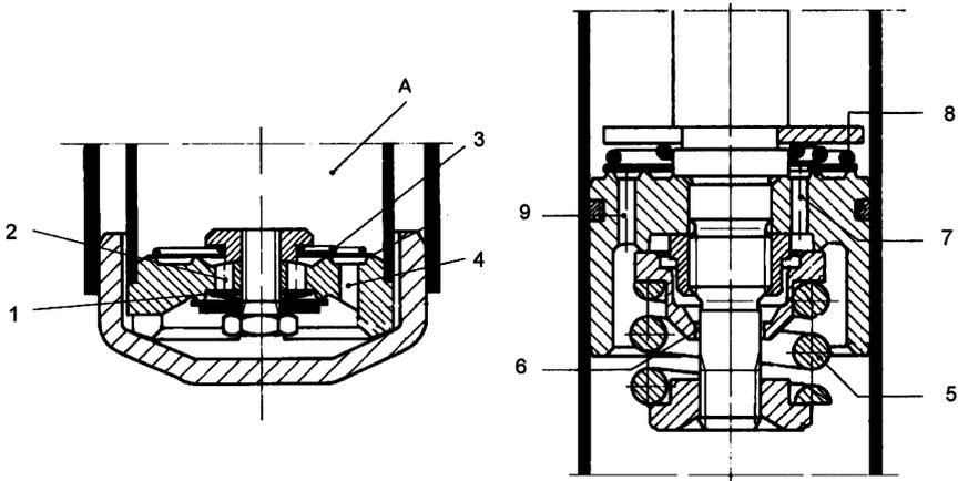
FIGURE 3.32. Valve assemblies of a double tube shock absorber.
