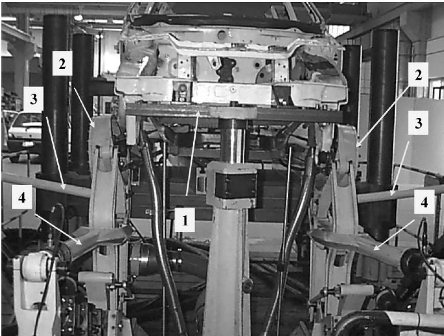
FIGURE 3.85. Three axial bench: the suspensions are mounted on a body, fixed to the bench with the structure 1. Suspensions are tested by actuators that can transfer to the wheel longitudinal, vertical and cornering forces.
