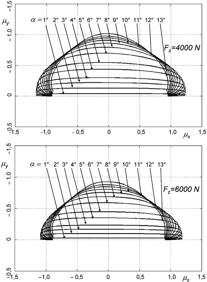
FIGURE 2.65. Ellipses calculated with modified Pacejka formulae for the same 195/65 R 15, tire, used to calculate carpet plots previously shown.
