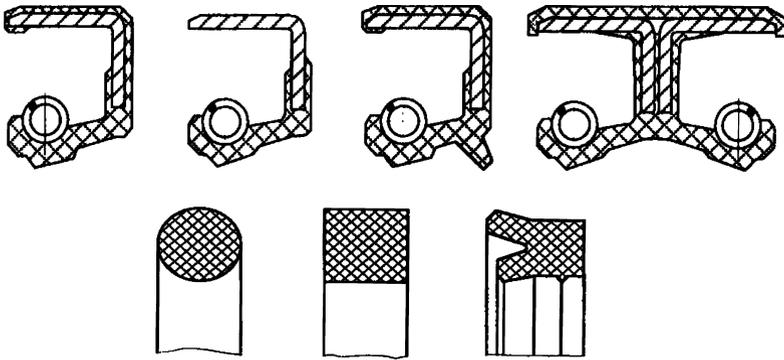
FIGURE 16.11. Examples of rotary seals (top) and sliding seals (bottom).
