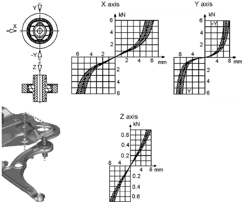
FIGURE 3.20. The stiffness of the more flexible bushing is very different in the  $x$  and  $y$  directions; for this purpose the rubber interior is designed as a beam, being bent in one direction and compressed in the other, in order to produce an asymmetric stiffness.
