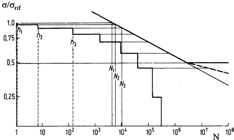
FIGURE 16.6. Comparison of a Wöhler (bilogarithmic representation) curve with an assigned load profile (staircase line). Stress is divided by a reference value;  $N_1$ ,  $N_2$ ,  $N_3$  represent the cycle number during which relative loads  $h_1$ ,  $h_2$ ,  $h_3$  are applied.
