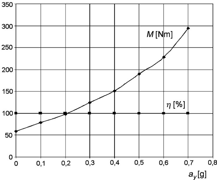
FIGURE 13.15. Diagram of driving wheel torque  $M$ , for a rear wheel driven car, on a 200 m radius steering-pad, as a function of centrifugal acceleration  $a_y$ , assuming an ideal differential mechanical efficiency  $\eta$  of 100%.
