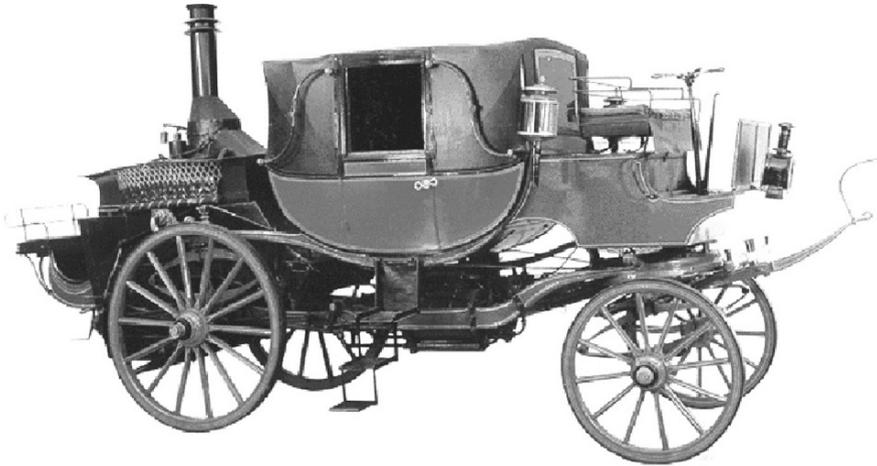
FIGURE 1.2. The Bordino's steam coach was built in 1854. The suspension system is strictly derived from that of a horse carriage. The rear axle is shaped as a crankshaft, where the connecting rods of the two cylinders operate directly (Automobile museum of Turin).
