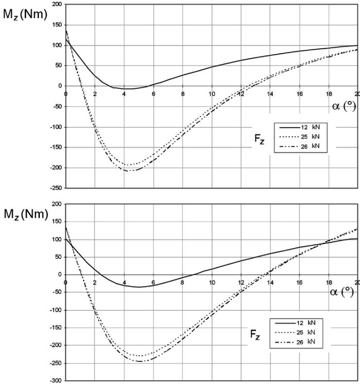
FIGURE 2.53. Carpet diagram of self aligning torque as function of sideslip angle for the same industrial vehicle tires 315/80 R 22,5 of previous figure.
