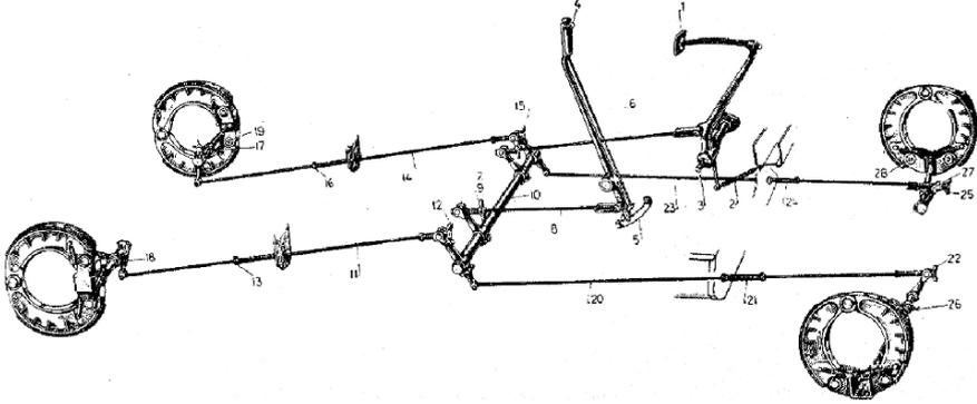
FIGURE 1.37. Mechanical control for a four wheels braking system; the articulation points between levers and tie rods had to stay on the center of instantaneous rotation of the axles during the suspension stroke, located near the fixed eyes of the leaf springs.
