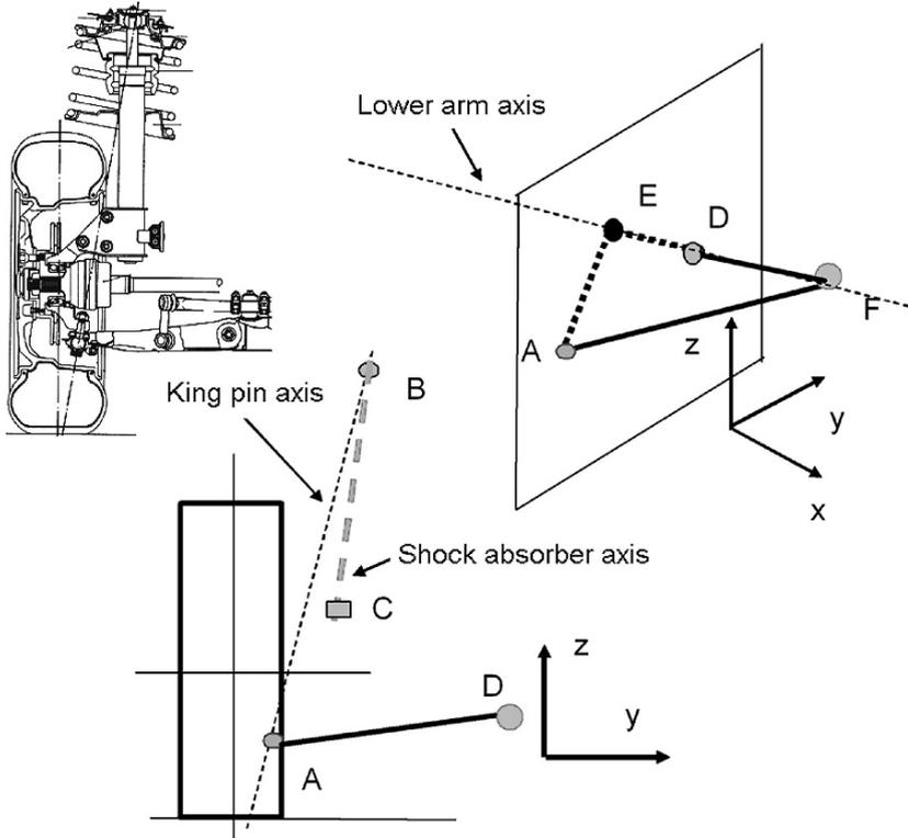
FIGURE 3.70. The arm rotation axis EF is determined to obtain the desired camber recovery, once A and B are determined.
