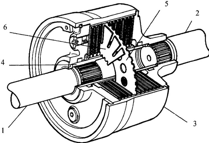
FIGURE 13.14. Scheme of a Ferguson joint. The friction between the two shafts 2 and 3 is made by the viscosity of the silicon oil inside the joint, working on discs 5 and 6; the friction torque depends on the relative speed between 2 and 3.
