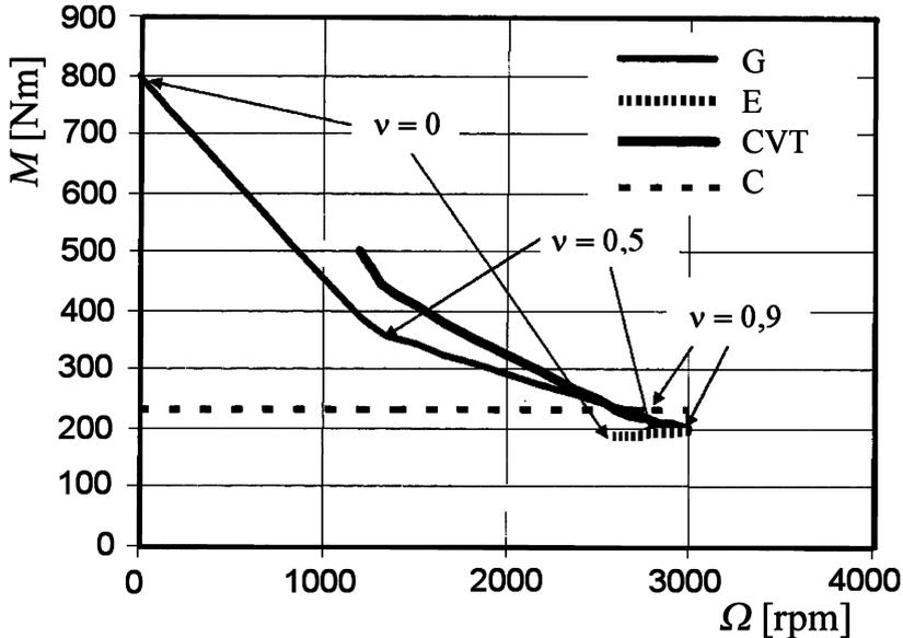
FIGURE 11.21. Calculation of the gearbox input torque  $M_2$  (G) starting from the engine torque  $M_1$  (E). The values of the speed transmission ratio of the different curves are shown. The values of  $M_2$  are also reported for an ideal continuously variable transmission (CVT) and for a slipping friction clutch (C).
