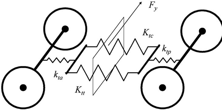
FIGURE 7.12. Elementary scheme for modelling the torsional deformation of a vehicle:  $k_{ta}$  and  $k_{tp}$  represent the torsional stiffness of the two axle suspensions, while  $K_{tc}$  and  $K_{tt}$  represent torsional stiffness of body and chassis frame in a hypothetical vehicle with separated frame.
