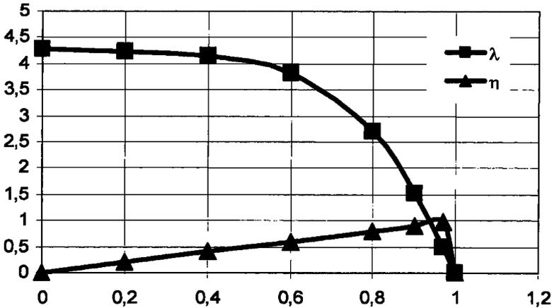
FIGURE 11.17. Characteristic curves of a hydraulic clutch representing  $\lambda$  and  $\eta$  as a function of  $\nu$ .  $\lambda$  is multiplied by 10,000.
