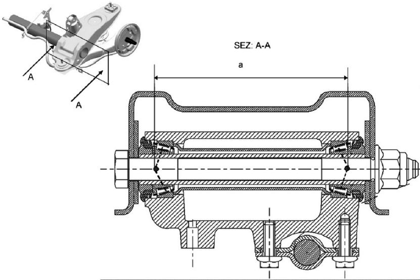
FIGURE 3.41. Detail of tapered roll bearings of the arm of the trailing arm suspension of the previous figure; one of the fixation points of the floating anti-roll bar can also be seen.
