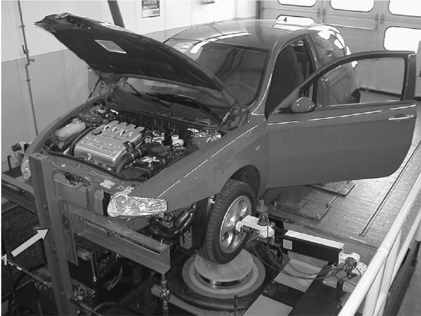
FIGURE 3.84. Elasto-kinematic bench with hydraulic actuators and anthropomorphic arm measuring system. The anthropomorphic arm detects the spatial wheel motion, consequent to force application or suspension stroke.
