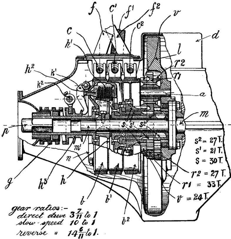
FIGURE 8.17. Epicycloidal gears gearbox of Ford model T of 1908. One reverse, one reduced forward speed and a direct drive are available.
