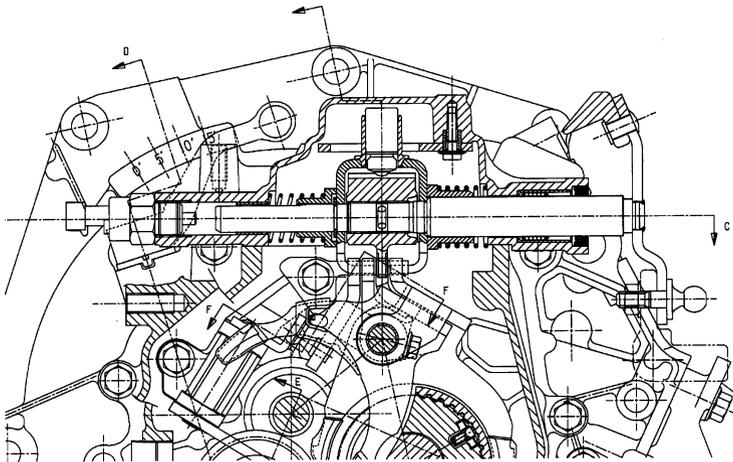
FIGURE 10.5. Cross section of a transversal gearbox; the forks of first and second speeds and of third and fourth speeds can slide on the bar of the fork of the fifth speed (FIAT).
