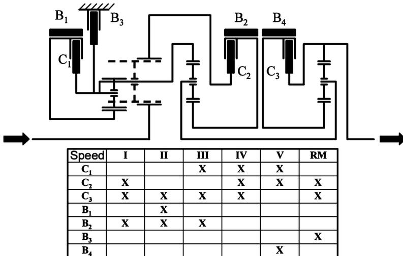
FIGURE 15.15. Scheme of an automatic powershift gearbox featuring three epicycloidal gear trains; five different speeds are obtained (Mercedes).
