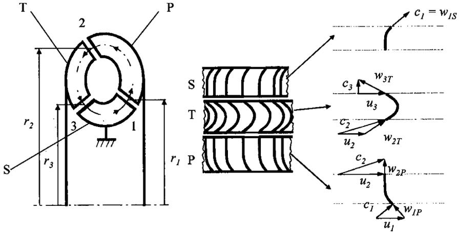
FIGURE 11.16. Speed triangles in a torque converter.
