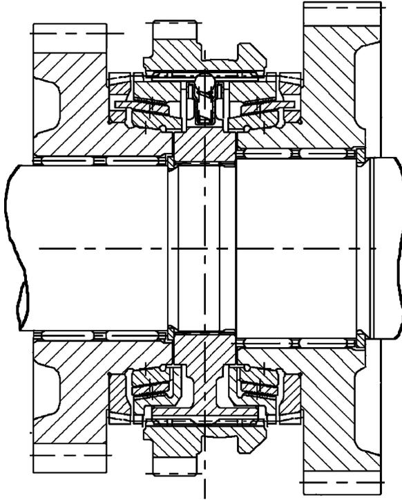
FIGURE 12.3. Cross section of a triple cone synchronizer (FIAT).
