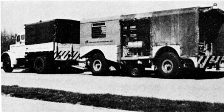
FIGURE 2.74. Vehicle for on road tire testing used by the vehicle research laboratory of the University of Delft. The test wheel is in the middle of the trailer.
