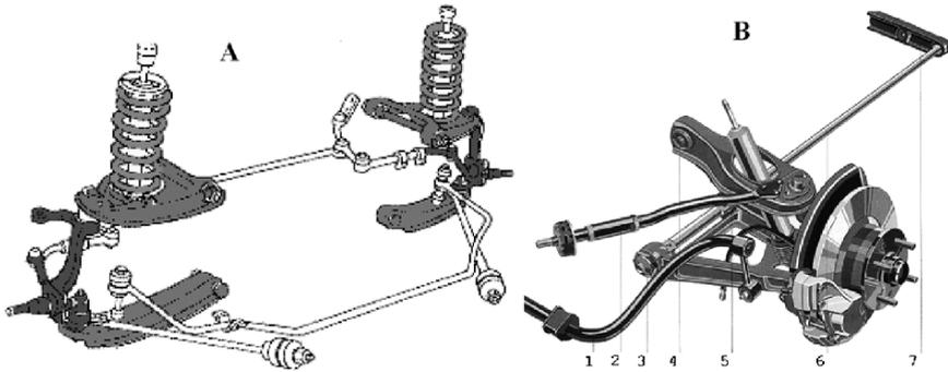
FIGURE 3.37. Different alternative positions for the coil spring and the shock absorber for a low double wishbone suspension.
