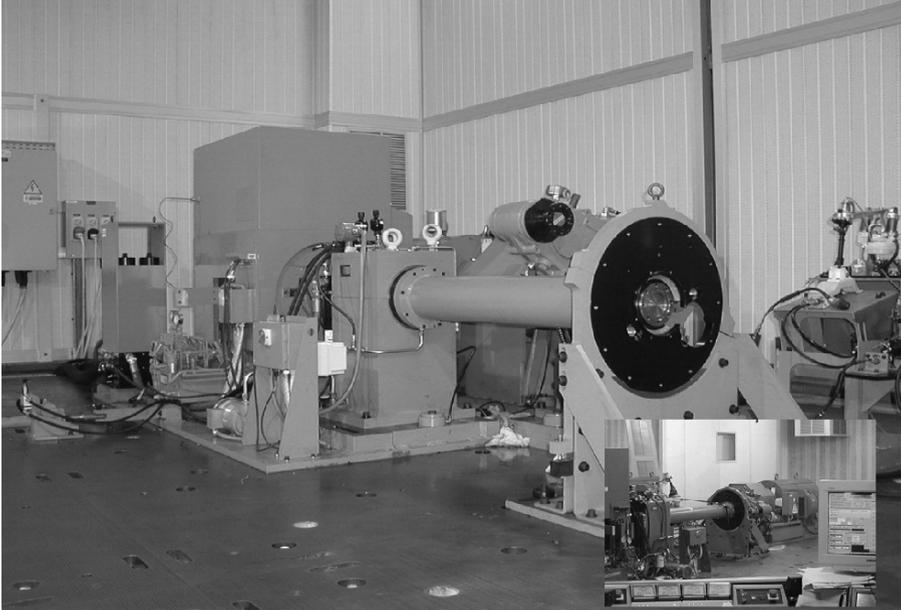
FIGURE 16.13. Interior of a typical modern test cell for complete transmissions. This kind of test cell can be adapted to all kind of tests, including acoustic emission measurement. It is acoustically reverberant, but can be changed to an anechoic cell, by encapsulating the transmission only in a suitable cabin.
