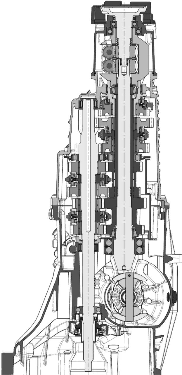
FIGURE 13.9. Gearbox, differential and transfer box of a permanent all wheel drive with longitudinal front engine (Audi). The gearbox output shaft is hollow, in order to install the front wheel axle drive shaft.
