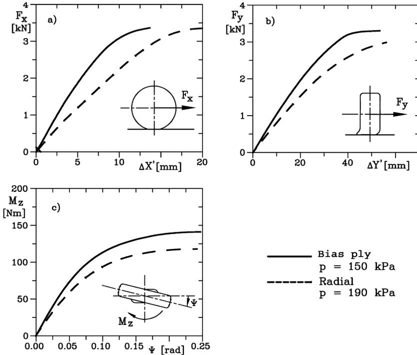
FIGURE 2.29. Forces in the  $X'$  and  $Y'$  directions and moments about the  $Z'$  axis versus deflections  $\Delta X'$  and  $\Delta Y'$  and rotation about the  $Z'$  axis for a radial and a bias-ply tire at standstill (wheel non-rolling) and in static conditions (load applied and removed slowly).
