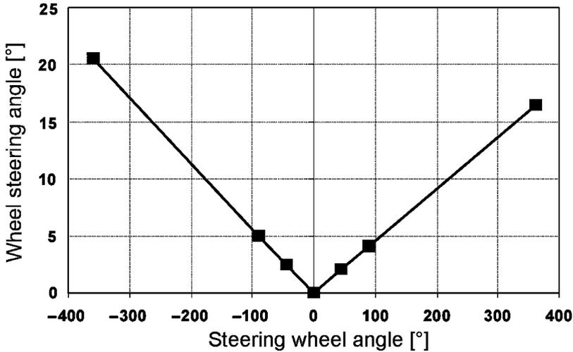
FIGURE 4.7. Diagram of wheel steering angle as a function of steering wheel angle; at the right the left wheel steering angle, at the left the right wheel steering angle.
