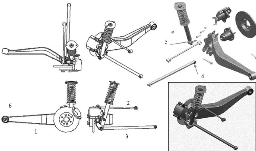
FIGURE 3.47. Scheme for a guided trailing arm suspension; the articulation point 6 must allow two rotational degrees of freedom to feature the desired camber angle recovery.
