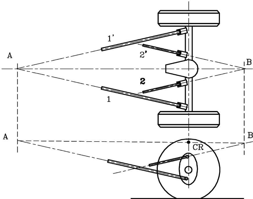
FIGURE 3.76. Four link suspension. Position of point CR.
