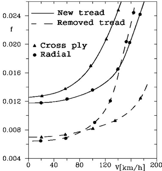
FIGURE 2.21. Effect of wear on  $f$ .
