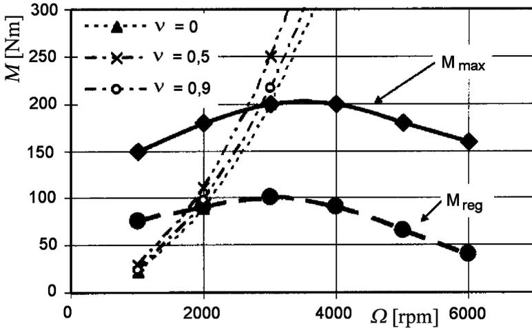
FIGURE 11.20. Matching torque curves of the engine and of a torque converter, at different values of the speed transmission ratio  $\nu$ . Notice that the operating speed is determined by the engine torque and the speed transmission ratio only.
