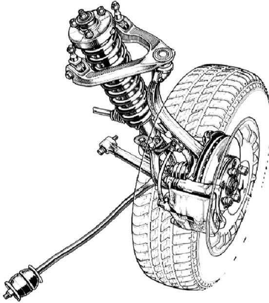
FIGURE 1.20. Honda front suspension with high double wishbone; high refers to the position of the upper arm compared to the conventional case.
