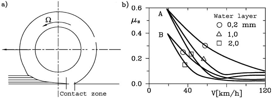
FIGURE 2.36. Hydrodynamic lift of a wheel (*aquaplaning*). (a) Scheme; (b) diagram of  $\mu_s$  as a function of speed on a wet road. Tire 145 - 15 with tread (curve A) and without (curve B);  $F_z = 3$  kN;  $p = 150$  kPa.
