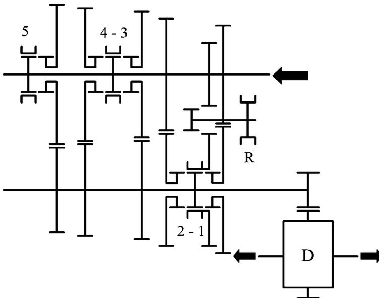
FIGURE 9.5. Scheme for a five speed single stage transmission, suitable for front wheel drive with transversal engine.
