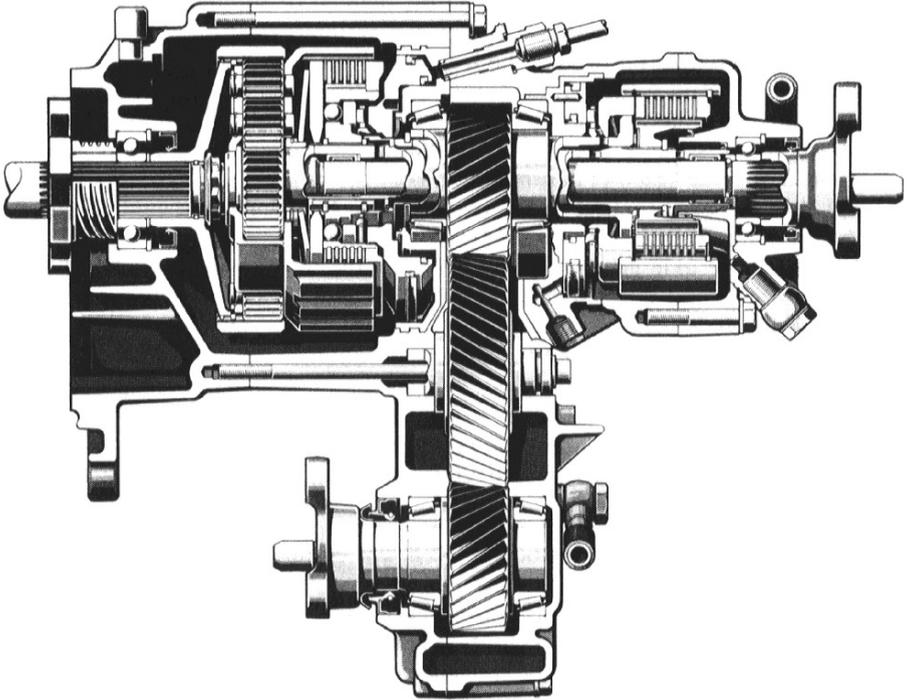
FIGURE 13.7. Transfer box for an all wheel drive on-road vehicle with longitudinal front engine (Mercedes). The box integrates the axle drive with an epicyclic differential with slip control.
