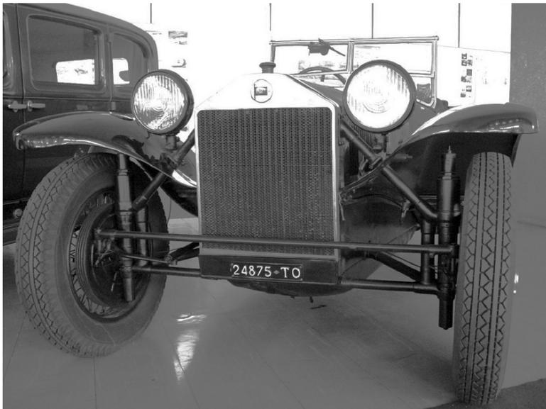
FIGURE 1.13. The front view of the Lancia Lambda shows the front suspension and the gate structure of connection to the body (Automobile Museum of Turin).
