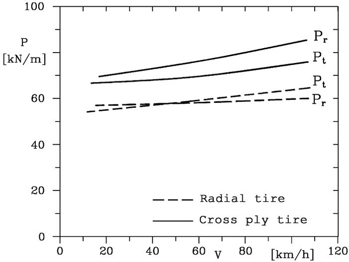
FIGURE 2.66. Dynamic stiffness in vertical  $P_r$  and lateral  $P_t$  direction of two 155 15 tires of radial and cross ply type, in function of speed.
