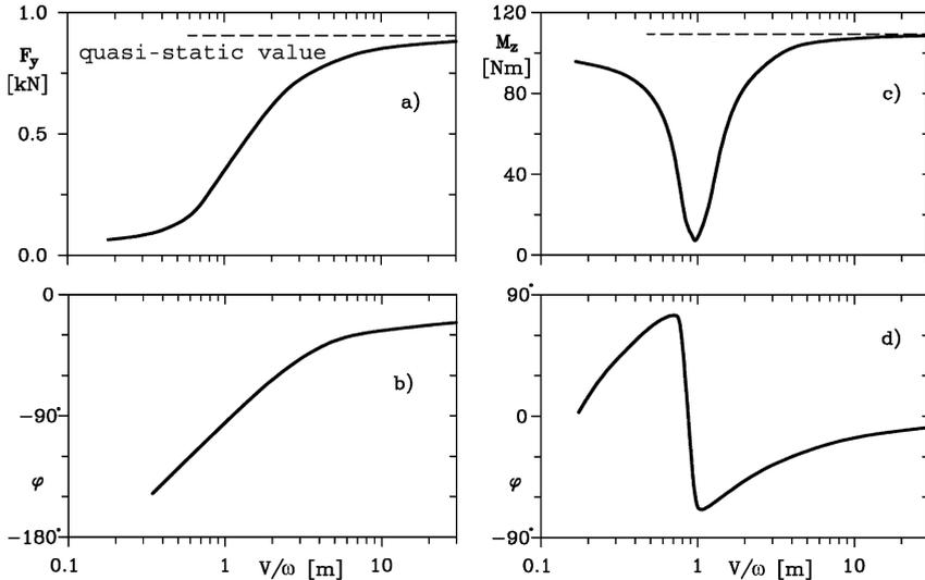
FIGURE 2.70. Lateral force and self aligning torque on a tire whose sideslip angle is changing according to harmonic law, between  $-4$  deg and  $4$  deg, as a function of the ratio  $V/\omega$  between speed and frequency of the low  $\alpha(t)$ , the wave length. Peak value (a), (c) and phase difference (b), (d) of force and moment are reported. Tire 190 14,  $F_z = 4.8$  kN,  $p = 165$  kPa.
