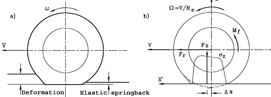
FIGURE 2.14. (a) Rolling tire on a deformable surface: ground deformation and spring back. (b) Forces  $F_z$  ed  $F_r$  and contact pressure  $\sigma_z$  in a rolling tire.
