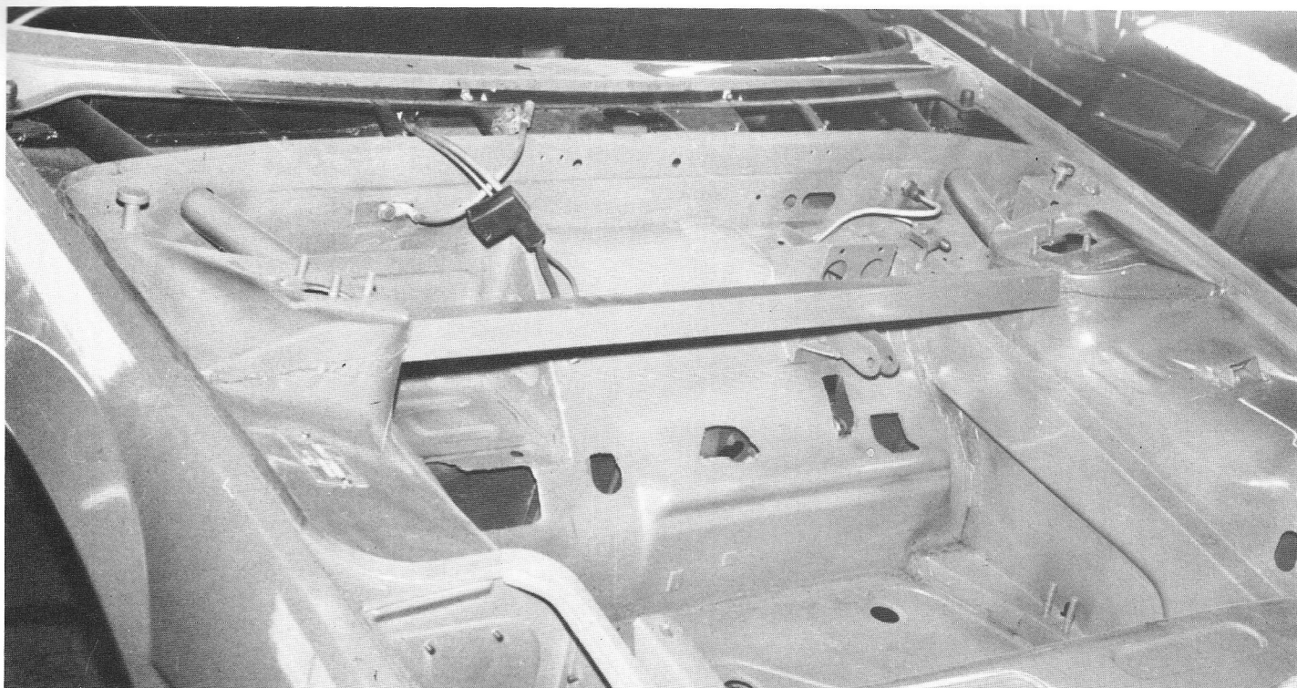
Cut-Outs For Steering Rack Clearance and Access
