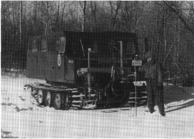
Fig. 2.34 A vehicle-mounted beavometer in field operation.
