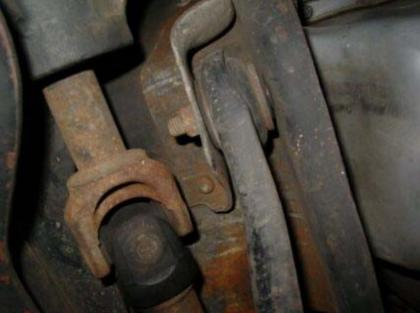
Now we can move on to the other sources of frame and suspension noises. Rivets  $\dots$  These things aren't a big problem in areas with little to no road salt, but they do rust or break. If you do find any broken, rusted or damaged, replace them with grade 8 bolts, nuts and lock washers.
