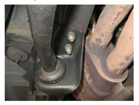
Below you can see the pivot arm bushings I mentioned. These bushings are what both the left and right sides of the twin I beam front suspension pivot on.
