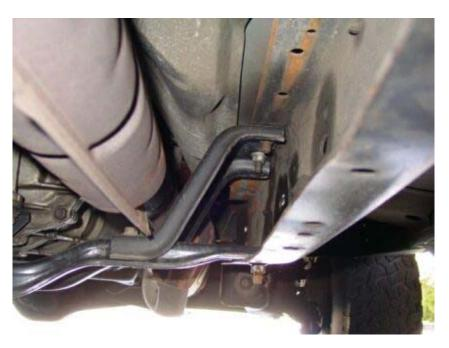
The first step is loosening all the bolts. Loosen the transmission to crossmember bolts, and all the bolts on the crossmember and gussets.
