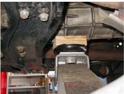
This next step may seem odd, but what you are doing is relieving any stress on the frame. This has to be done on a firm level surface such as a garage floor. Transmission in neutral, parking brake off, Start the engine and turn the steering wheel from center to full left, then full right and repeat. Return the steering wheel to straight when you are finished. Shut engine off, Apply parking brake.
