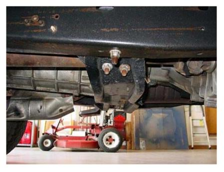
Now once all the bolts are loose, use a jack to raise the transmission up off the crossmember. The next step is to make sure the crossmember and gussets are free and not binding. You can use a small pry bar or flat tip screwdriver to make sure all the parts are loose.
