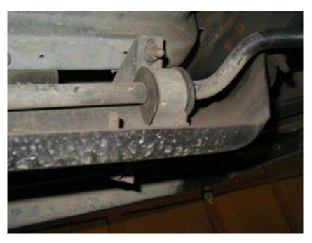
The next problem area below may be hard to see. Where the bolts that attach the steering box to the frame, cracks can appear in this area of the frame or the bolts can become loose.
