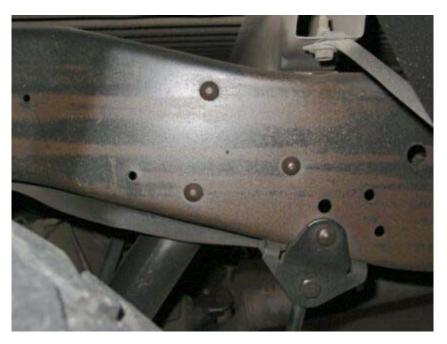
Body mounts, especially the front shown below, can deteriorate over time and cause noises. If you see any of these that look cracked replace them. They not only cause noise but they can cause the body of your truck to sag.
