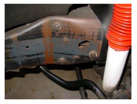
Finally, inspect the rear suspension area. There are a lot of bushings on the rear sway bar and shocks to have a look at. The trailing arm link bushings are of special interest simply because of their exposure to the elements.
