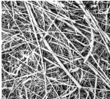
Fig. 6.1. Scanning electron micrograph of glass micro-fibre mat [5].
