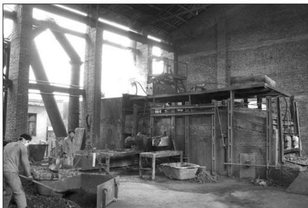
Fig. 15.2. Coal-fired reverberatory furnace processing battery scrap in China still in operation today.
