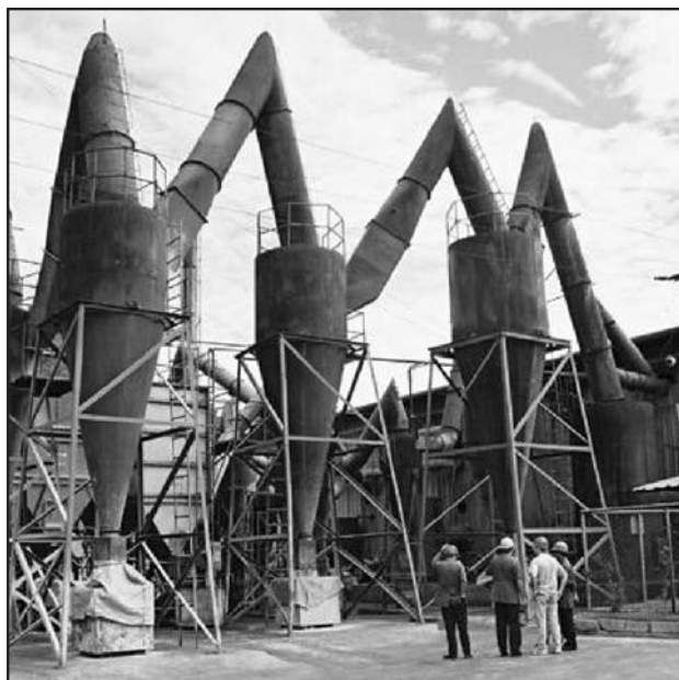
Fig. 16.11. Cyclones in series at the Baterias de El Salvador plant in San Salvador. (By courtesy of Baterias de El Salvador S.A.) [26].
