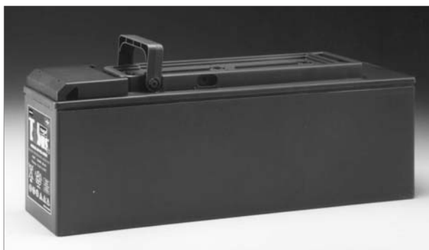
Fig. 13.14. 12-V, 100-Ah AGM battery (Marathon-type) with front terminals for telecommunications applications.
