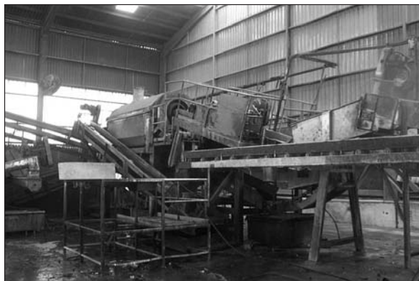
Fig. 15.1. Typical battery-breaker from Battery Recycling Industries. Conveyor belt in foreground is for small VRLA batteries that bypass the trommel, which is in the background.
