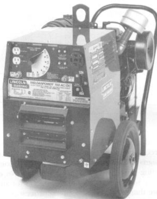
FIGURE 1-1 SMAW machines are relatively inexpensive and very popular for home workshops.
