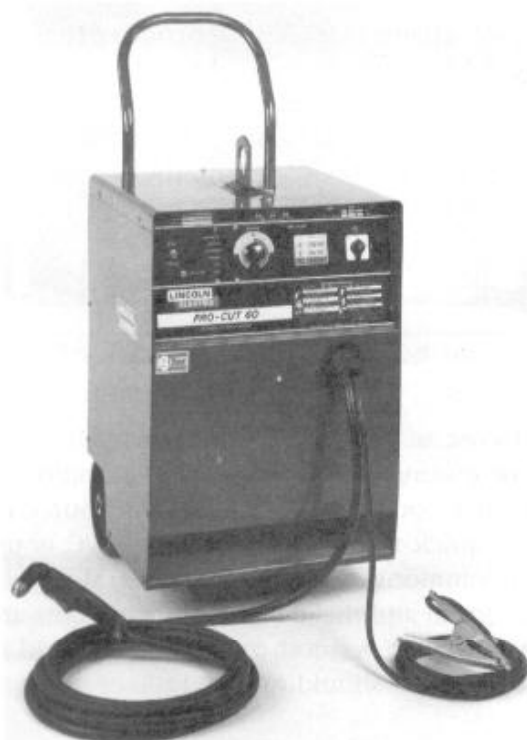
FIGURE 1-4 Any material that is electrically conductive can be cut using the plasma arc cutting process.
