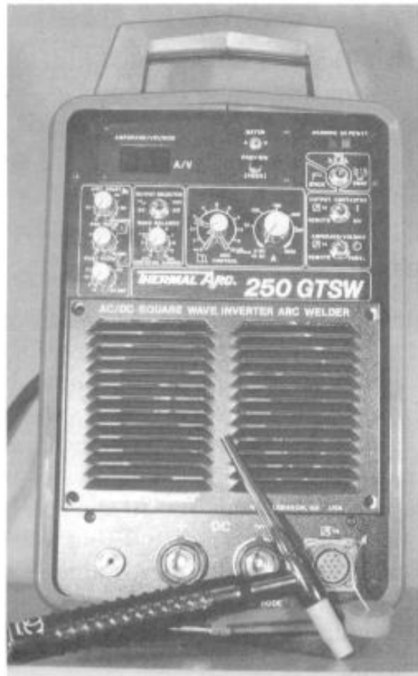
FIGURE 1-2 The GTAW machines date back to the 1930s. They are ideal for welding aluminum, magnesium, stainless steel, and carbon steel.
