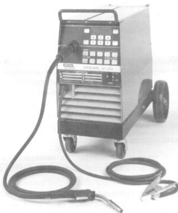
FIGURE 1-3 The GMA welding process utilizes a solid metal wire and requires the use of a shielding gas to protect the weld pool from the atmosphere.
