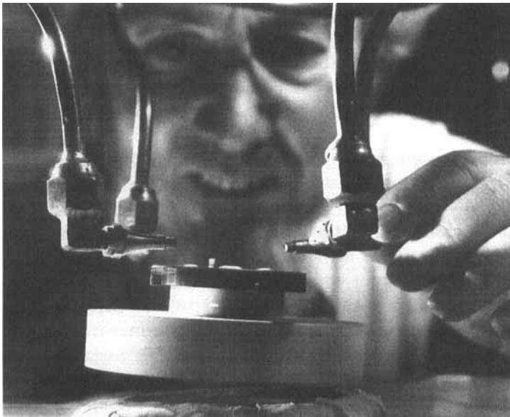
Figure 6-3 Photo of a spinning 0.8 kg rotor supported by YBCO magnetic bearing (Cornell University).
