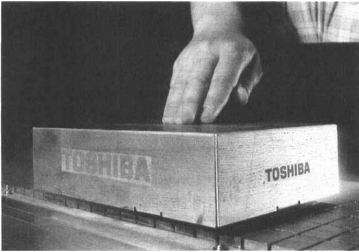
Figure 6-10 Linear magnetic bearing using high- T_c superconductor. [From Azukizawa et al. (1992), with permission; Toshiba Ltd., Japan.]
