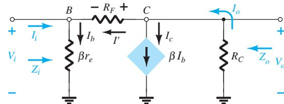
**FIG. 5.46**Substituting the  $r_e$  equivalent circuit into the ac equivalent network of Fig. 5.45. **$Z_i$**
