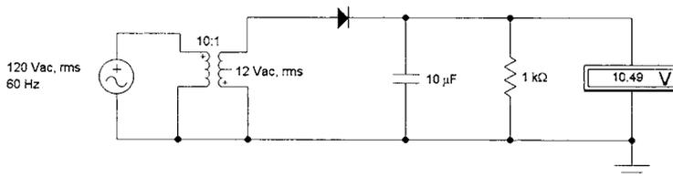
FIG. 15.33 DC supply with transformer input.
