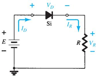
FIG. 2.8 Series diode configuration.
