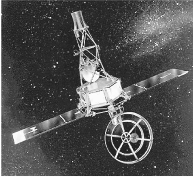
Figure 1. Mariner 2, launched in 1962, became the first spacecraft to fly by another planet, studying the Venusian atmosphere and surface. During its 3\frac{1}{2} -month journey to Earth's neighbor, the craft made the first-ever measurements of the solar wind, a constant stream of charged particles flowing outward from the Sun. It also measured interplanetary dust, which turned out to be scarcer than predicted. In addition, Mariner 2 detected high-energy charged particles coming from the Sun, including several solar flares, as well as cosmic rays from outside the solar system. As it flew by Venus on 14 December 1962, Mariner 2 scanned the planet with infrared and microwave radiometers, revealing that Venus has cool clouds and an extremely hot surface. Mariner 2's signal was tracked until 3 January 1963. The spacecraft remains in orbit around the Sun.
