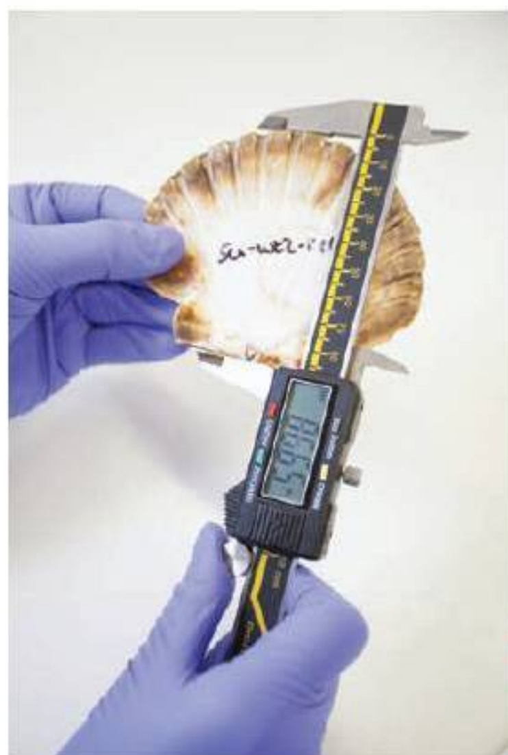
Figure 15.1 Digital callipers being used to measure shells.
