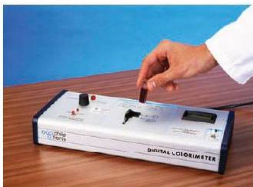
Figure 15.3 (a) A colorimeter measures optical density and (b) a potometer measures the volume of water taken up by a leafy plant shoot.
