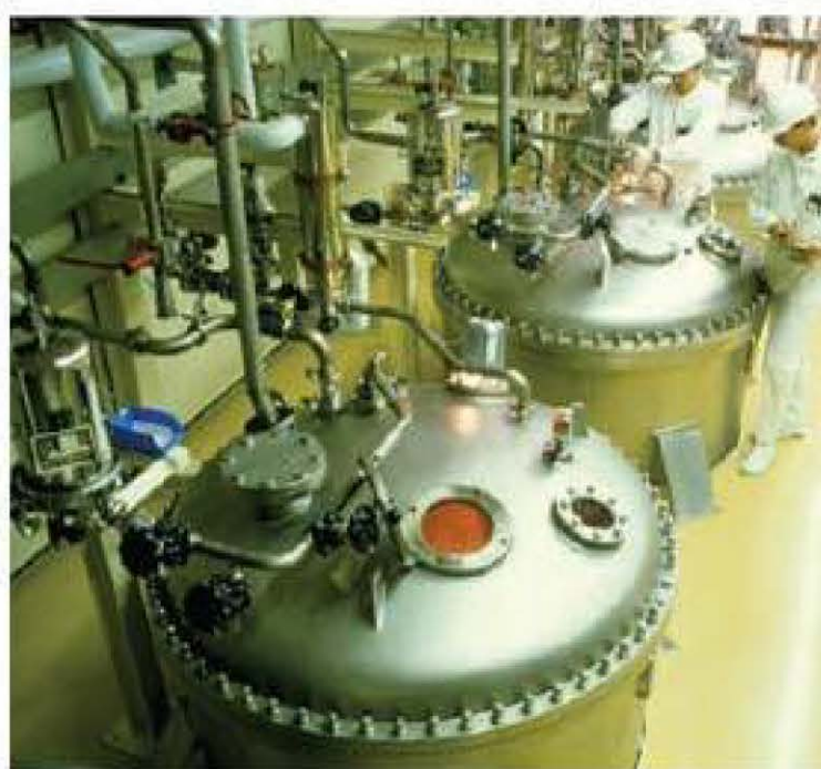
Figure 11.14 These large industrial fermenters contain a culture of transgenic bacteria that produce a human protein. Since the bacteria secrete the human protein, it is relatively simple to extract it from the culture medium.
