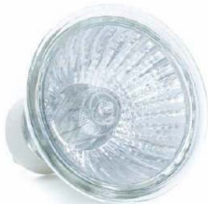
Figure 10.11 A halogen bulb, contains a halogen such as iodine or bromine. As tungsten evaporates from the filament, it usually condenses on the inner surface of the bulb. The halogen combines with this tungsten deposit on the glass to produce tungsten halides, which evaporate easily. When the tungsten halide reaches the filament, the intense heat of the filament causes the halide to break down, releasing tungsten back to the filament. This process, known as the halogen cycle, extends the life of the filament and keeps the inner surface of the bulb clean, which lets halogen bulbs stay close to full brightness as they age.
