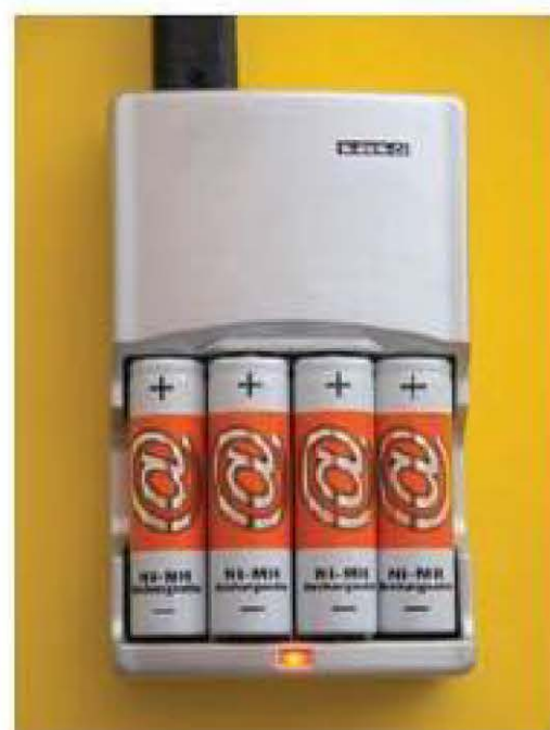
Figure 6.3 These batteries can be recharged as the reaction that releases the electrical energy is reversible. Plugging the batteries into the mains via the charger converts electrical energy back into chemical energy, stored in the batteries.
