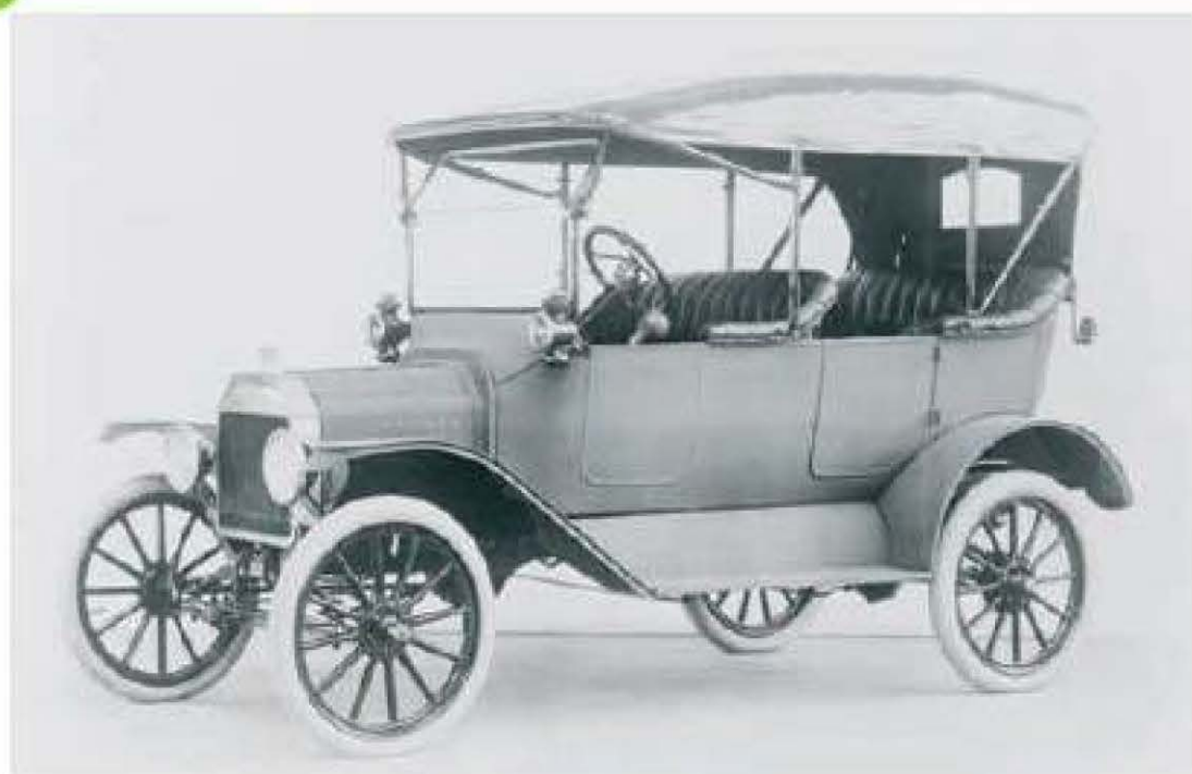
Figure 4.19 Henry Ford came across a vanadium alloy in 1905 in a crash at a racing event. When Ford picked up a fragment, which was part of a valve spindle, he was surprised how strong it was. He decided his new Model-T car would be made from vanadium steel. Mass production began in 1913 and 15 million cars were made, all with vanadium steel components.
