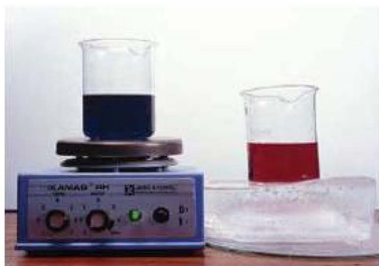
Figure 6.10 Cobalt chloride equilibrium. Experiment demonstrating the changes in equilibrium in cobalt chloride solutions that are heated (left) or cooled (right).
