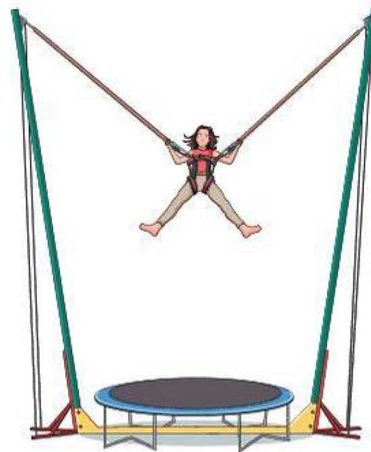
Figure 12.7 A bungee trampoline makes use of the elastic properties of ropes. When a tensile force is applied to the ropes, they stretch. The greater the force applied, the more they stretch.
