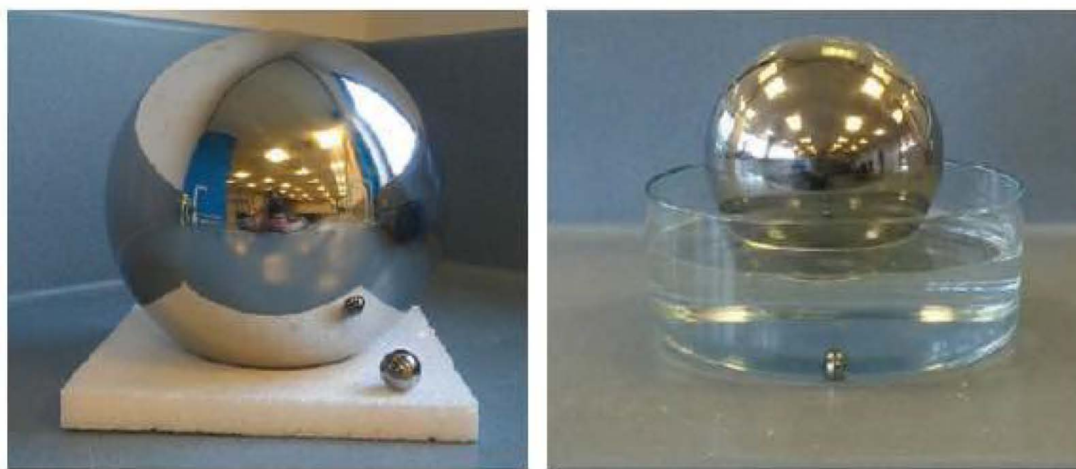
Figure 12.4 The large stainless steel globe is more massive than the small stainless steel ball bearing. The globe floats; the ball bearing doesn't. Why?
