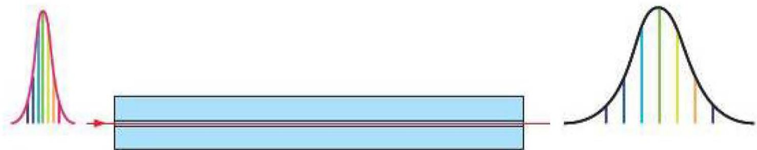
Figure 5.27 Material dispersion: different frequencies have a different refractive index.
