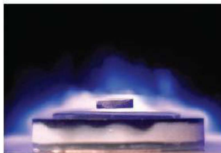
Figure 13.13 Magnetically levitating superconductor.
