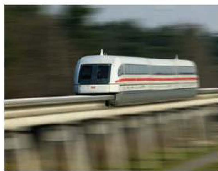
Figure 13.14 One of the Shanghai Maglev trains, where superconducting magnets support the train, enabling it to travel at speeds up to 270 mph (430 km/h).
