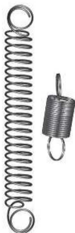
Figure 12.9 These two springs were the same length. One of them has gone beyond its elastic limit and will not return to its original length.
