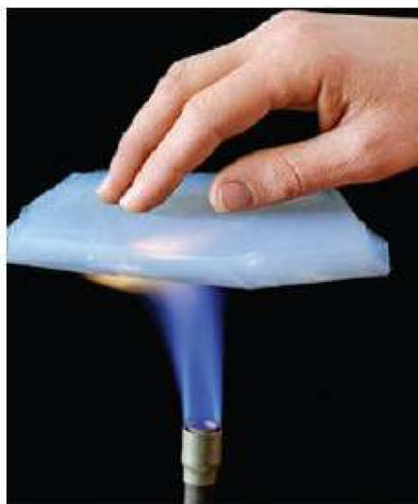
Figure 12.5 Aerogel: a very low-density material that is 99.8% air.
