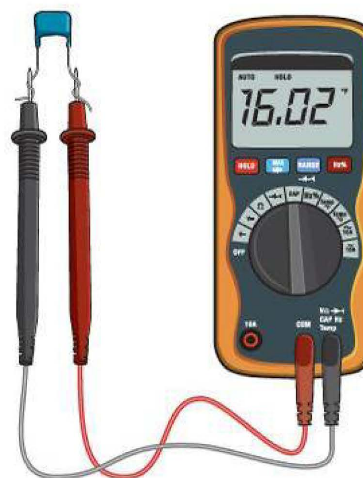
Figure 6.8 Digital multimeter measuring capacitance.
