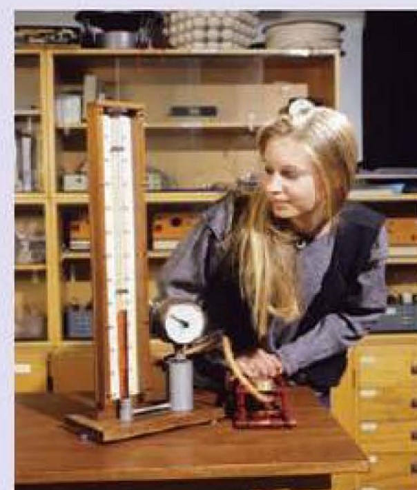
Figure 4.12 Apparatus used to investigate Boyle's law.
