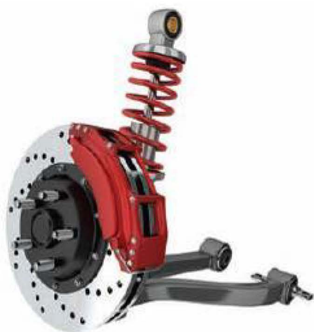
Figure 2.27 The spring and the piston-cylinder on a shock absorber form the suspension system for a wheel in a car.
