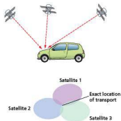
Figure 7.2 Calculation of position using satellites
