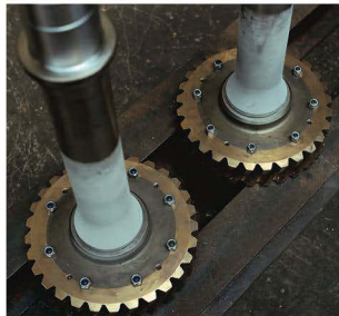
Figure 19.1 'Shrink-fitting' of axles into gear wheels
