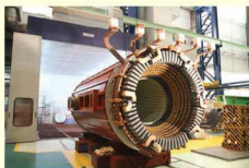
b Stator (induction coils)
