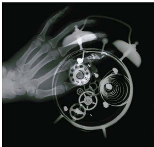
Figure 32.7 X-rays cannot penetrate bone and metal.
