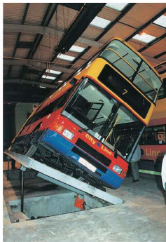
Figure 11.6b A double-decker bus being tilted to test its stability
