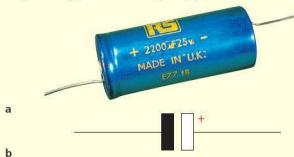
Figure 39.4a Electrolytic capacitor; b symbol showing polarity
