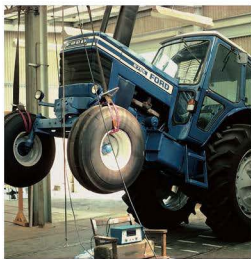
Figure 11.6a A tractor under test to find its centre of mass
