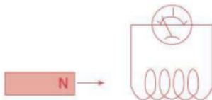
An e.m.f. is induced in the coil and current flows in the circuit making the coil act like a magnet. What will be the polarity of the end of the coil nearest the magnet when the N pole of the magnet:
