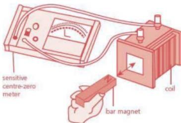
The meter needle swings to the left when the magnet is moving towards the coil. State how the needle behaves when the bar magnet:
