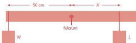
Find the distance  $X$  for the beam to be balanced when:
