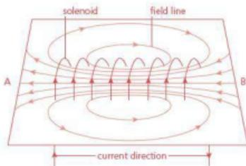
a A solenoid, like a bar magnet, has a N and a S pole.
