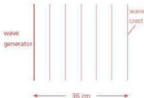
The distance occupied by 6 waves is 36 cm. The frequency of the wave generator is 5 Hz.
