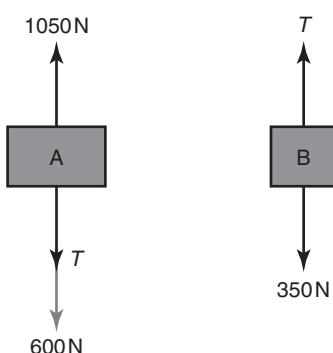
**(ii)**  $60a = 1050 - 600 - T$ ;  $35a = T - 350$ **(iii)**  $a = 1.05 \text{ ms}^{-2}$ ;  $T = 386.84 \text{ N}$ **9 (i)**  $a = 0.625 \text{ ms}^{-2}$ ;  $T = 93.75 \text{ N}$ **(ii)**  $15.81 \text{ ms}^{-1}$ **(iii)** 557.5 N
