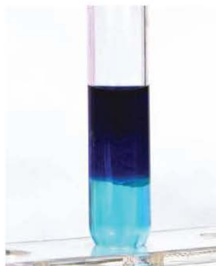
Figure 18.2.9 The result of adding butylamine to a solution of copper ions. The hydrated copper(II) ions give the light blue colour, while the dark blue colour is due to the formation of a complex between the copper and the butylamine.
