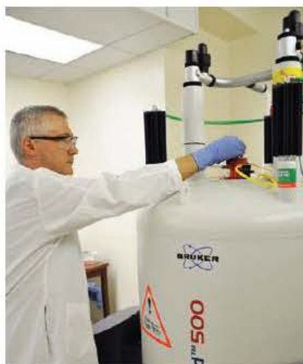
Figure 19.14 Researcher adding a sample to an NMR spectrometer.
