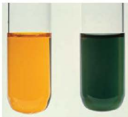
Figure 14.7 Another test for reducing agents. The test: add orange dichromate(VI) solution acidified with dilute sulfuric acid to the reducing agent. The result: the orange solution turns green as orange \text{Cr}_2\text{O}_7^{2-} ions are usually reduced to green \text{Cr}^{3+} ions but sometimes to blue \text{Cr}^{2+} ions.
