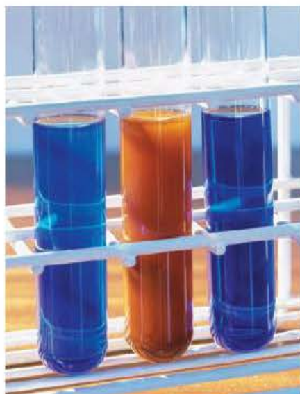
Figure 17.2.18 The test tube in the middle contains Fehling's reagent that has been reduced by an aldehyde to form an orange-brown precipitate of copper(I) oxide. The test tubes on the left and right contain Fehling's reagent and ketones.
