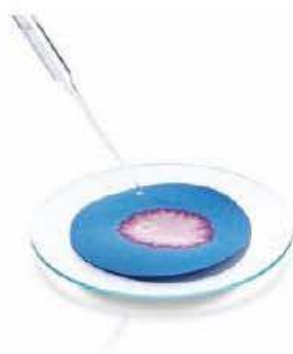
Figure 15.21 Filter paper soaked in pink cobalt(II) chloride solution and dried in an oven until it is blue, can be used to test for the presence of water.
