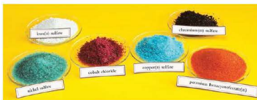
Figure 15.14 Crystals of co-ordination compounds. From left to right these are: \text{NiSO}_4 \cdot 7\text{H}_2\text{O} , \text{FeSO}_4 \cdot 7\text{H}_2\text{O} , \text{CoCl}_2 \cdot 6\text{H}_2\text{O} , \text{CuSO}_4 \cdot 5\text{H}_2\text{O} , \text{Cr}_2(\text{SO}_4)_3 \cdot 18\text{H}_2\text{O} and \text{K}_3[\text{Fe}(\text{CN})_6] .
