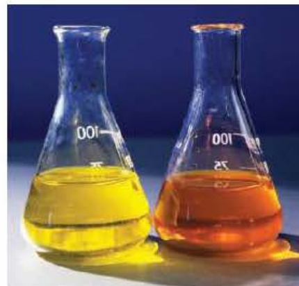
Figure 11.6 On the left, a yellow solution of chromate(vi) ions in water. On the right, the solution has turned orange as more dichromate(vi) ions form after adding a few drops of strong acid.
