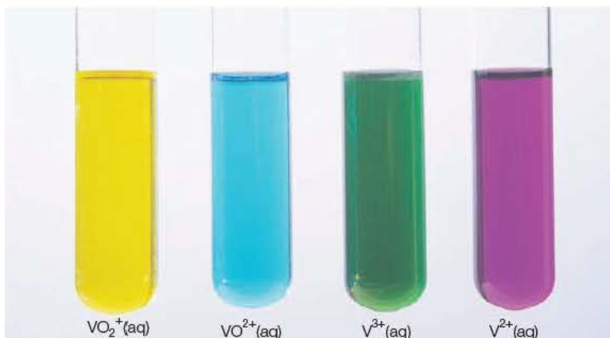
Figure 15.8 The oxidation states of vanadium showing the colours of its ions in the +5, +4, +3 and +2 oxidation states.
