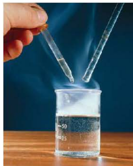
Figure 17.3.13 Ethanoyl chloride reacts vigorously with water, releasing hydrogen chloride. A smoke of ammonium chloride forms when an ammonia-soaked glass rod is held in these fumes.
