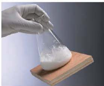
Figure 13.2.6 The endothermic reaction between the solids barium hydroxide and ammonium chloride cools the flask so much that the water between the flask and the wooden block freezes.
