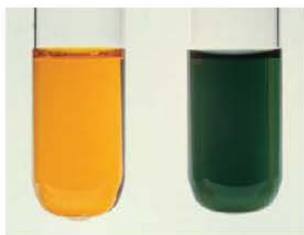
Figure 15.9 Solutions containing ions in two of the oxidation states of chromium. On the left, a solution of dichromate(vi) ions, \text{Cr}_2\text{O}_7^{2-} ; on the right, a solution of chromium(III) ions, \text{Cr}^{3+} .
