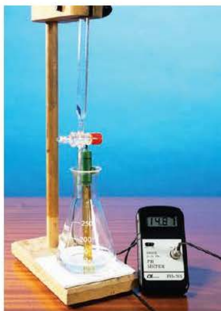
Figure 12.9 A pH meter can be used to measure the pH of the solution in the flask during an acid–base titration, and to detect the end-point.
