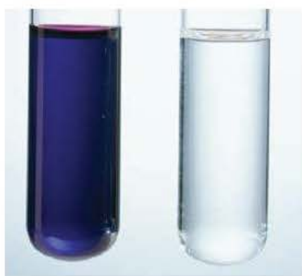
Figure 14.6 A test for reducing agents. The test: add a solution of purple potassium manganate(VII) acidified with dilute sulfuric acid to the reducing agent. The result: the purple solution turns colourless as purple \text{MnO}_4^- ions are reduced to very pale pink \text{Mn}^{2+} ions.
