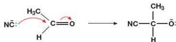
Figure 17.2.13 The first step of the nucleophilic addition of hydrogen cyanide to ethanal.
