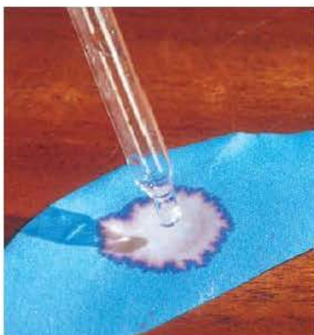
Figure 14.3 ▲ Using cobalt chloride paper to test for water
