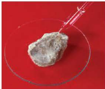
Figure 12.3 ▲ Geologists use dilute hydrochloric acid to test for carbonates in rocks
