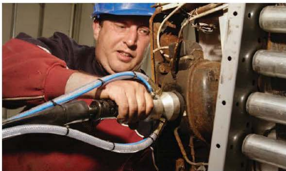
Figure 15.19 ◀ A recycling plant in South Wales which recovers CFCs from the coolant system of old refrigerators and freezers. The CFCs are removed from the canisters as gases, liquefied and then chemically destroyed.
