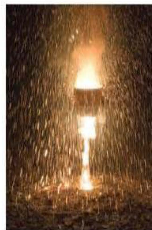
Thermite (exothermic) reaction creating molten iron
