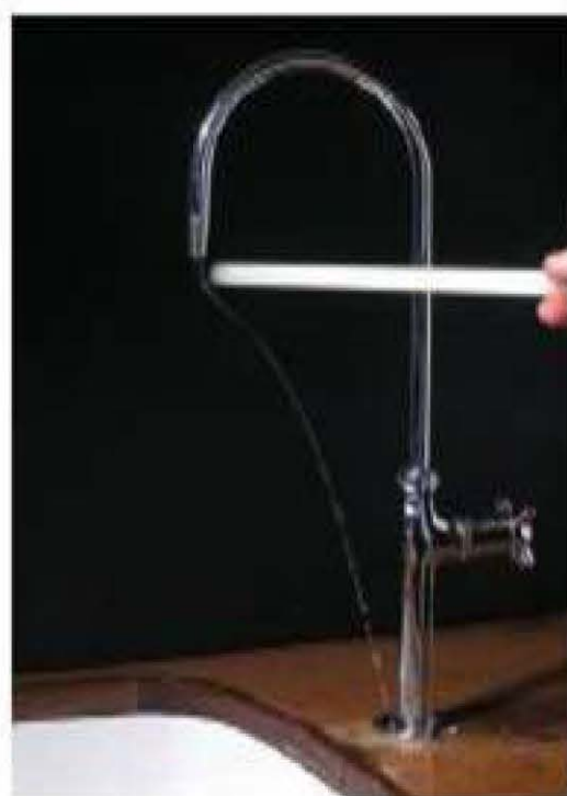
Stream of polar liquid deflected by a charged rod
