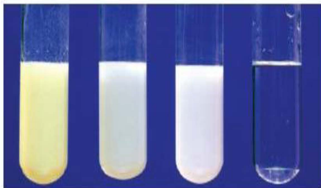
Silver halide precipitates. From left to right: silver iodide, silver bromide, silver chloride and a solution of silver fluoride
