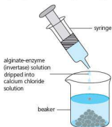
■ Figure 2.45 Laboratory demonstration of enzyme immobilization
