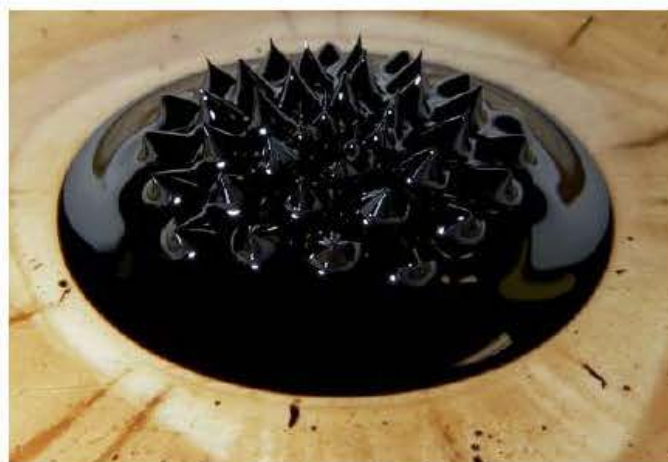
■ Figure 2.10 A ferrofluid is a suspension of iron particles in oil, giving a 'magnetic' fluid
