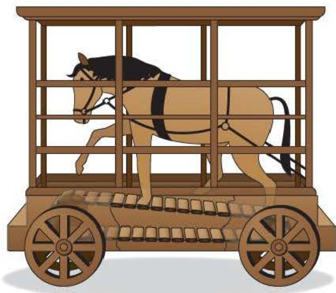
■ Figure 6.25 Early design for a horse-powered railway locomotive
