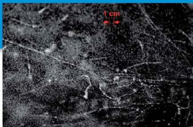
■ Figure 11.39 Photograph of ionization vapour trails inside a cloud chamber
