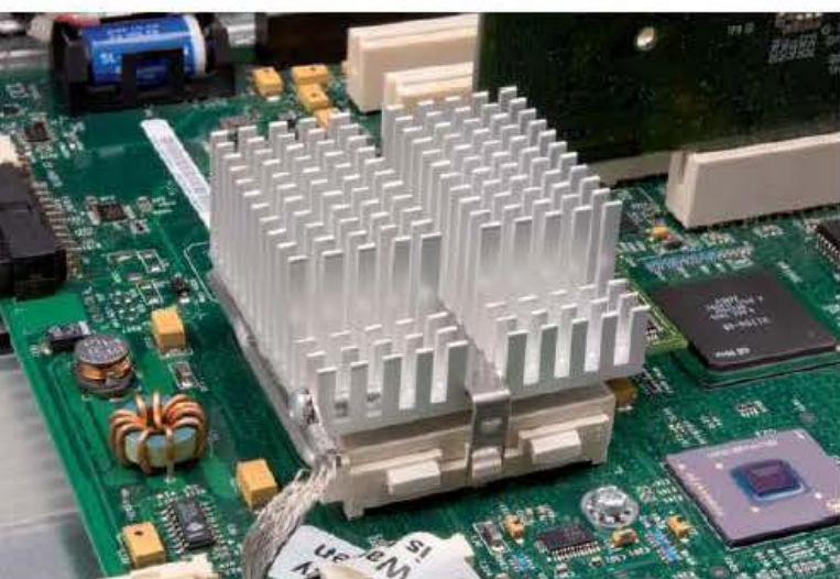
■ Figure 6.23 A heat sink is used to dissipate wasted energy as heat in a microprocessor
