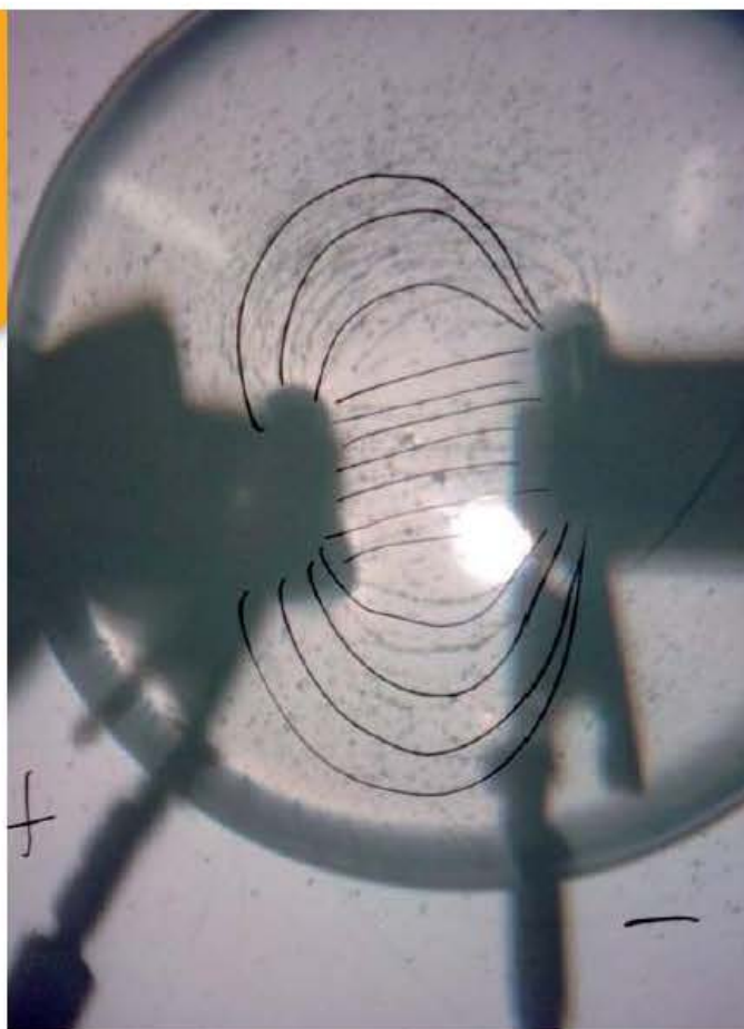
■ Figures 2.11 and 2.12 In these photos two copper plate 'electrodes' are being submersed in vegetable oil. The electrodes are then connected to a high-voltage supply of electricity, and black pepper is sprinkled into the oil. The pepper aligns itself with the electric field in the oil
