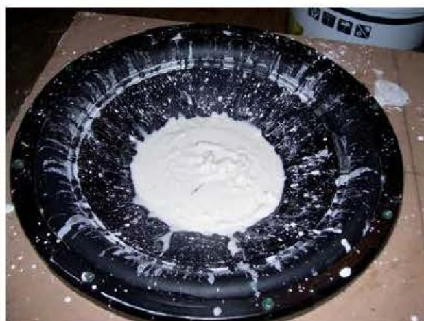
■ Figure 3.16 A bowl of corn starch on a loudspeaker. The sound waves cause the non-Newtonian fluid to go rigid
