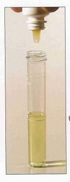
Continue adding drops of reagent until the sample turns a stable yellow color. Each drop added since the beginning of the test represents 1°dH.
