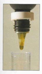
Above: Liquid test kits involve adding a specified number of drops of one or more reagents to a water sample. Hold the bottle vertically so that the drop sizes are equal and correctly measured. Compare the final color change to a printed chart.
