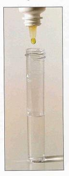
1 Add the KH reagent to a 5 ml sample of water and gently swirl the tube to mix it up. Count the numbers of reagent drops added.
