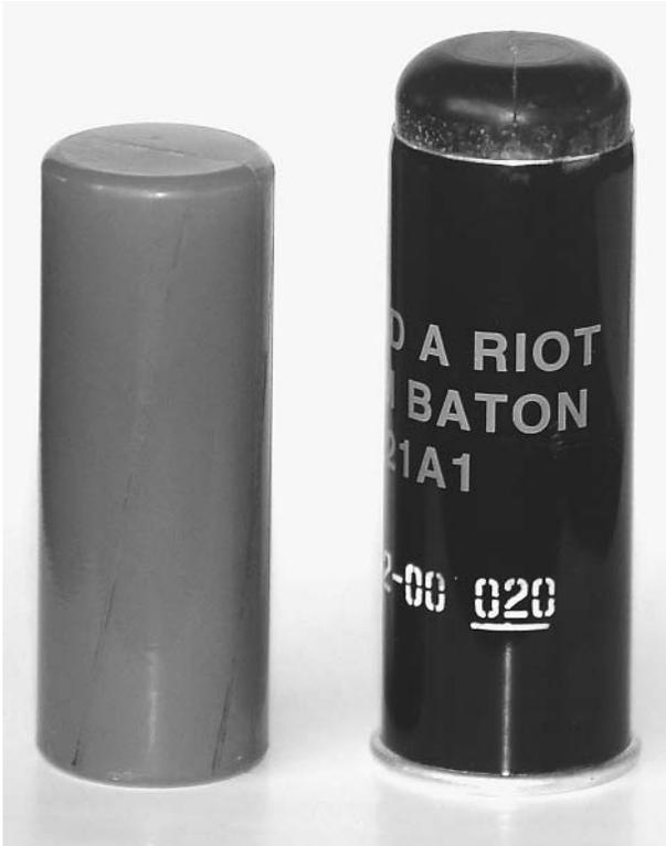
An old baton round, left, and one of the new baton rounds, right, also known as plastic bullets. The plastic bullets expand upon contact and release most of their destructive energy before penetrating vital organs.
