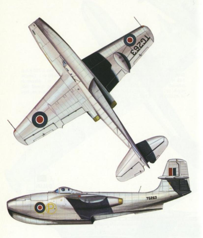
First prototype Saunders-Roe SR/A1, as modified in 1948. Engine: One 3,250 lb. (1,474 kg.). st Metropolitan-Vickers F.2/4 Beryl MVB 1 turbojet. Span: 46 ft. 0 in. (14·02 m.). Length: 50 ft. 0 in. (15·24 m.). Wing area: 415 sq. ft. (38·55 sq. m.). Normal take-off weight: 16,255 lb. (7,373 kg.). Maximum speed: 512 m.p.h. (824 km/hr.), achieved by third prototype with 3,850 lb. (1,746 kg.) st engine.
