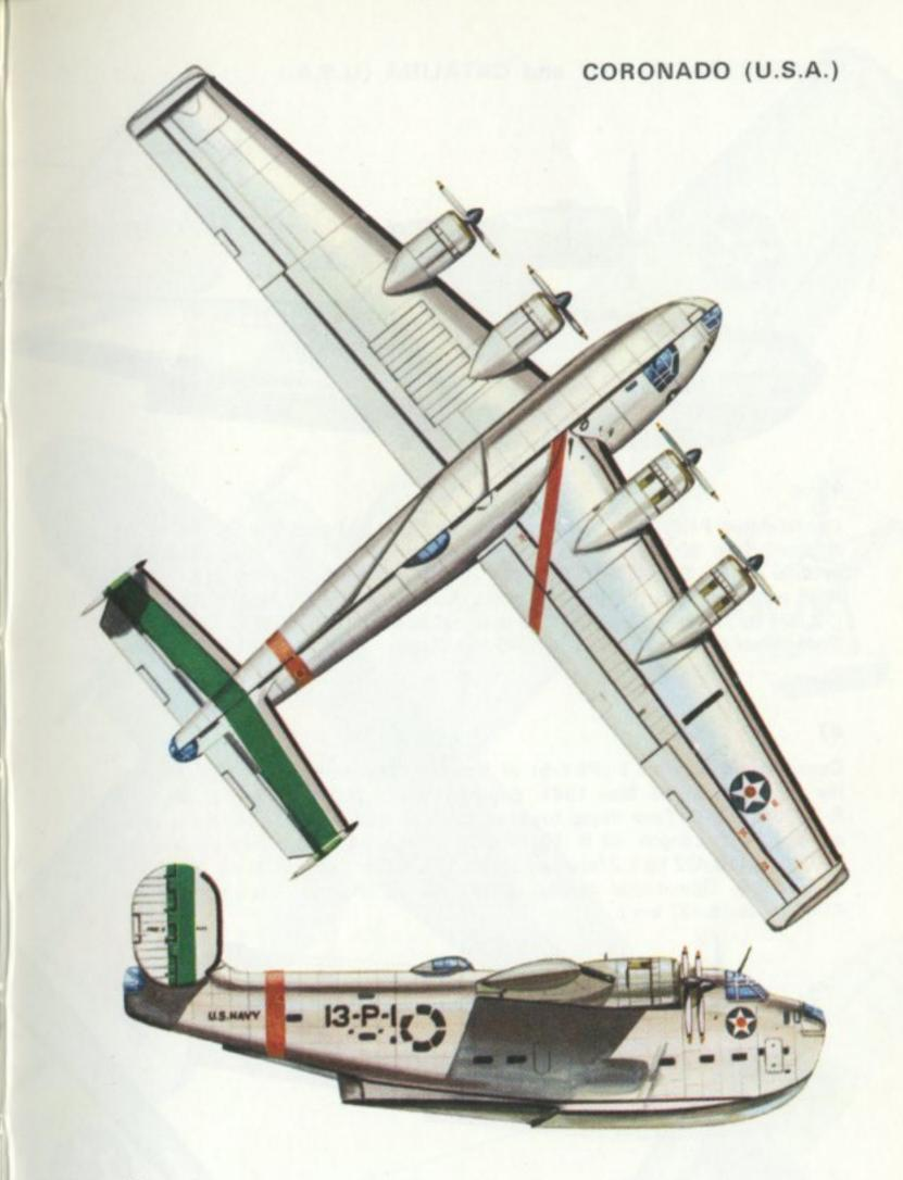
Consolidated PB2Y-2 Coronado of US Navy Squadron VP-13, early 1941. Engines: Four 1,200 h.p. Pratt & Whitney R-1830-78 Twin Wasp fourteen-cylinder radials. Span: 115 ft. 0 in. (35·05 m.). Length: 79 ft. 0 in. (24·08 m.). Wing area: 1,780 sq. m. (165·37 sq. m.). Normal take-off weight: 60,441 lb. (27,416 kg.). Maximum speed: 255 m.p.h. (410 km/hr) at 19,000 ft. (5,791 m.). Operational ceiling: 24,100 ft. (7,346 m.). Normal range: 3,705 miles (5,963 km.).
