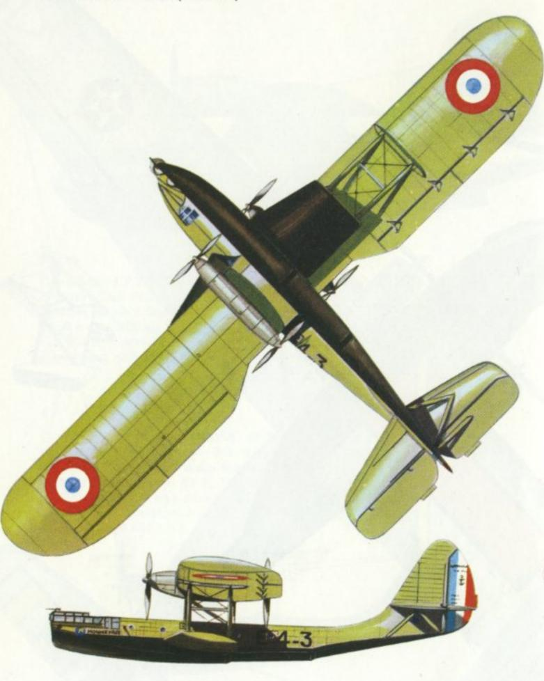
Latécoère 302 Mouneyres of Escadrille E4, French Navy, ca late 1939. Engines: Four 930 h.p. Hispano-Suiza 12 Ydrs twelve-cylinder Vee-type. Span: 144 ft.  $4\frac{1}{4}$  in. (44 m.). Length: 85 ft.  $9\frac{1}{2}$  in. (26·15 m.). Wing area: 2,755·6 sq. ft. (256 sq. m.). Take-off weight: 52,911 lb. (24,000 kg.). Maximum speed: 149 m.p.h. (240 km/hr.) at 6,560 ft. (2,000 m.). Operational ceiling: 16,400 ft. (5,000 m.). Maximum range: 2,050 miles (3,300 km.).
