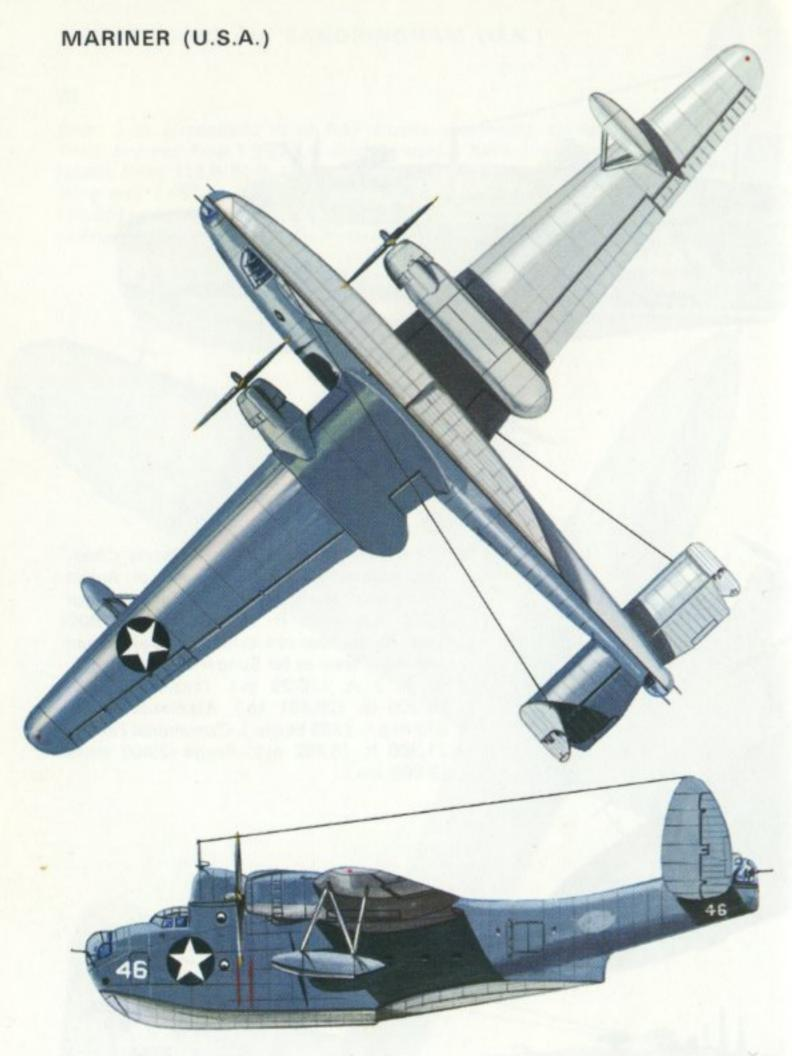
Martin PBM-3D Mariner of the US Navy, March 1944. Engines: Two 1,900 h.p. Wright R-2600-22 Cyclone fourteen-cylinder radials. Span: 118 ft. 0 in. (35·97 m.). Length: 79 ft. 10 in. (24·33 m.). Wing area: 1,408 sq. ft. (130·80 sq. m.). Normal take-off weight: 51,330 lb. (23,283 kg.). Maximum speed: 211 m.p.h. (340 km/hr.) at 16,100 ft. (4,907 m.). Operational ceiling: 19,800 ft. (6,035 m.). Range: 2,420 miles (3,895 km.).
