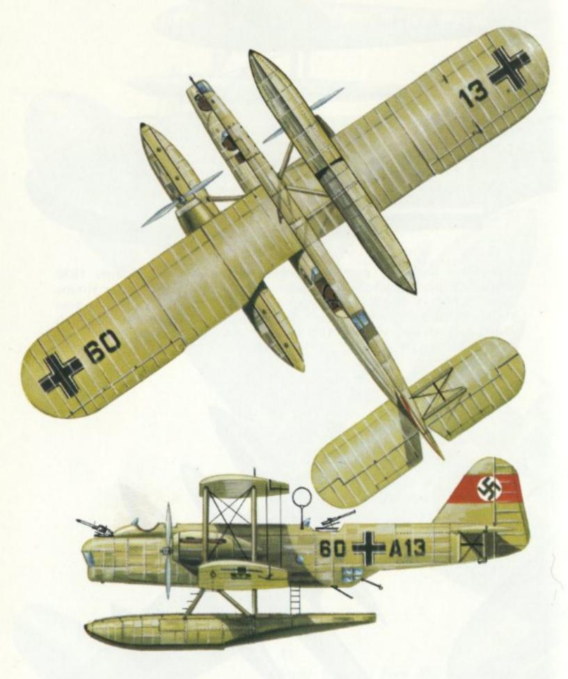
Heinkel He 59B-2 of the 1st Staffel, K.Fl.Gr. 106, Luftwaffe, ca 1937. Engines: Two 660 h.p. BMW VI 6·0 ZU twelve-cylinder Vee-type. Span: 77 ft. 9 in. (23·70 m.). Length: 57 ft. 1 in. (17·40 m.). Wing area: 1,649 sq. ft. (153·2 sq. m.). Take-off weight: 19,842 lb. (9,000 kg.). Maximum speed: 137 m.p.h. (220 km/hr.) at sea level. Operational ceiling: 11,480 ft. (3,500 m.). Maximum range: 1,085 miles (1,750 km.).
