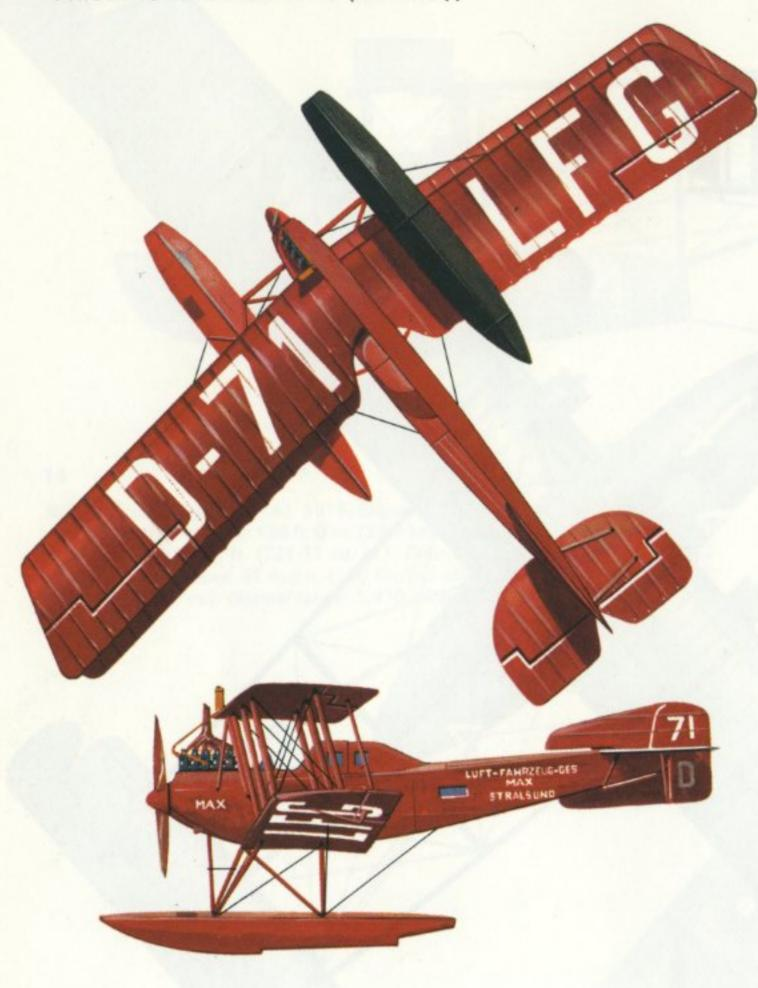
V1 Max (Friedrichshafen FF49) built and operated ca mid-1919 by Luft-Fahrzeug GmbH. Engine: One 200 h.p. Benz Bz IV six-cylinder in-line. Span: 56 ft. 3\frac{1}{4} in. (17.15 m.). Length: 38 ft. 2\frac{3}{4} in. (11.65 m.). Wing area: 766 sq. ft. (71.16 sq. m.). Take-off weight: 4,718 lb. (2,140 kg.). Maximum cruising speed: 84 m.p.h. (135 km/hr.). Endurance: approx 5 hr. 30 min.
