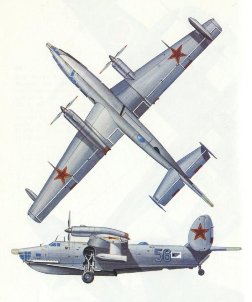
Beriev Be-12 of the Soviet naval air arm, ca 1968. Engines: Two 4,000 s.h.p. Ivchenko AI-20D turboprops. Span: 98 ft. 5 in. (30 m.). Length: 98 ft. 5 in. 30 m.). Wing area: 1,130·2 sq. ft. (105 sq. m.). Maximum take-off weight: 64,926 lb. (29,450 kg.). Maximum speed: 378 m.p.h. (608 km/hr.). Operational ceiling: 37,040 ft. (11,290 m.). Maximum range: 2,485 miles (4,000 km.). All data estimated.
