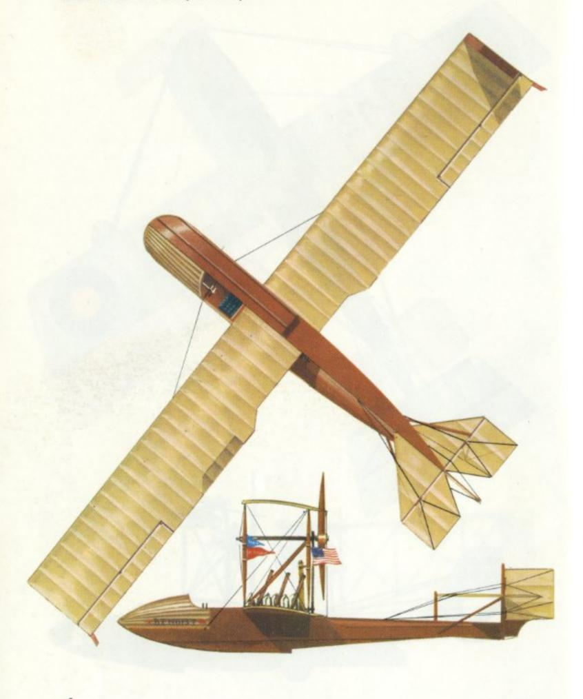
Benoist flying boat used for Tampa-St Petersburg service, early 1914. Engine: One 75 h.p. Roberts six-cylinder in-line. Span: 45 ft. 0 in. (13·72 m.). Length: 26 ft. 0 in. (7·92 m.). Wing area: approx 416 sq. ft. (38·65 sq. m.). Empty weight: 1,190 lb. (540 kg.). Speed: 64 m.p.h. (103 km/hr.).
