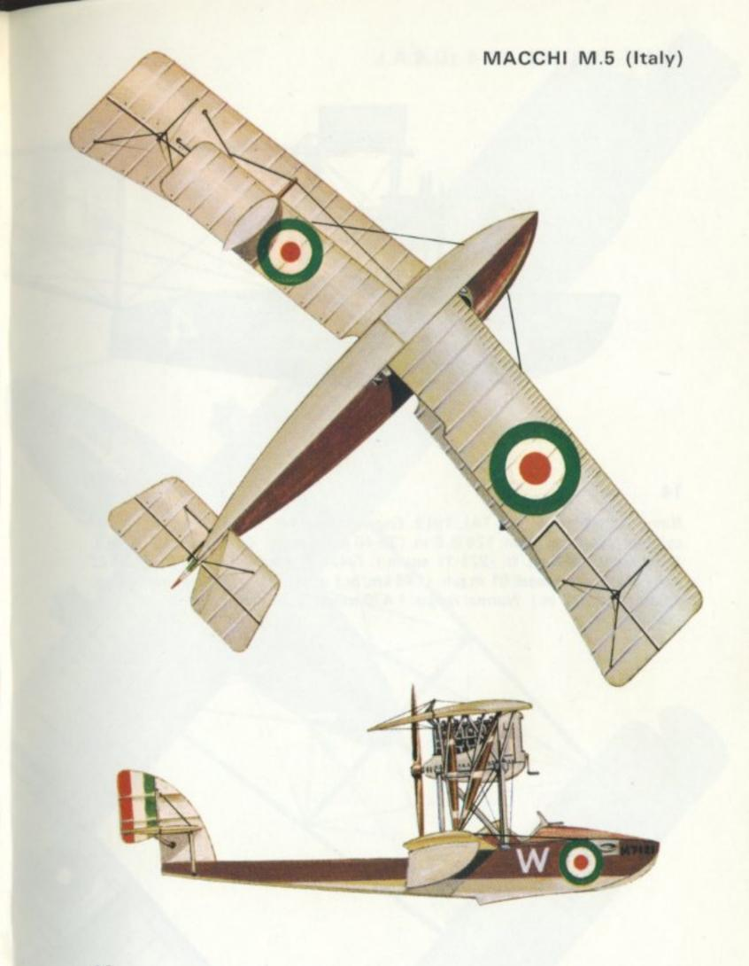
Macchi M.5 of the Regia Marina Italiana, ca 1918/19. Engine: One 160 h.p. Isotta-Fraschini V-4B twelve-cylinder Vee-type. Span: 39 ft.  $0\frac{1}{2}$  in. (11·90 m.). Length: 26 ft.  $5\frac{1}{4}$  in. (8·06 m.). Wing area: 279·9 sq. ft. (26 sq. m.). Take-off weight: 2,138 lb. (970 kg.). Maximum speed: 117·4 m.p.h. (189 km/hr.) at sea level. Operational ceiling: 15,090 ft. (4,600 m.). Endurance: 3 hr. 0 min.
