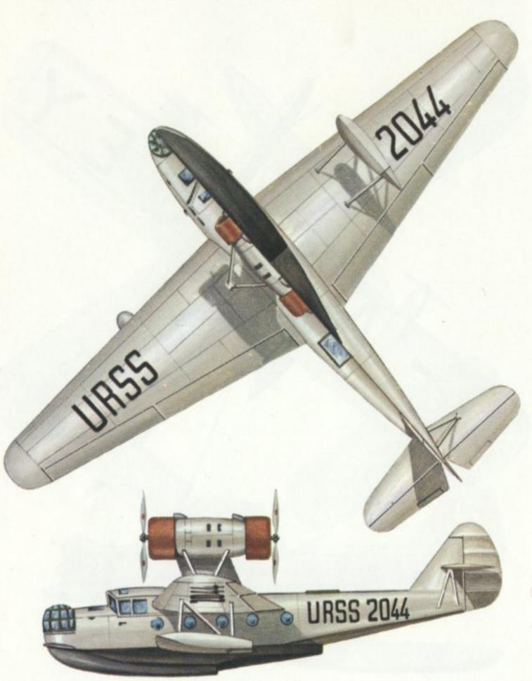
Chetverikov ARK-3-2 (second prototype), Sebastopol, spring 1939. Engines: Two 650 h.p. M-25A nine-cylinder radials. Span: 65 ft. 10½ in. (20·07 m.). Length: 48 ft. 0¾ in. (14·65 m.). Wing area: 641 sq. ft. (59·55 sq. m.). Maximum take-off weight: 12,346 lb. (5,600 kg.). Maximum speed: 199 m.p.h. (320 km/hr.) at 4,920 ft. (1,500 m.). Operational ceiling: approx 19,360 ft. (5,900 m.). Normal range: approx 930 miles (1,500 km.).
