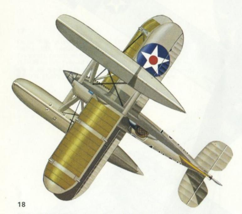
Curtiss CR-3 (A6081), winner of the 1923 Schneider Trophy race at Cowes, U.K. Engine: One 450 h.p. Curtiss D-12 twelve-cylinder Vee-type. Span: 22 ft. 8 in. (6·91 m.). Length: 25 ft. 0\frac{3}{8} in. (7·63 m.). Wing area: 168 sq. ft. (15·61 sq. m.). Take-off weight: 2,746 lb. (1,246 kg.). Maximum speed: 194 m.p.h. (312 km/hr.) at sea level. Operational ceiling: 19,200 ft. (5,852 m.). Range: 522 miles (840 km.).
