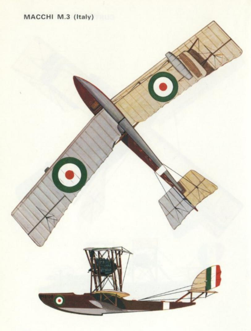
Macchi M.3 of the Regia Marina Italiana, 1918/19. Engine: 160 h.p. Isotta-Fraschini V-4B twelve-cylinder Vee-type. Span: 52 ft. 4 in. (15·95 m.). Length: 33 ft. 7½ in. (10·25 m.). Wing area: 484·4 sq. ft. (45 sq. m.). Take-off weight: 2,976 lb. (1,350 kg.). Maximum speed: 90 m.p.h. (145 km/hr.). Operational ceiling: 19,685 ft. (6,000 m.). Range: 280 miles (450 km.).
