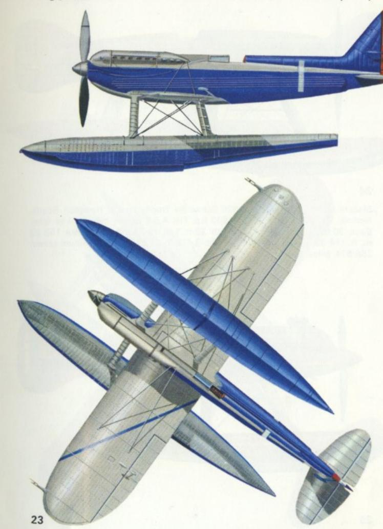
Supermarine S.6B, winning aircraft in the 1931 event for the Schneider Trophy in the U.K. Engine: One 2,350 h.p. Rolls-Royce 'R' twelve-cylinder Vee-type. Span: 30 ft. 0 in. (9·14 m.). Length: 28 ft. 10 in. (8·79 m.). Wing area: 145 sq. ft. (13·47 sq. m.). Take-off weight: 6,086 lb. (2,761 kg.). Maximum speed: 379·05 m.p.h. (610·75 km/hr.) with 2,350 h.p. engine.
