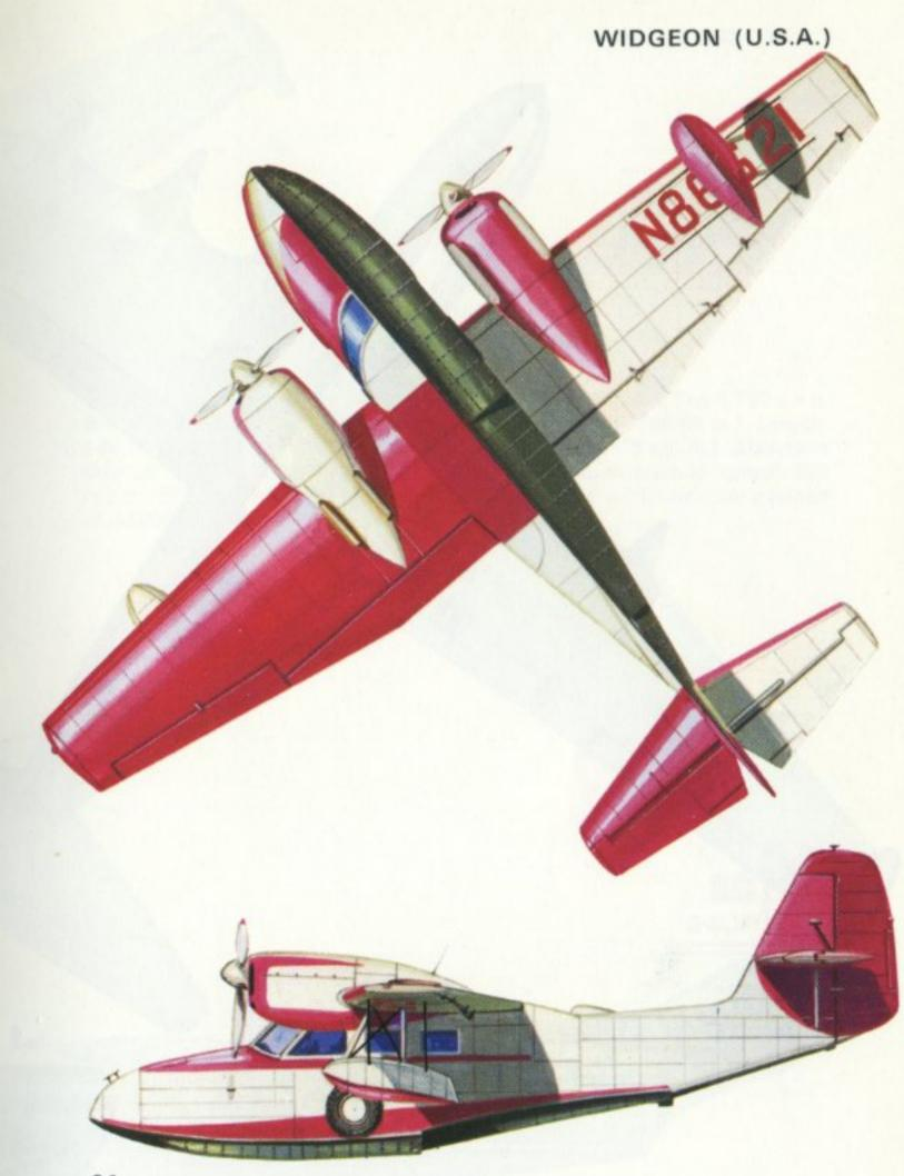
Grumman G-44A Super Widgeon of the US Fish and Wildlife Service, ca 1966. Engines: Two 270 h.p. Lycoming GO-480-B1D 'flat six'. Span: 40 ft. 0 in. (12·19 m.). Length: 31 ft. 1 in. (9·47 m.). Wing area: 245 sq. ft. (22·76 sq. m.). Take-off weight: 5,500 lb. (2,495 kg.). Maximum speed: 185 m.p.h. (298 km/hr.). Operational ceiling: 18,000 ft. (5,486 m.). Range: 1,000 miles (1,610 km.).
