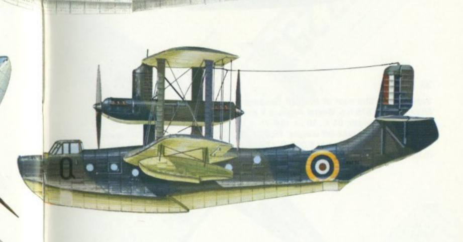
Short S.19 Singapore III of No. 209 Squadron RAF, mid-1940. Engines: Two 730 h.p. Rolls-Royce Kestrel VIII and two 730 h.p. Kestrel IX twelve-cylinder Vee-type. Span: 90 ft. 0 in. (27·43 m.). Length: 64 ft. 2 in. (19·56 m.). Wing area: 1,834 sq. ft. (170·39 sq. m.). Take-off weight: 27,500 lb. (12,474 kg.). Maximum speed: 145 m.p.h. (233 km/hr.) at 2,000 ft. (1,524 m.). Operational ceiling: 15,000 ft. (4,572 m.). Normal range: 1,000 miles (1,609 km.).
