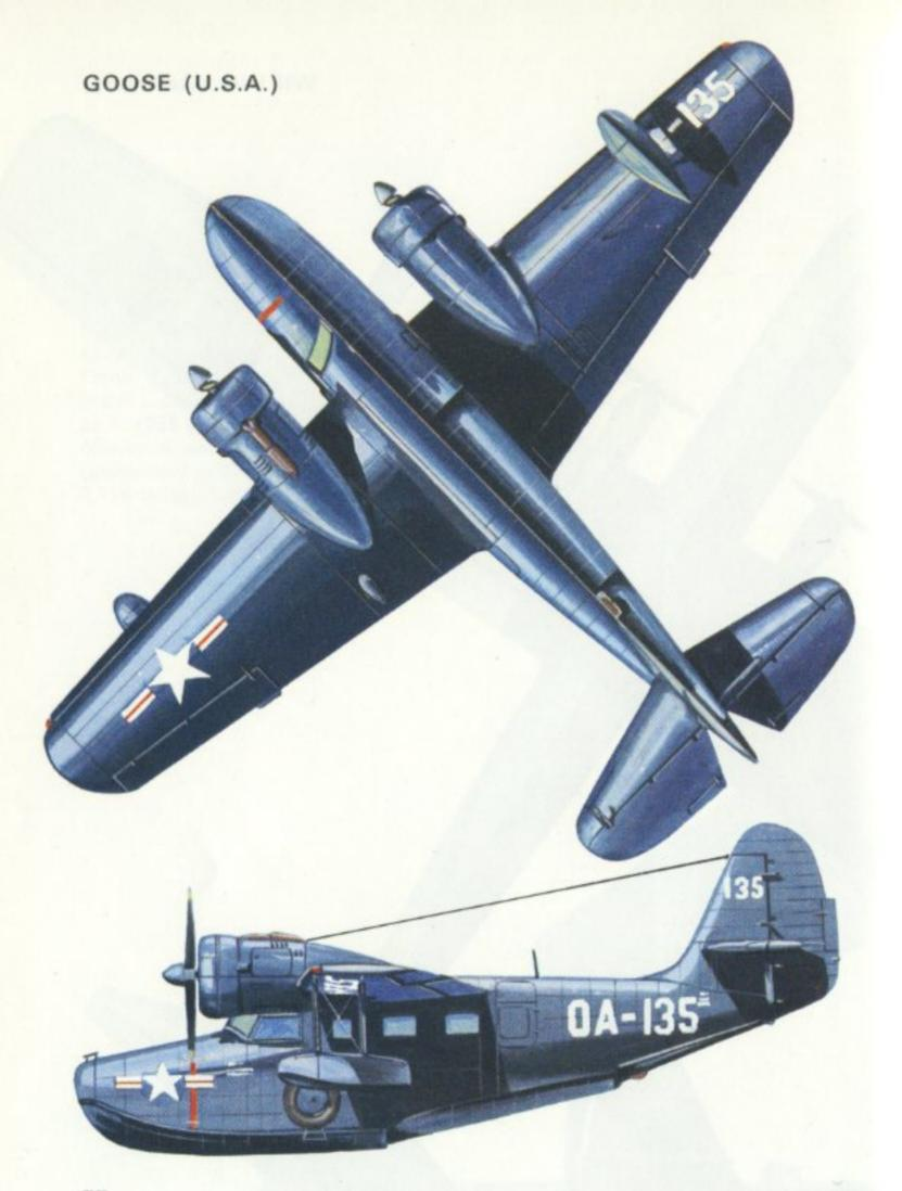
Grumman JRF-5 Goose of the US Navy, ca 1945. Engines: Two 450 h.p. Pratt & Whitney R-985-AN-6 Wasp Junior nine-cylinder radials. Span: 49 ft. 0 in. (14·94 m.). Length: 38 ft. 4 in. (11·68 m.). Wing area: 375 sq. ft. (34·84 sq. m.). Take-off weight: 8,000 lb. (3,629 kg.). Maximum speed: 201 m.p.h. (323 km/hr.) at 5,000 ft. (1,524 m.). Operational ceiling: 21,300 ft. (6,492 m.). Maximum range: 640 miles (1,030 km.).
