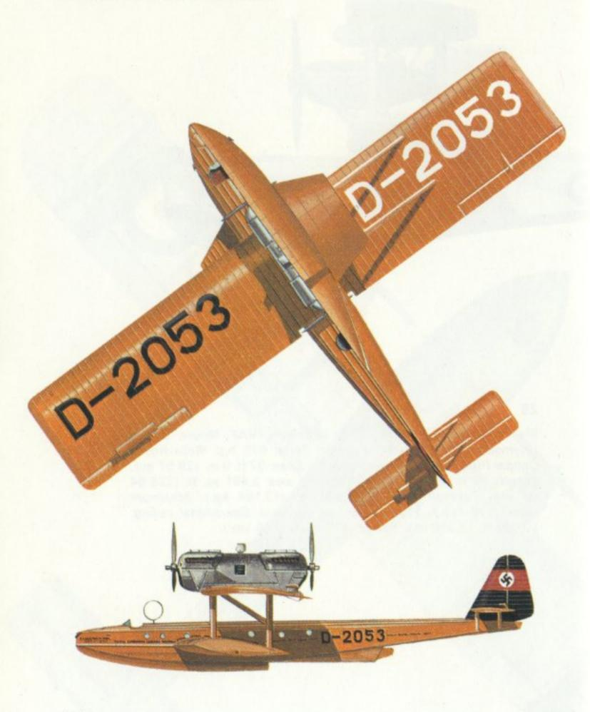
Dornier-built Do J II b Bos *Grönland-Wal* of Deutsche Luft Hansa, ca 1933. (The aircraft flown by von Gronau across the Atlantic in August 1930). *Engines:* Two 600 h.p. BMW VI twelve-cylinder Vee-type. *Span:* 76 ft. 1½ in. (23·20 m.). *Length:* 59 ft. 8½ in. (18·20 m.). *Wing area:* 1,033·3 sq. ft. (96 sq. m.). *Take-off weight:* 17,637 lb. (8,000 kg.). *Maximum speed:* 140 m.p.h. (225 km/hr.). *Operational ceiling:* 9,845 ft. (3,000 m.). *Range:* 1,365 miles (2,200 km.).
