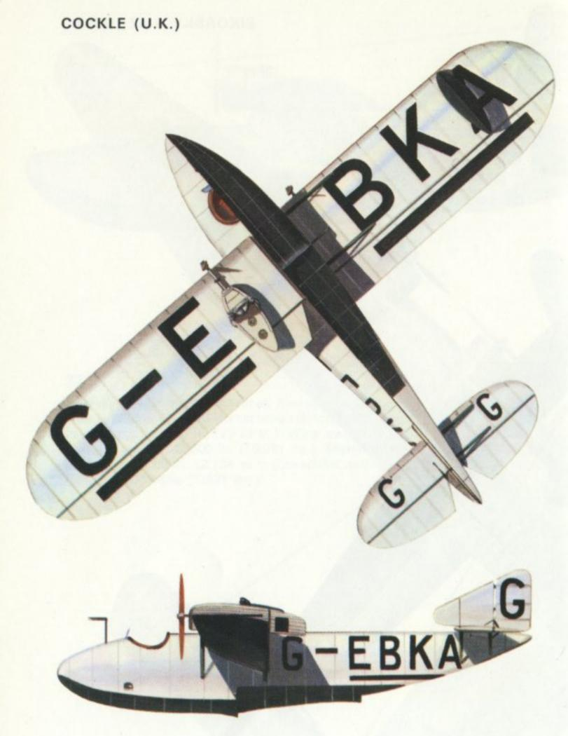
Short S.1 Cockle, late 1924. Engines: Two 697 cc Blackburne Tomtit motor-cycle engines, each developing 16 h.p. Span: 36 ft. 0 in. (10·97 m.). Length: 24 ft. 8 in. (7·52 m.). Wing area: 210 sq. ft. (19·51 sq. m.). Take-off weight: 1,062 lb. (482 kg.). Maximum speed: 68 m.p.h. (109 km/hr.).
