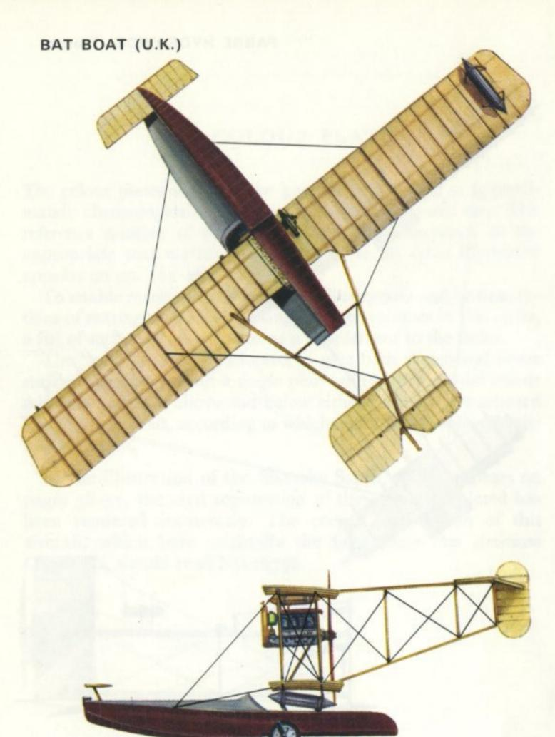
Sopwith Bat Boat, early summer 1913. Engine: One 90 h.p. Austro-Daimler four-cylinder in-line. Span: 41 ft. 0 in. (12·50 m.). Length: 30 ft. 4 in. (9·24 m.). Wing area: 428 sq. ft. (39·76 sq. m.). Take-off weight: 1,700 lb. (771 kg.). Speed: 65 m.p.h. (105 km/hr.).
