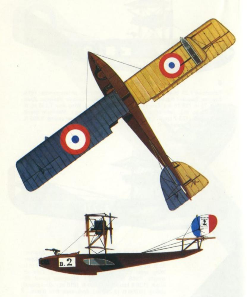
FBA Type H of the French Navy, ca 1919/20. Engine: One 170 h.p. Hispano-Suiza six-cylinder in-line. Span: 47 ft. 6¾ in. (14·50 m.). Length: 33 ft. 1¾ in. (10·10 m.). Wing area: 452·1 sq. ft. (42 sq. m.). Take-off weight: 3,219 lb. (1,460 kg.). Maximum speed: 90 m.p.h. (145 km/hr.). Range: 185 miles (300 km.).
