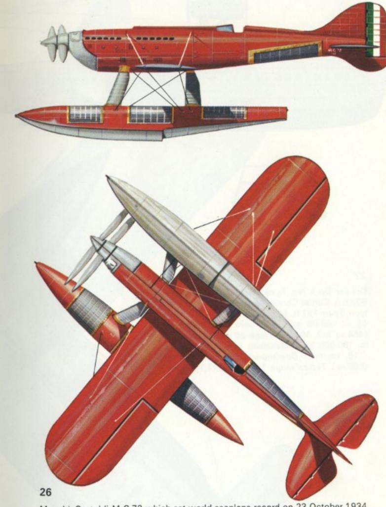
Macchi-Castoldi M.C.72 which set world seaplane record on 23 October 1934. Engine: One 2,800 h.p. Fiat A.S.6 twenty-four-cylinder Vee-type (two A.S.5 engines coupled in tandem). Span: 31 ft. 1½ in. (9·48 m.). Length: 27 ft. 3½ in. (8·32 m.). Wing area: 161·46 sq. ft. (15 sq. m.). Take-off weight: 6,409 lb. (2,907 kg.). Maximum speed: 440·681 m.p.h. (709·209 km/hr.).
