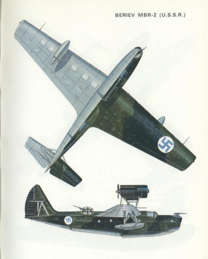
Beriev MBR-2, captured aircraft in Finnish Air Force markings (TLeLv 12), August 1941. Engine: One 750 h.p. Mikulin AM-34NB twelve-cylinder Vee-type. Span: 62 ft. 4 in. (19 m.). Length: 44 ft. 3½ in. (13·50 m.). Wing area: 592 sq. ft. (55 sq. m.). Maximum take-off weight: 9,359 lb. (4,245 kg.). Maximum speed: 171 m.p.h. (275 km/hr.) at 6,560 ft. (2,000 m.). Operational ceiling: 25,920 ft. (7,900 m.). Typical range: 405 miles (650 km.).
