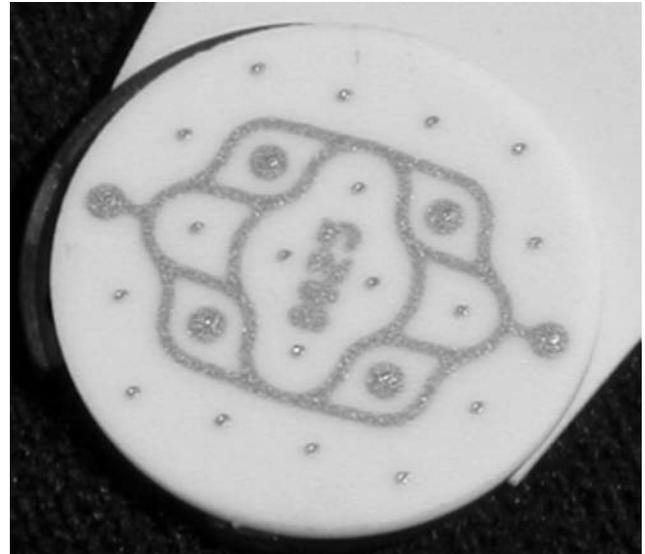
**Figure 11.** Close-up view of tissue glucose and oxygen sensor array (77). Sensor array with small ( $125\text{ }\mu\text{m}$  diameter) independent platinum working electrodes, large ( $875\text{ }\mu\text{m}$  diameter) common platinum counterelectrodes, and a curved common Ag/AgCl reference electrode. The membrane is not present. (Copyright 2003, American Physiological Society.)
