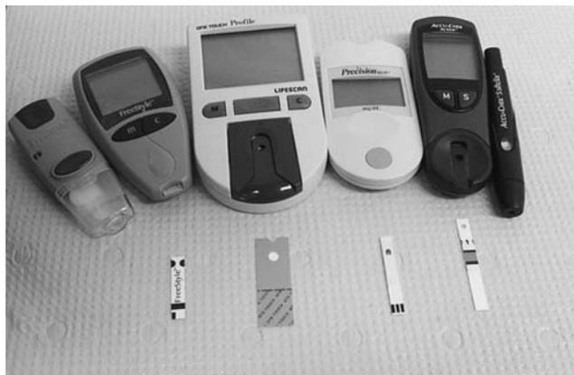
**Figure 3.** A small collection of home glucose monitoring equipment developed over the past decade. At either end (above) are devices used to puncture the skin for sample collection. Examples of commercial glucose meter (above, center) are also shown. Strips (below) contain immobilized glucose oxidase and are discarded after a single measurement.
