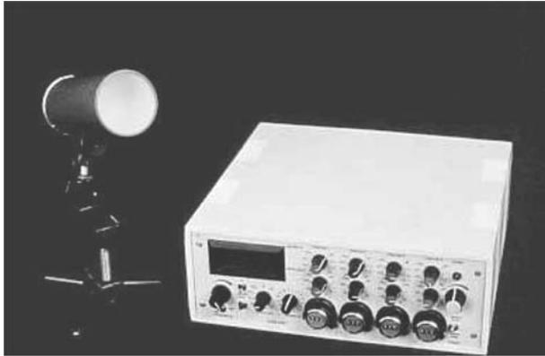
**Figure 3.** A “mini-Ganzfeld” based on light emitting diode technology. The device shown has four independent color channels, blue, green, orange and red, each of which can be used as stimulus or background alone or in combination. (Courtesy of Chris Hogg, CH electronics, Bromley, Kent, UK; [www.ch-electronics.net](http://www.ch-electronics.net).)
