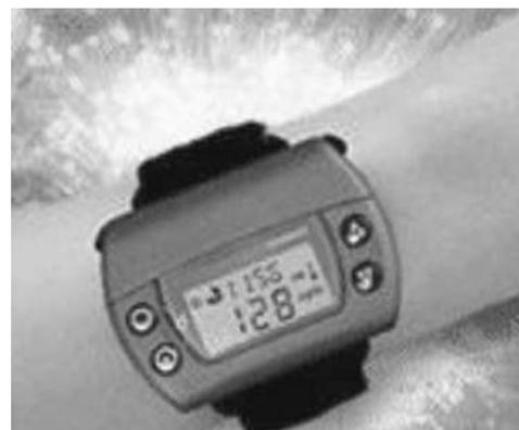
**Figure 13.** GlucoWatch device (1) and principle of iontophoresis (2). This device provides non-invasive monitoring of glucose and uses reverse iontophoresis to extract glucose from the skin to monitor glucose. A low electric current is applied, which draws interstitial fluid through the skin. The glucose in this fluid is collected in a gel. A chemical process occurs, which generates an electrical signal that is converted into a glucose measurement.
