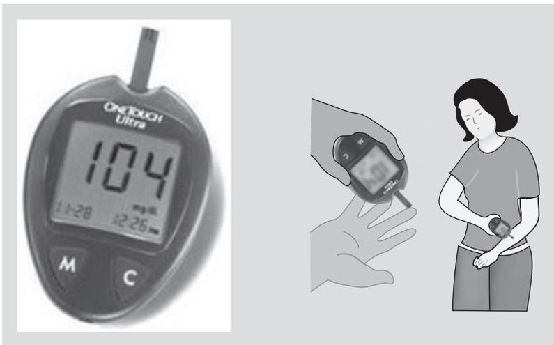
**Figure 12.** Glucose meter. This is used for self-monitoring blood glucose. The blood is taken from the fingertip and analyzed using a test strip.
