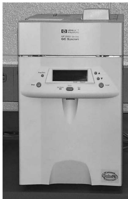
**Figure 4.** An HP/Agilent laboratory-grade gas chromatograph.
