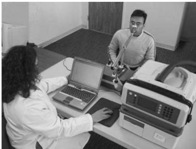
**Figure 5.** Mensanna portable GC for measuring breath VOCs.
