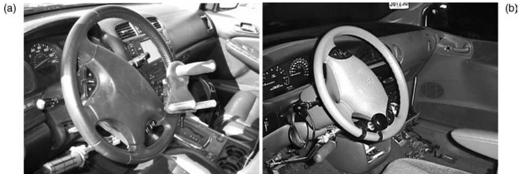
**Figure 7.** Steering knobs.
