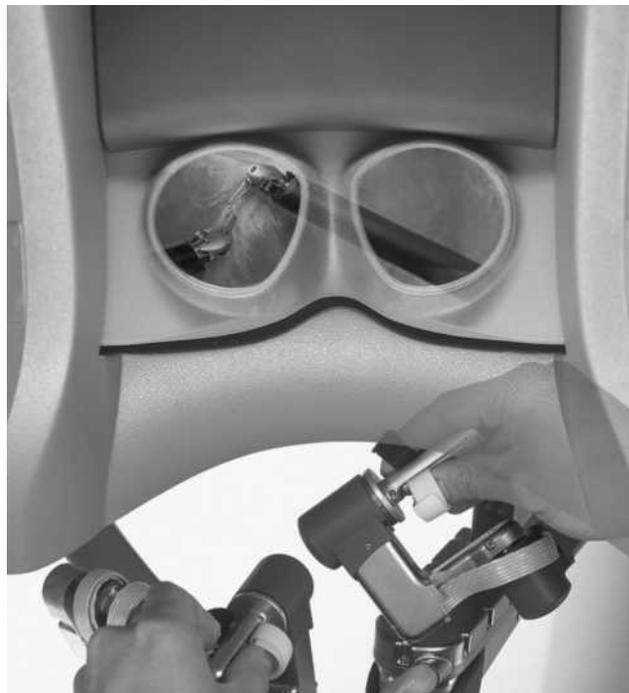
**Figure 4.** Intuitive Surgical stereo display and joysticks. (Copyright ©2005 Intuitive Surgical, Inc.)
