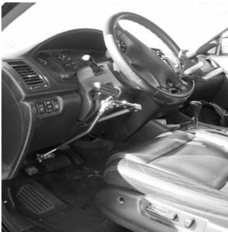
**Figure 8.** Common hand controls.
