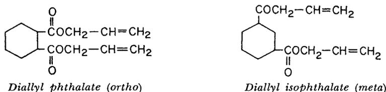
Figure A.9 General chemical structures for diallyl phthalate and diallyl isophthalate.
