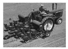
Fig. 5. Planting cotton with a four-row tractor-propelled planter. (John Deere Co.)
