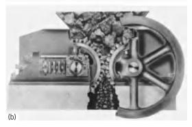
Fig. 4. Types of roll crusher. (a) Single-roll. (b) Double-roll. (Link Belt Co.)
