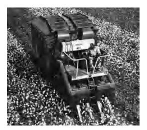
Fig. 6. Two-row, self-propelled cotton picker in operation. (International Harvester Co.)
