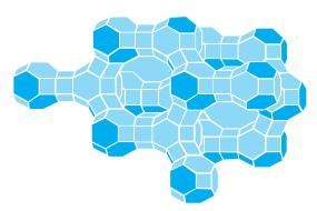
Fig. 3. Model of zeolite type Y.
