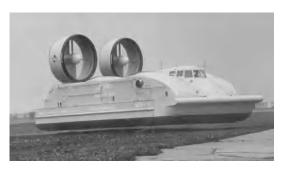
Fig. 2. Two ducted fans provide propulsion for Bell-Navy Hydroskimmer. (Bell Aerosystems Co.)
