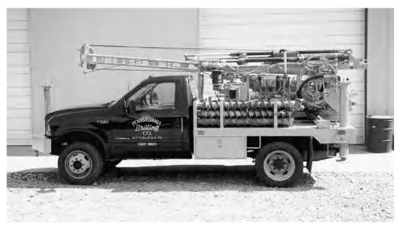
Fig. 1. Auger-core drill. (Pennsylvania Drilling Co.)
