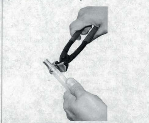
Figure 6-49 Uponor SSC Fitting Removal
