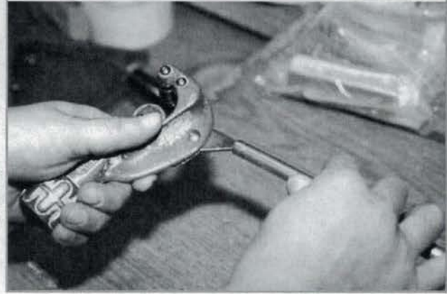
Figure 6-66 Tube Cutter with Deburring Tool
