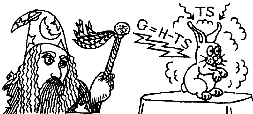
Figure 5.1. To create a rabbit out of nothing and place it on the table, the magician need not summon up the entire enthalpy, H = U + PV . Some energy, equal to TS , can flow in spontaneously as heat; the magician must provide only the difference, G = H - TS , as work.
