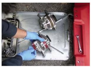
**Step 5:** Compare the old and new alternators to make sure everything is the same. Transfer any connectors or bolts from the old to the new.
