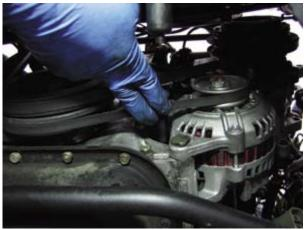
**Step 7:** Check belt tension. A little under an inch of deflection is ideal. Too much tension will quickly destroy bearings. Better a slightly loose belt than one too tight.
