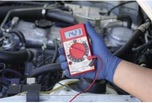
**Step 9:** Start the vehicle and check alternator output with a multimeter.
