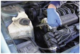
**Step 8:** On this vehicle, the alternator and the engine-driven accessories rely on one serpentine belt. A spring-loaded tensioner holds the belt in place. Slack allows the belt and the alternator to be removed.
