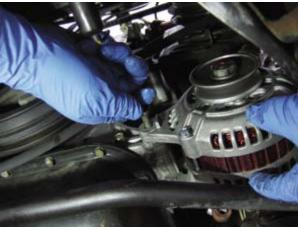
**Step 6:** Reverse the removal procedure and install the new alternator.
