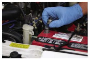
**Step 1:** Disconnect the battery negative. This is an especially important first step, as all the electricity for the entire vehicle goes through the alternator. A wrench or a screwdriver across connectors can quickly fry voltage regulators, expensive engine computers, and cause injury.
