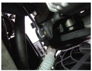
**Step 2:** On a v-belt vehicle there are usually two bolts holding an alternator to its mounts. One bolt or assembly maintains tension on the belts, and the other holds the alternator in place. First loosen and remove the tension bolt or assembly.
