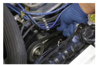
Step 10: Re-check belt tension after about 500 miles. Adjust tension if required.
